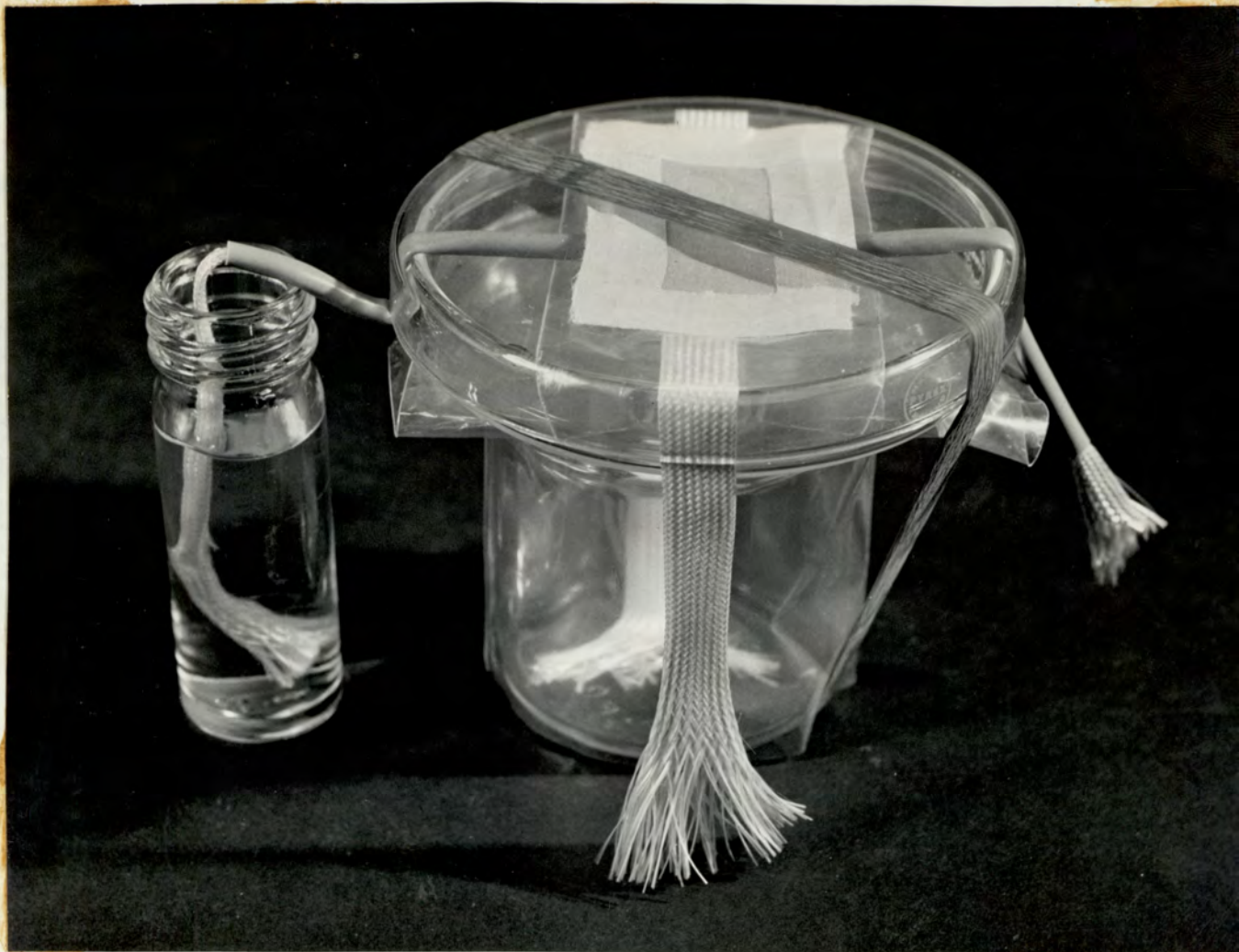
Plate 13. The perfusion device for increasing the oxygen level around veneers. The side bottle contains hydrogen peroxide which perfuses through the extra sleeving.
