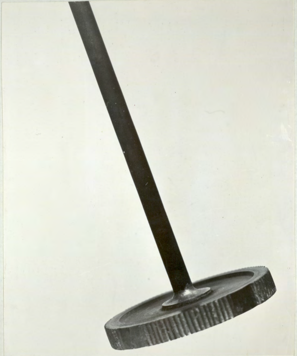
Plate 4. The grinding wheel with cutting grooves along the edge.
