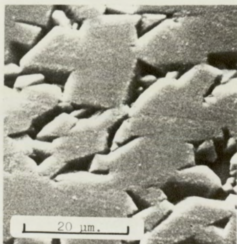
Fig. 2.16. Showing surface of the oxide after polishing with 1 micron diamond paste.
