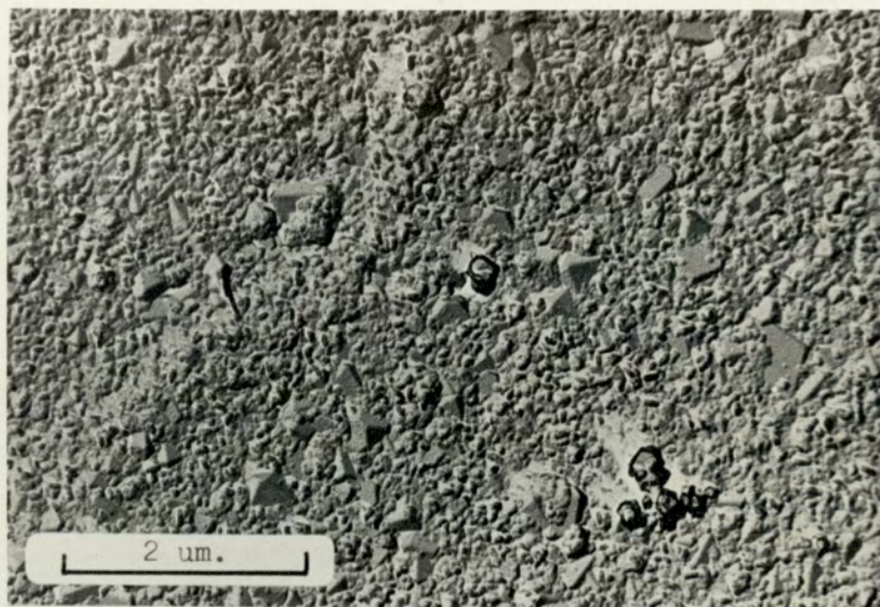
Fig. 5.5. Transmission electron micrograph of a direct carbon replica of steel oxidised in 0.1\text{M FeCl}_2 + 0.001\text{M NiCl}_2 ( 316^\circ\text{C} , 12 minutes).
