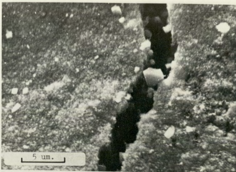
Fig. 6.9a. Scanning electron micrograph of the oxide formed on iron electrodeposited from ammonium ferrous sulphate solution showing defects in the oxide.
