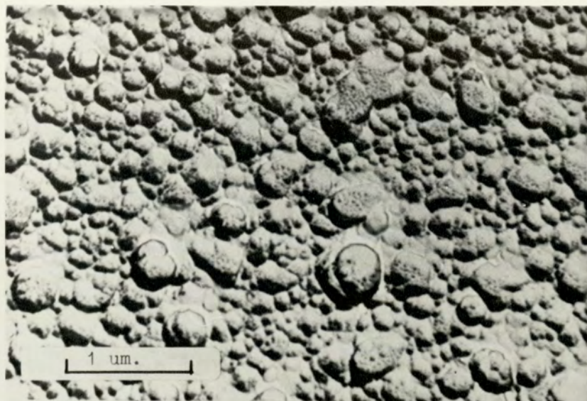
Fig. 3.11. As Fig. 3.10. but oxidised for 40 minutes, showing initial magnetite crystallites.
