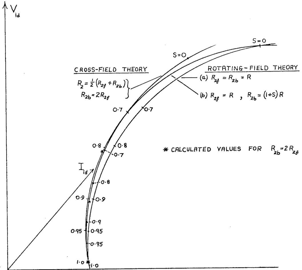
Fig. 5.9 Stator current loci
