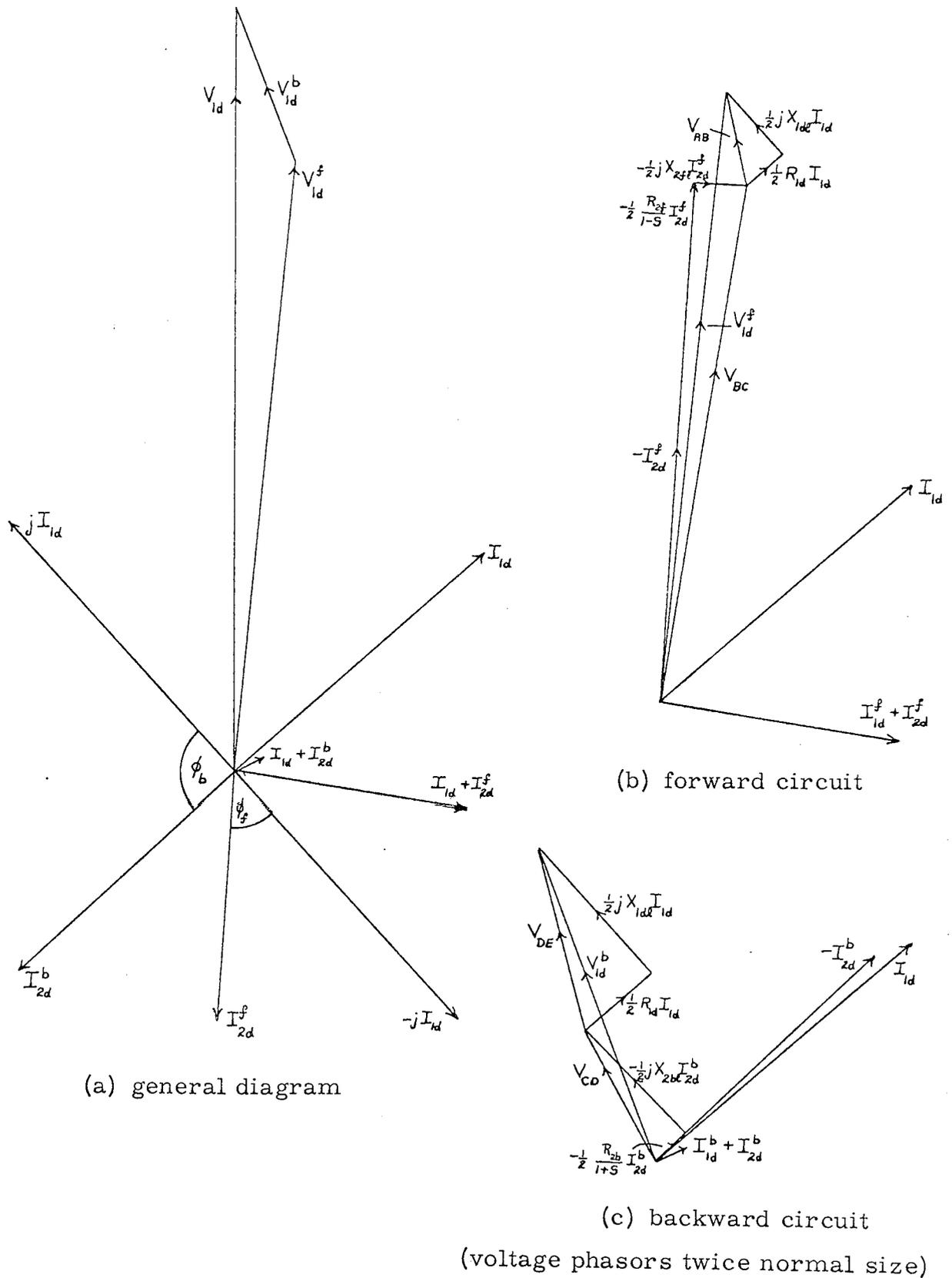
Fig. 3.6 Phasor diagrams based on the equivalent circuit
