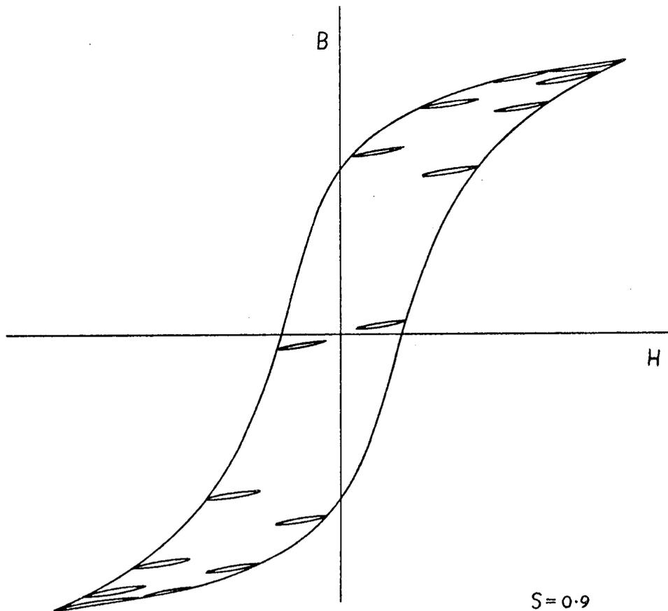
The hysteresis loop for a point on the rotor showing the presence of recoil loops.
