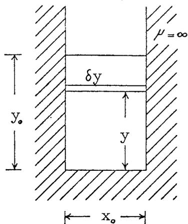
The diagram represents a rectangular conductor embedded in a theoretical slot in iron of infinite permeability.
