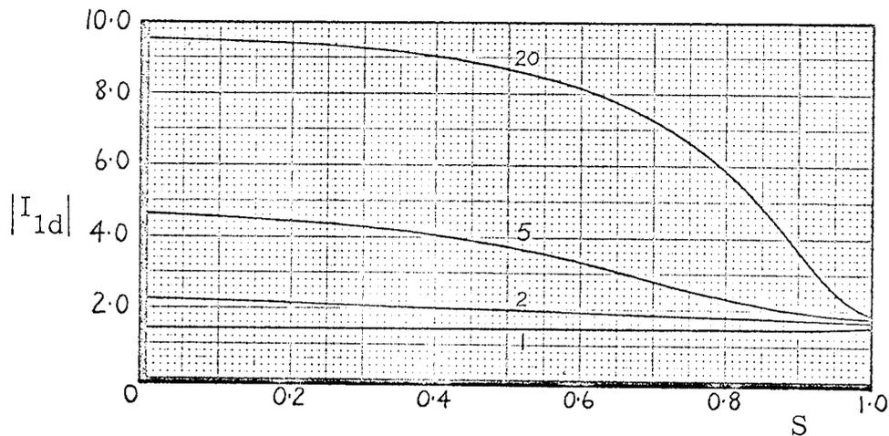
Fig. 3.3 Stator current/speed characteristic for 4 values of the ratio  $X_2/R_2$ .
