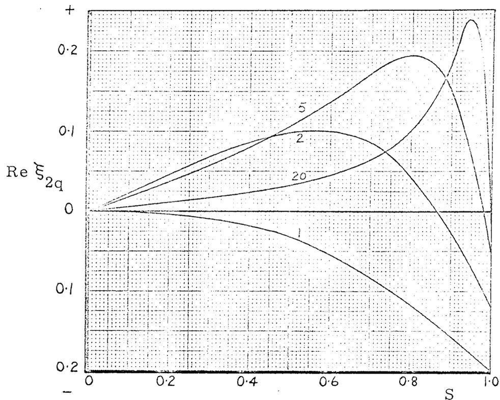
Fig. 3.2 Graph of the function  $\text{Re } \xi_{2q}$  to a base of speed for 4 values of the ratio  $X_2/R_2$ .
