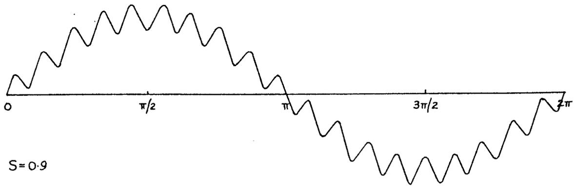
Graph showing the variation of the resultant m.m.f. at a point on the rotor, as the resultant m.m.f. vector moves through  $2\pi$ .
