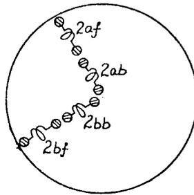
A schematic layout of the windings of the modified rotor is shown in the diagram above. Further subscripts  $f, b$  are added to the parameter symbols to distinguish between the two layers;  $f$  is associated with the low frequency component of the rotor current, while  $b$  is associated with the high frequency component.
