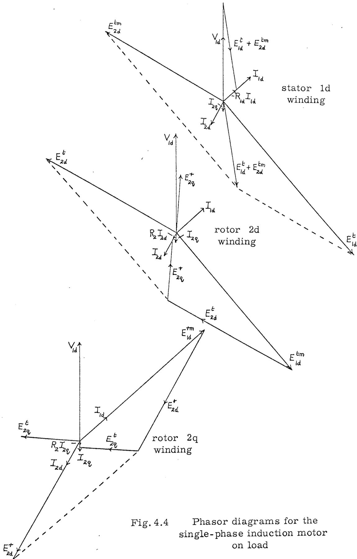
Fig. 4.4 Phasor diagrams for the single-phase induction motor on load
