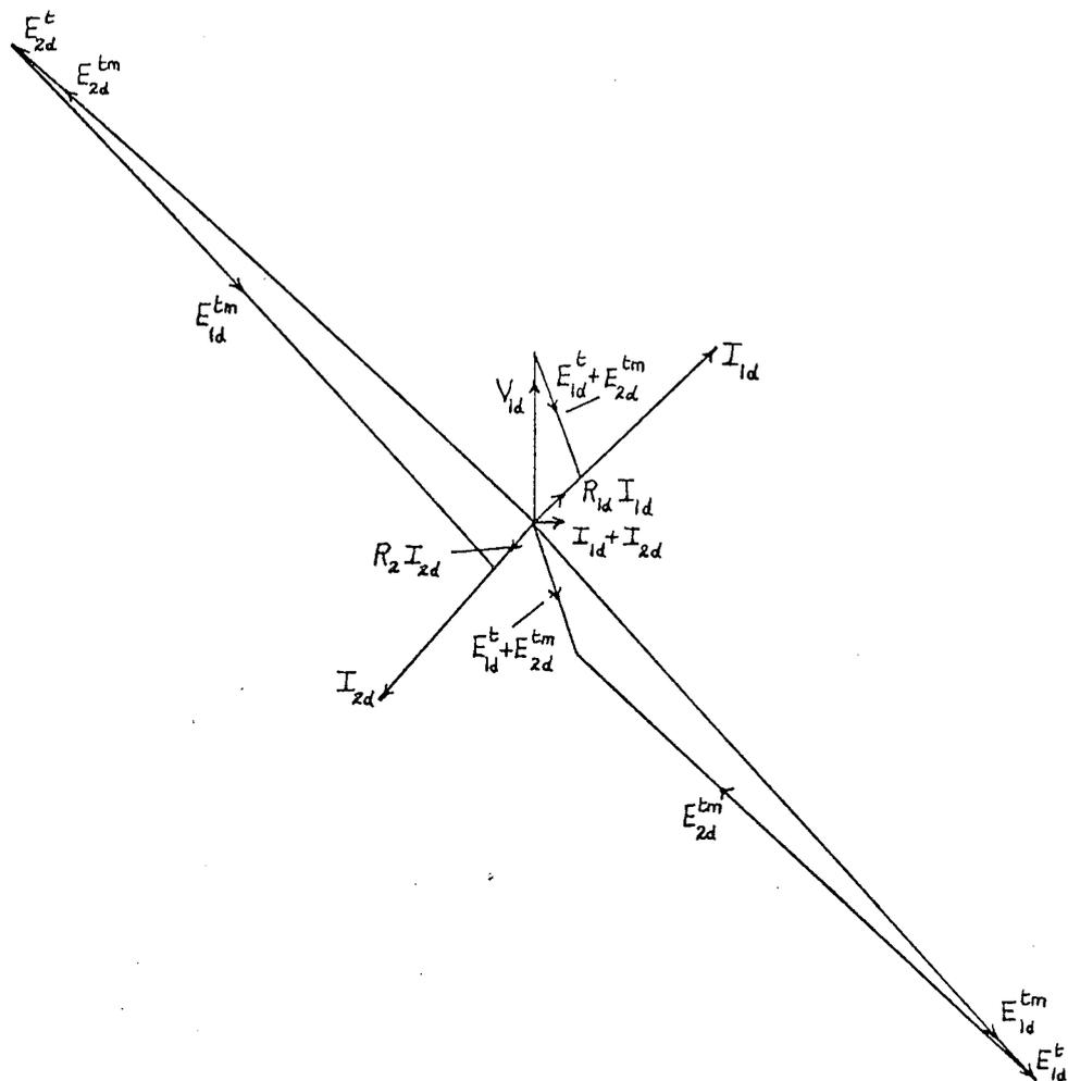
Fig. 4.3 The phasor diagram at standstill for the single-phase induction motor
