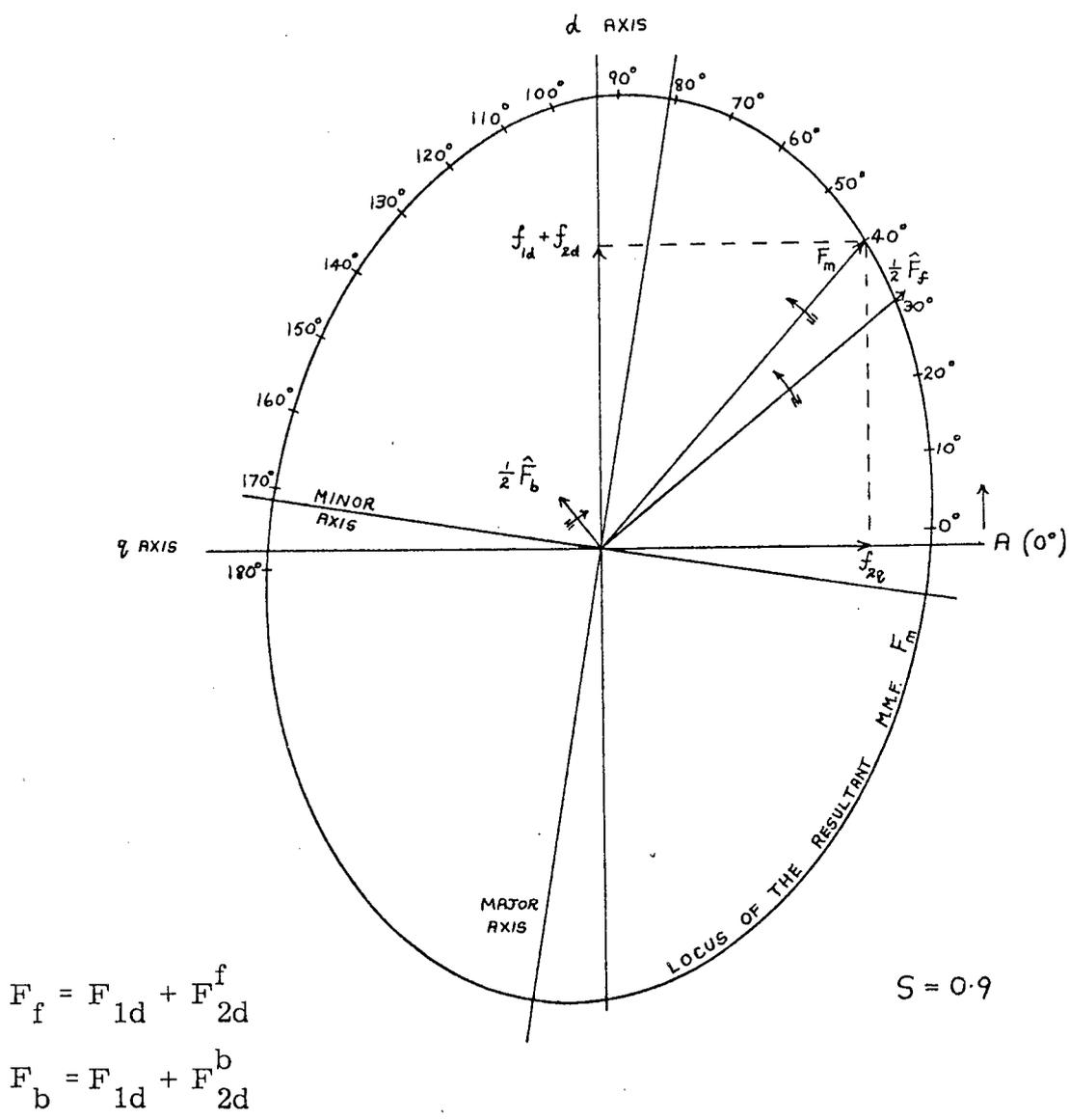
Fig. 5.1 The locus of the resultant m.m.f. vector viewed from the stator.
