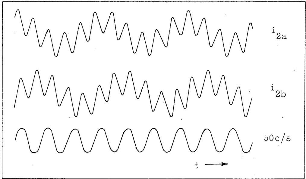
Fig. 2.2 The rotor current waveforms ( $S \approx 0.69$ )
