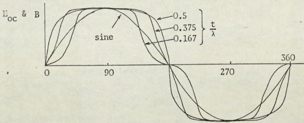
Fig 6: Waveforms of alternating flux,  $\frac{S}{g} = 20$ , and open circuit e.m.f.
