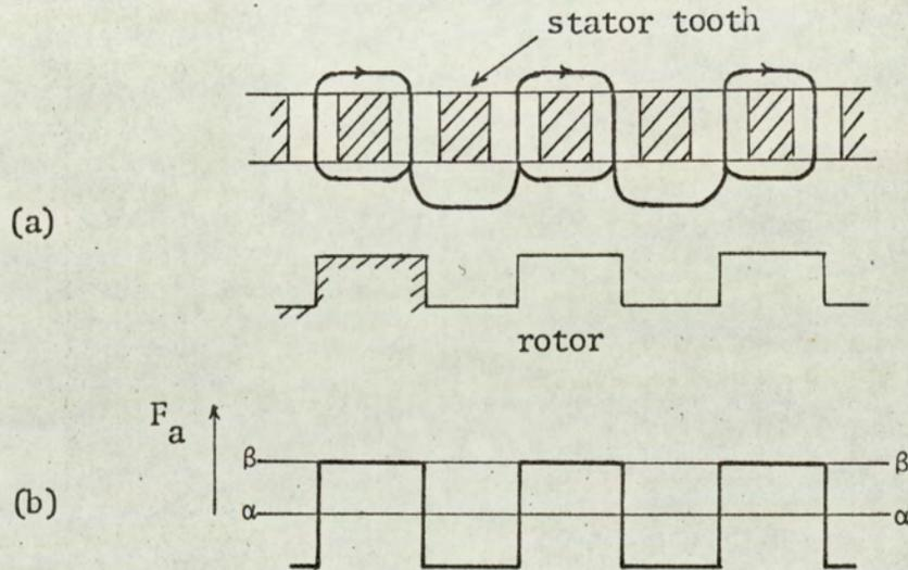
Fig 9: a) Armature winding
