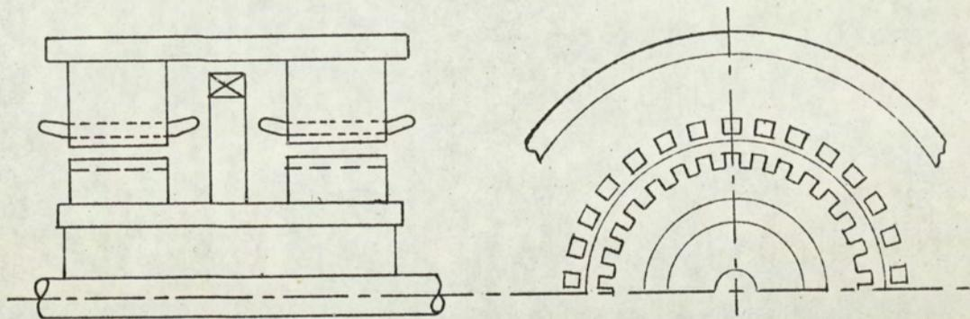
Fig 3: Homopolar inductor-alternator
