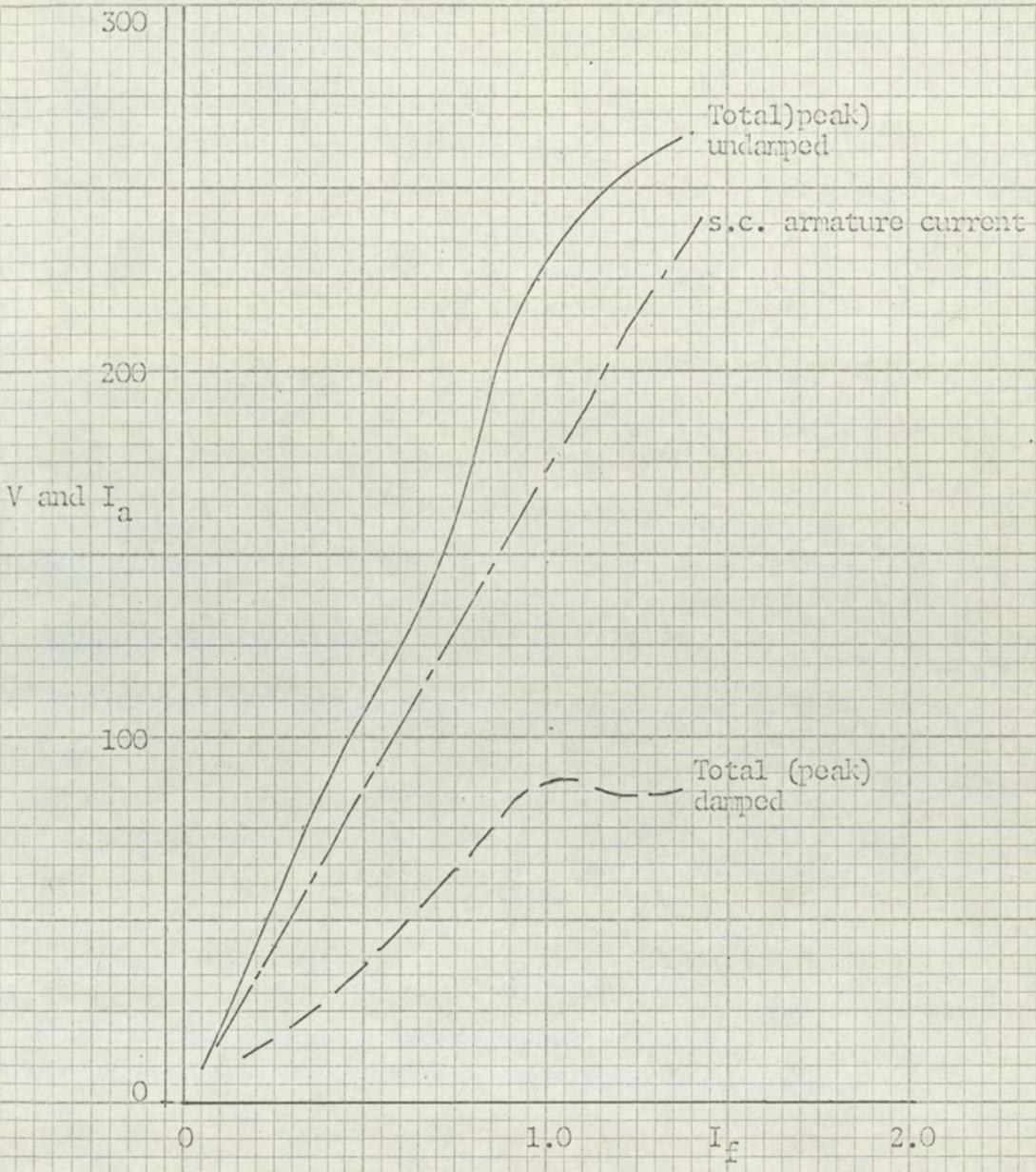
Fig 40(b): Peak voltage induced in a single field coil for short circuit conditions, damped and undamped
