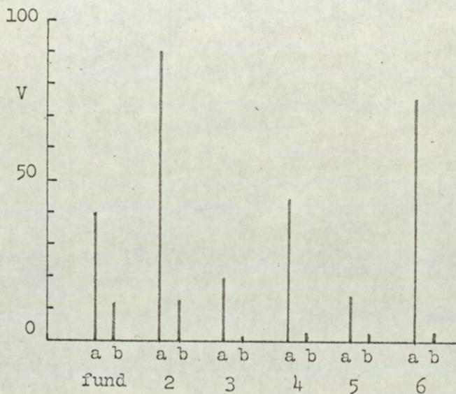
Fig 28: Harmonic voltage modulations present in a single field coil on rated open circuit ( $V_{rms}$ )
