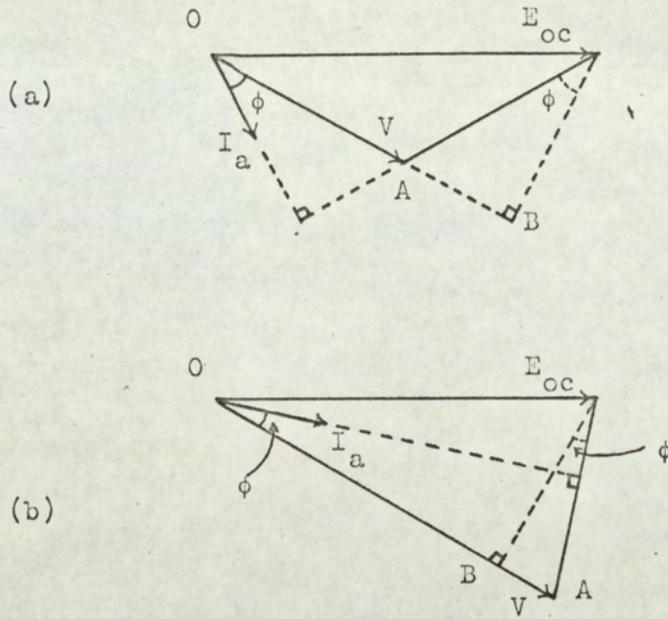
Fig 55: (a) lagging p.f. (b) leading p.f.
