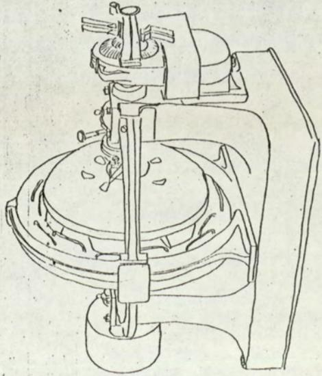
FIG. 3 LARME'S 10,000 KVA ALTERNATOR
