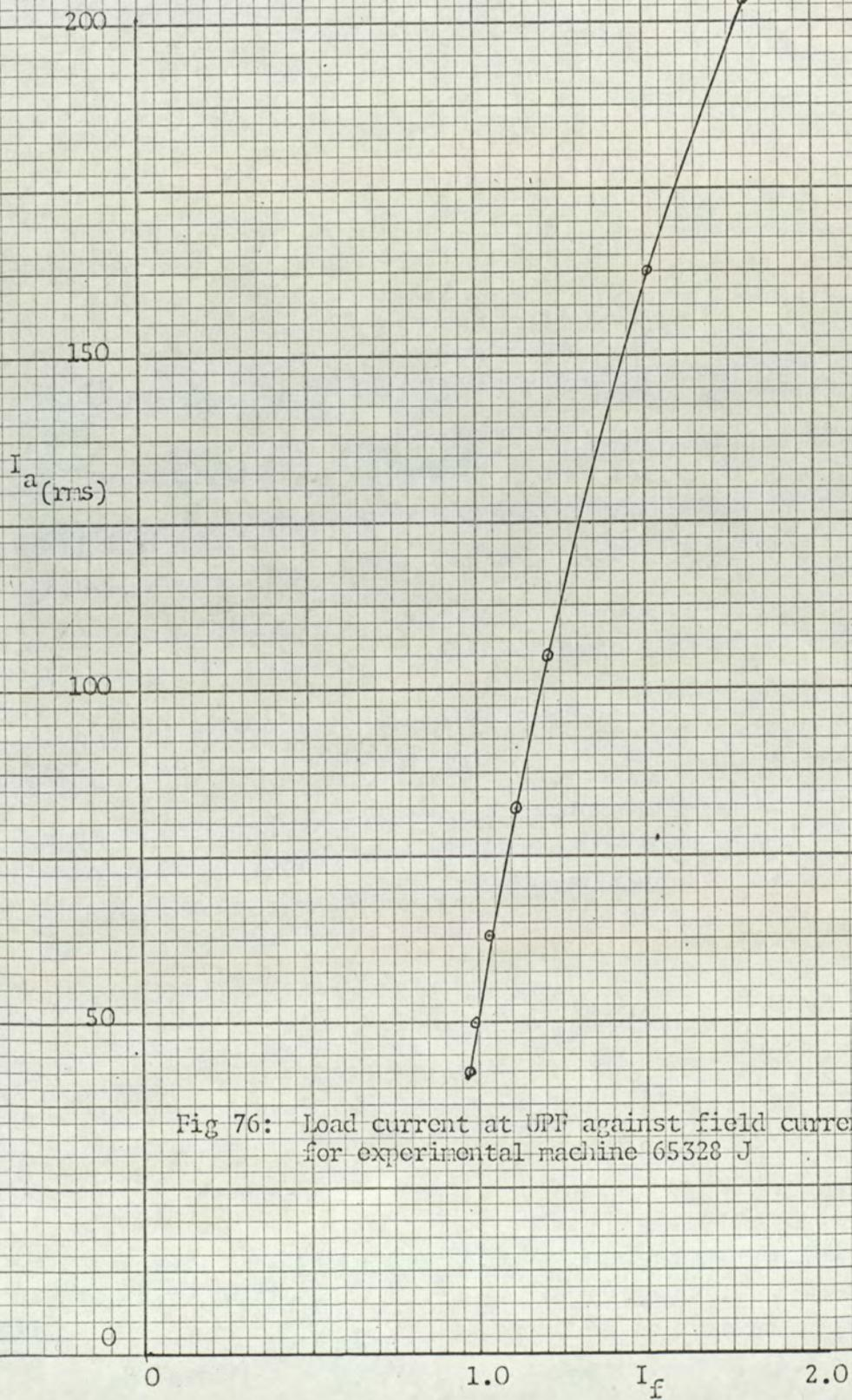
Fig 76: Load current at UPF against field current for experimental machine 65328 J
