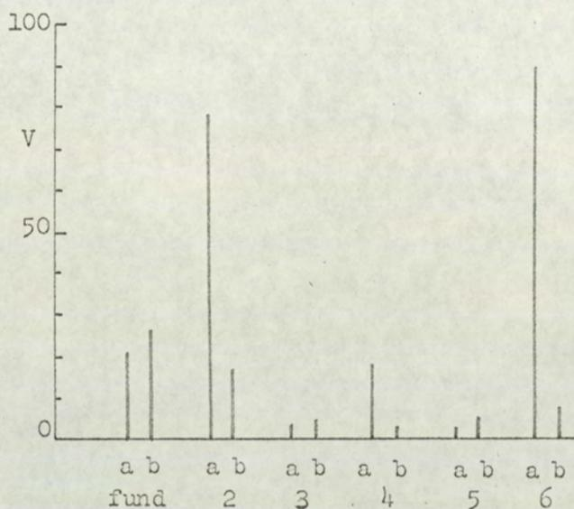
Fig 39: Harmonic voltage modulations present in a single field coil on rated short-circuit ( $V_{rms}$ )
