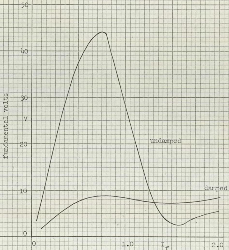
Fig 38: Fundamental voltage induced in a single field coil against field current
