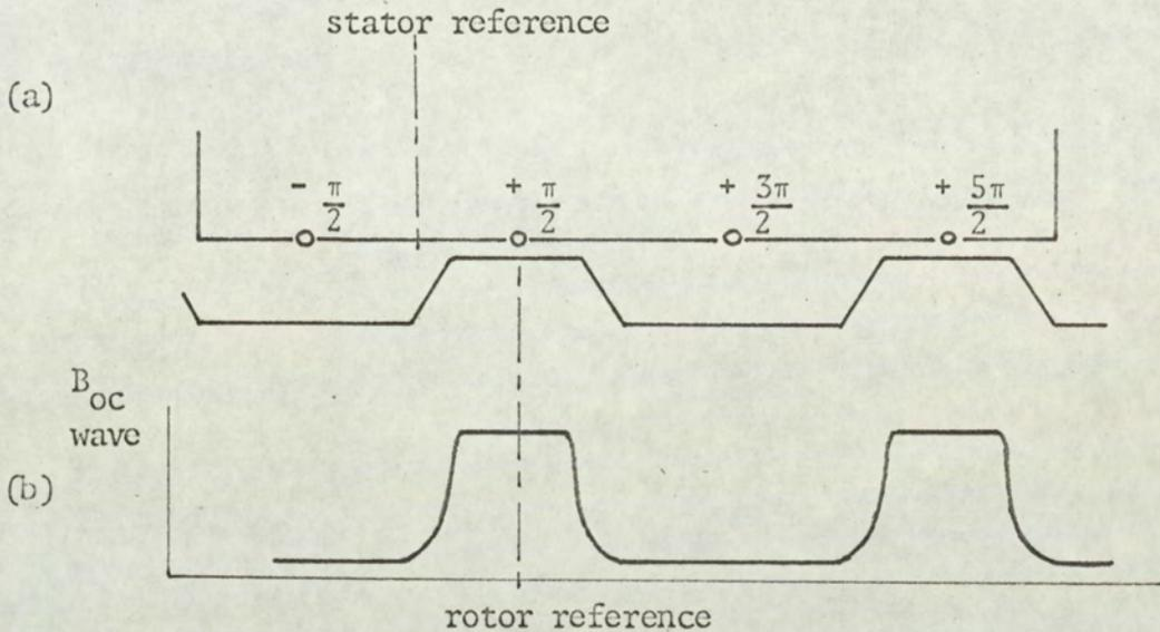
Fig 32: Ideal stator and rotor geometry with open-circuit flux-density wave.
