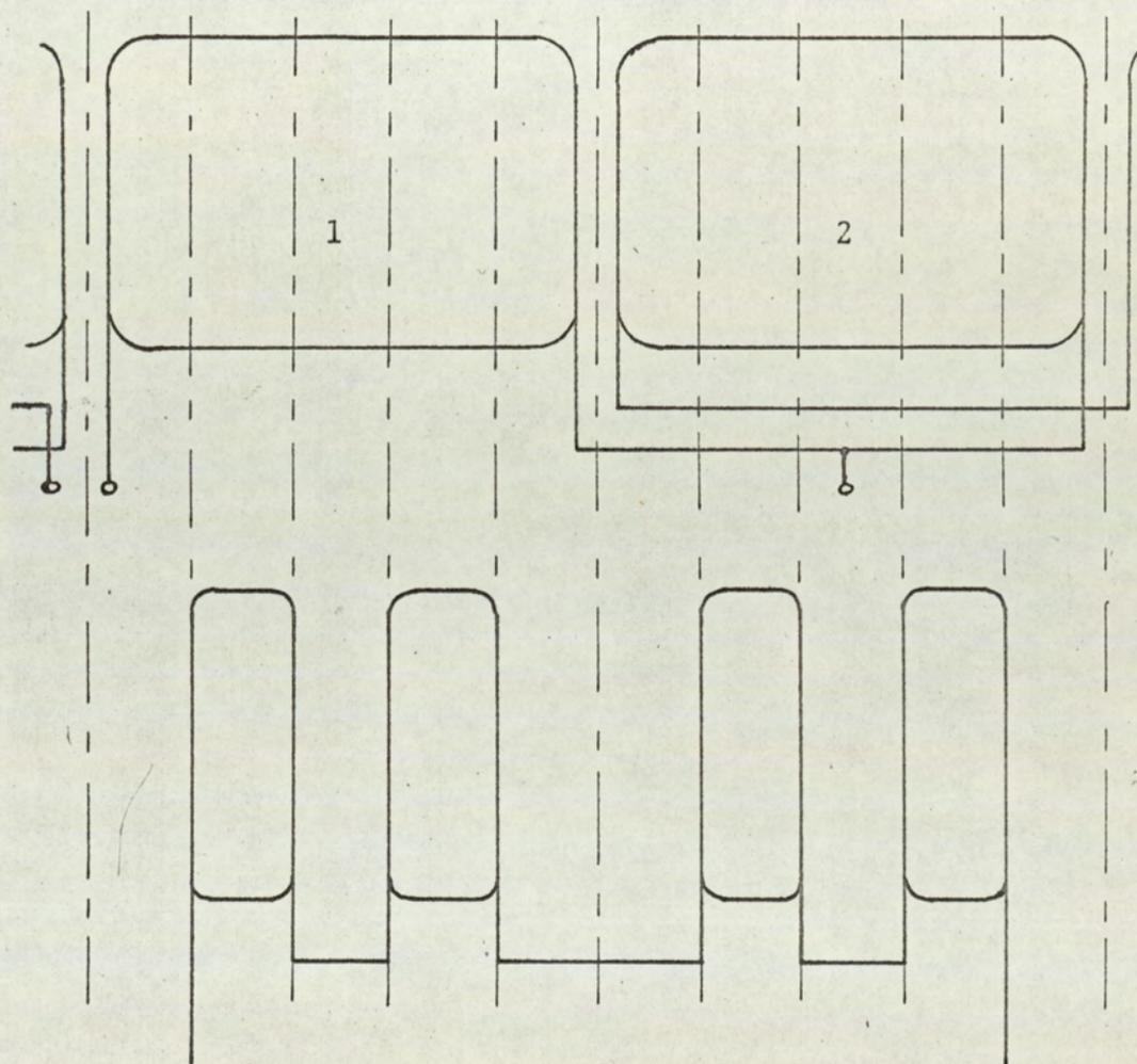
Fig. 22: Winding diagram for field poles 1 and 2
