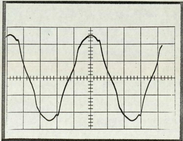
Fig 69: Output waveforms  $I_f = 2.0A$ (m)  $V_{oc} = 215.5$
