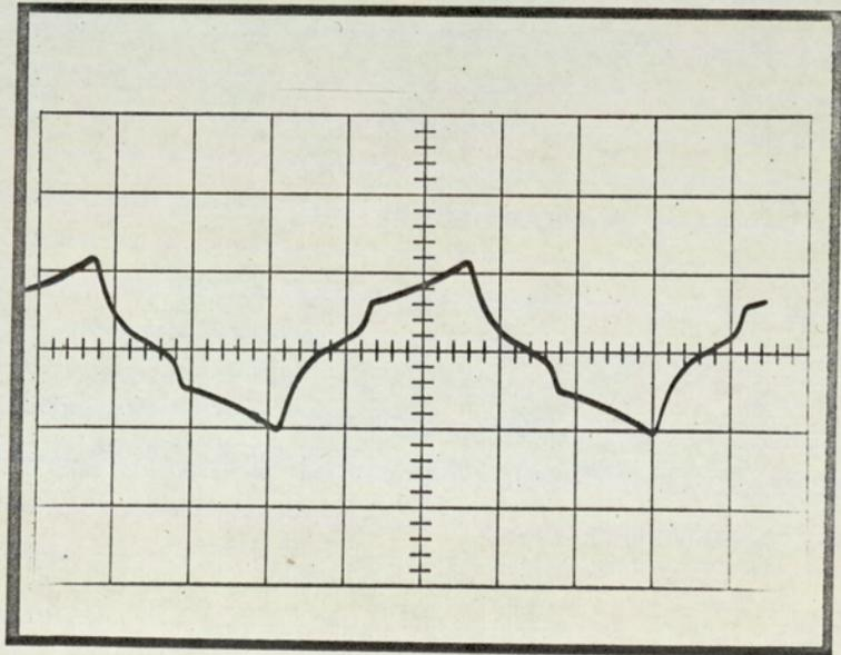
Fig 69: Output waveforms  $I_f = 0.6A$ (e)  $V_{oc} = 110$
