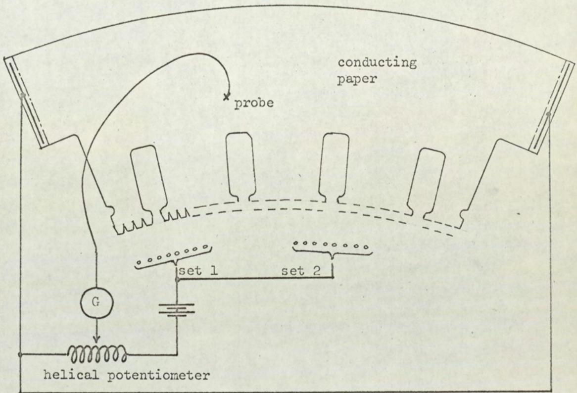
Fig 24: Full d.c. pole pitch conducting paper analogue and circuit for details of tab connections, see Fig 25.
