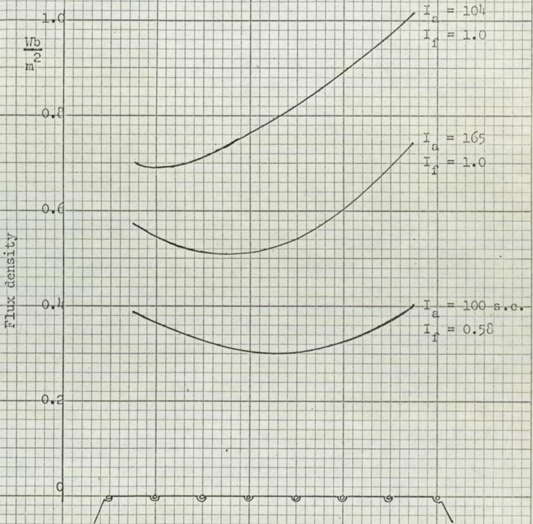
Fig 47: Measured on-load flux density distribution across rotor tooth surface
