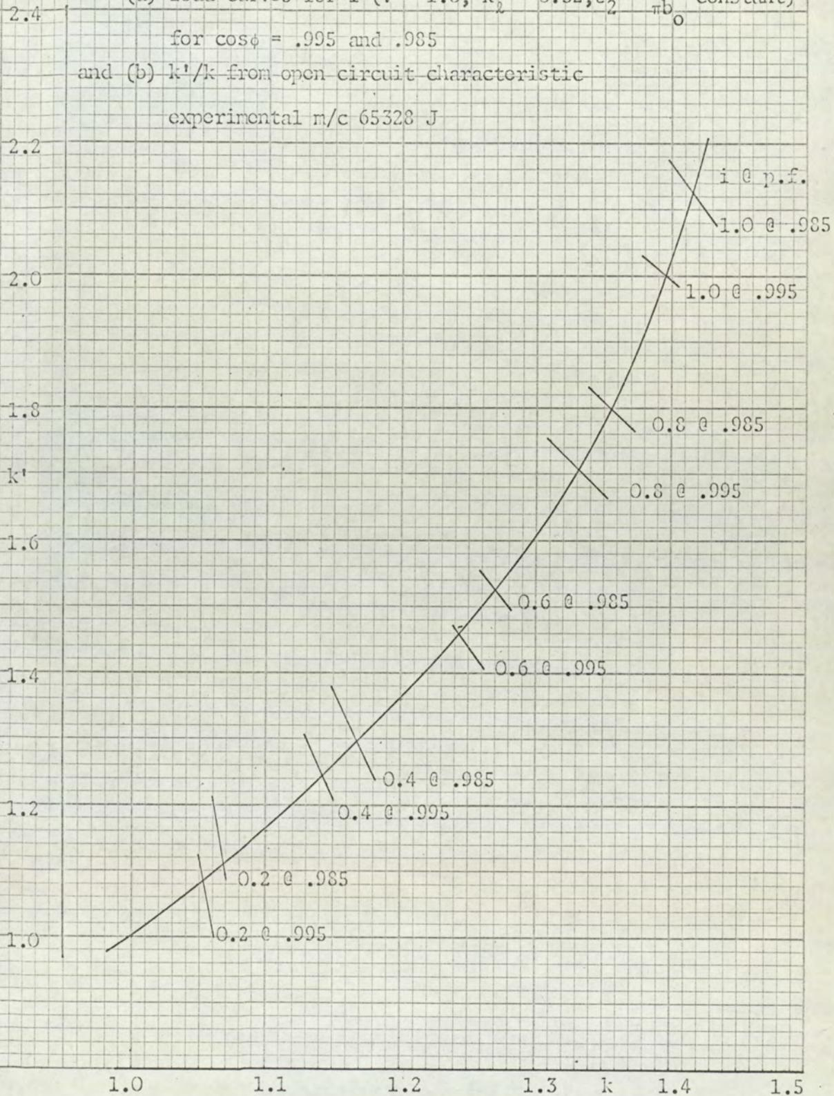
Fig 63: Field current against p.u. load current
