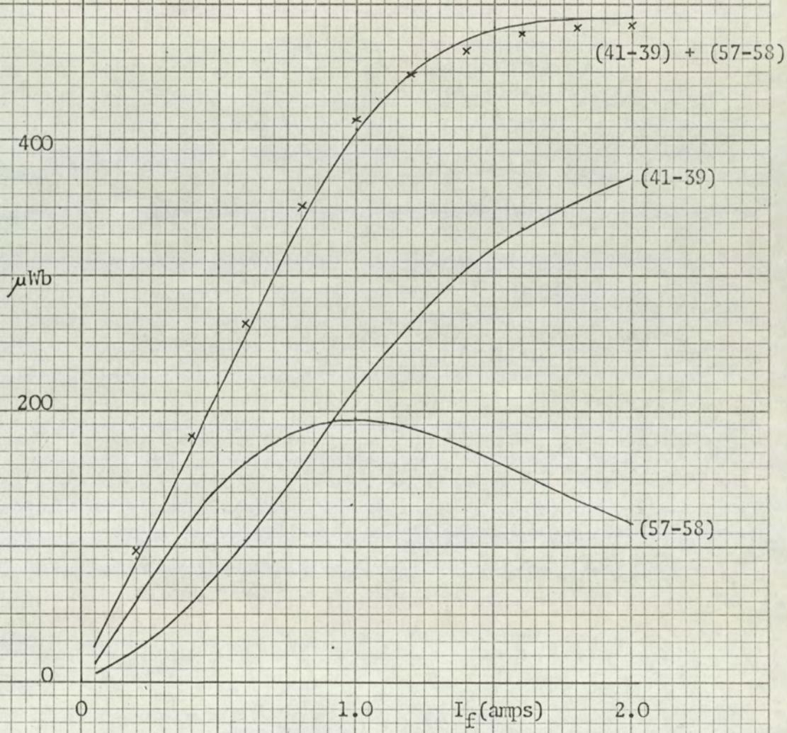
Fig 37: Fundamental fluxes, open-circuit, undamped.
