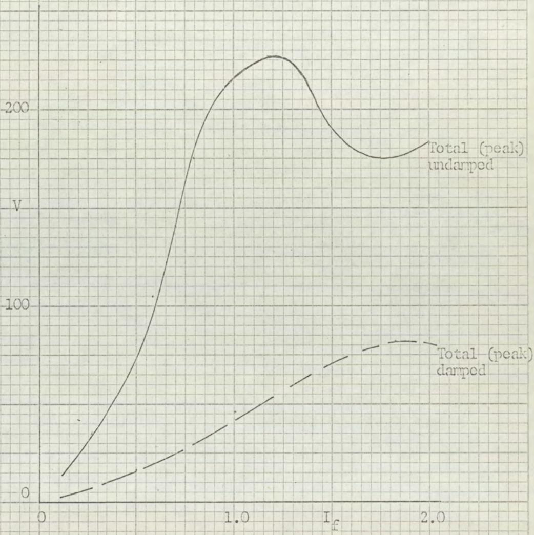
Fig 40(a): Peak voltage induced in a single field coil on open circuit, damped and undamped
