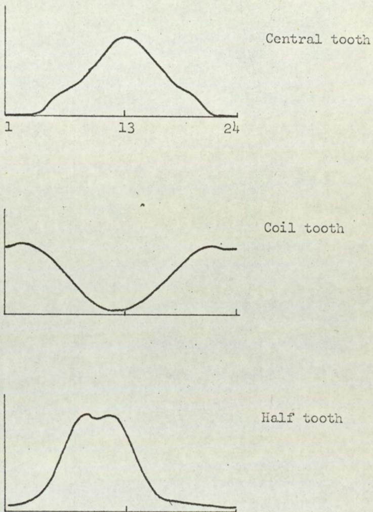
Fig 27: Cycles of variation in  $B$  ( $\propto V/l$ ) at centre of each tooth root from conducting paper analogue, see Table 1 for analysis.
