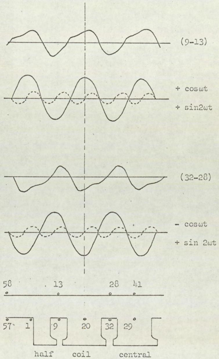
Fig 31: Comparison of flux waveforms behind consecutive armature slots
