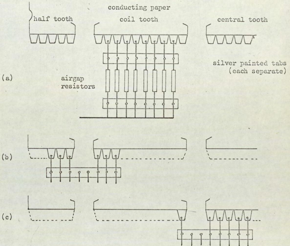
Fig 25: Detail of airgap surface 'tabs' on conducting paper analogue fed by resistors representing the airgap
