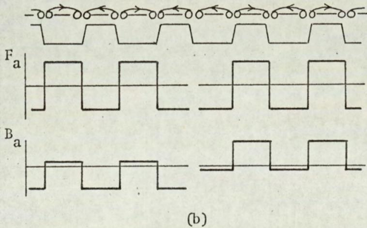
Fig 12: Peak reaction m.m.f.s and resulting flux-densities
