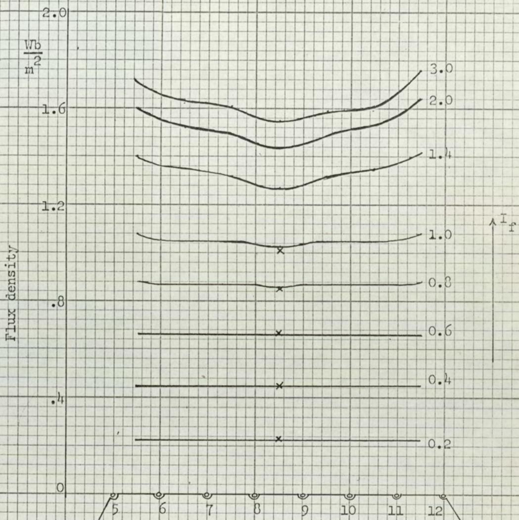
Fig 43: Distribution of flux density across rotor tooth surface - open circuit
