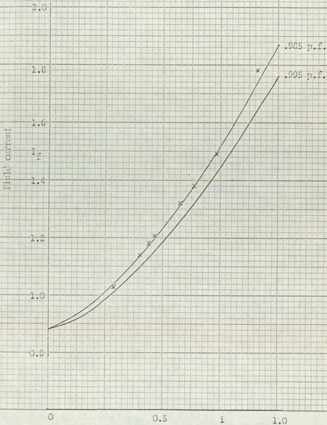
Fig 64: Field current against p.u. load current
