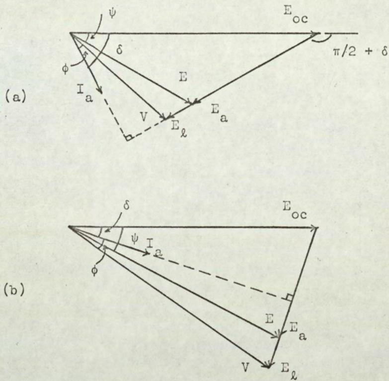
Fig 54: (a) lagging p.f. (b) leading p.f.
