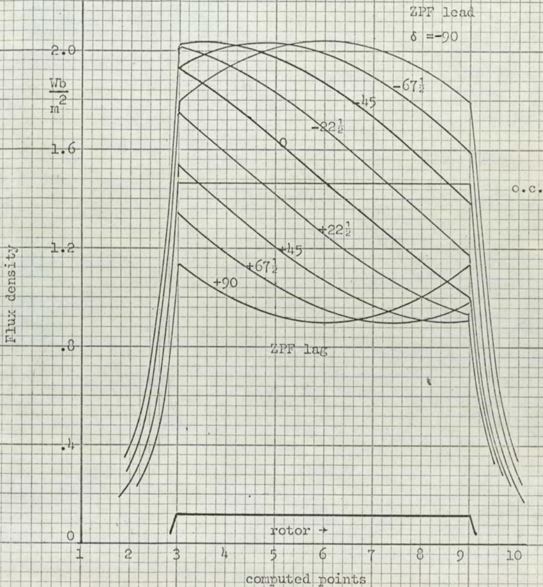
Fig 49: Flux density across a rotor tooth surface
