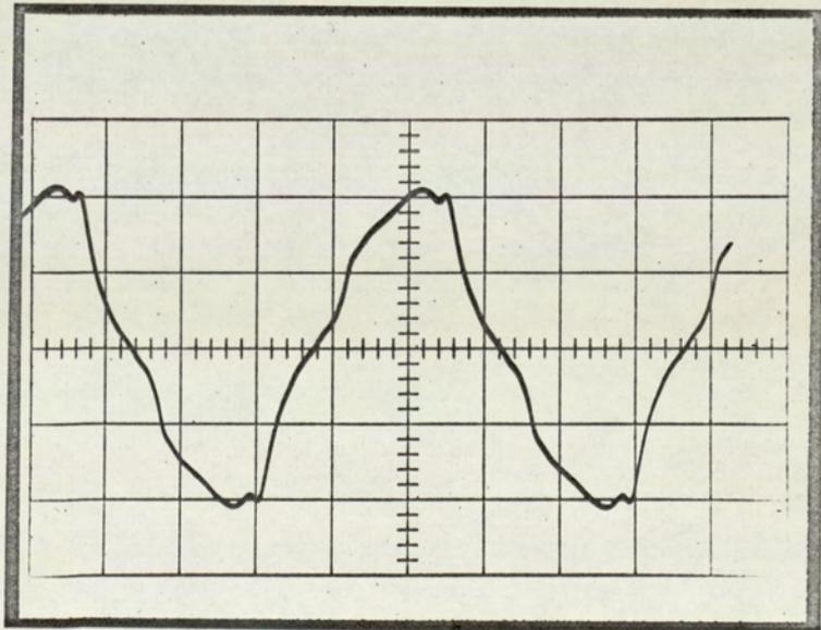
Fig 69: Output waveforms  $I_f = 1.5A$ (k)  $V_{oc} = 200$
