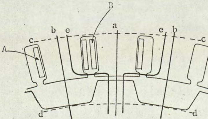
Fig 7: Flux paths between circles of equipotential m.m.f.
