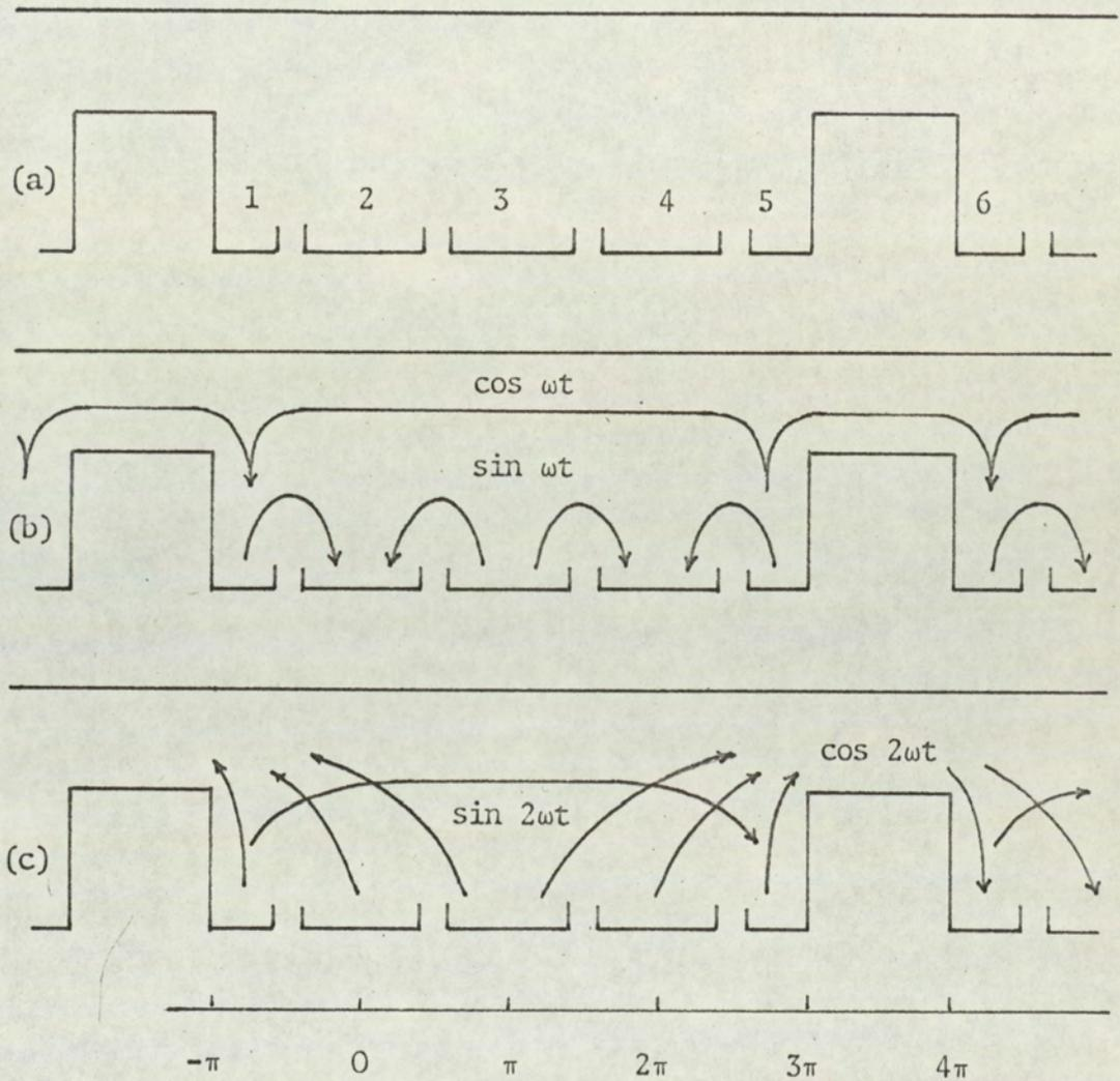
Fig 33: Distribution of open-circuit flux variations (even a.c. slots per d.c. pole)
