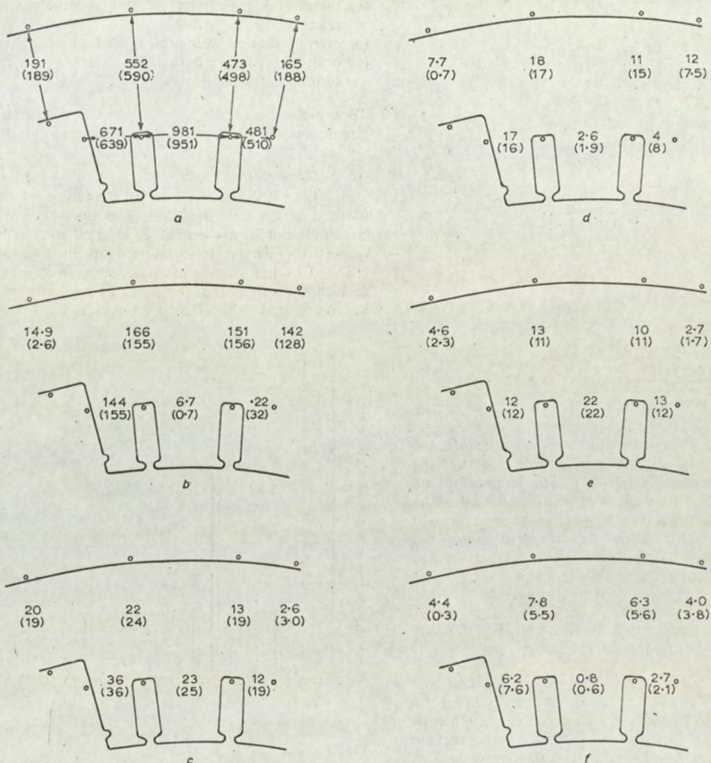
Fig 29: Harmonic components of peak flux, in  $\mu\text{Wb}$ , in core and teeth at rated open circuit voltage
