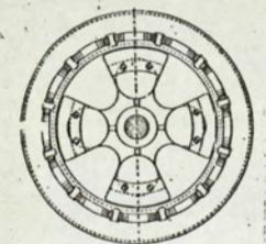
FIG. 7.—HOMOPOLAR INDUCTOR ALTERNATOR (OPPOSITE COIL).
