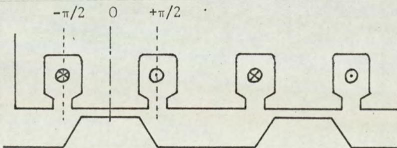
Fig 51: Basic inductor alternator airgap geometry with armature coil sense and rotor positioned for peak ZPF armature current condition
