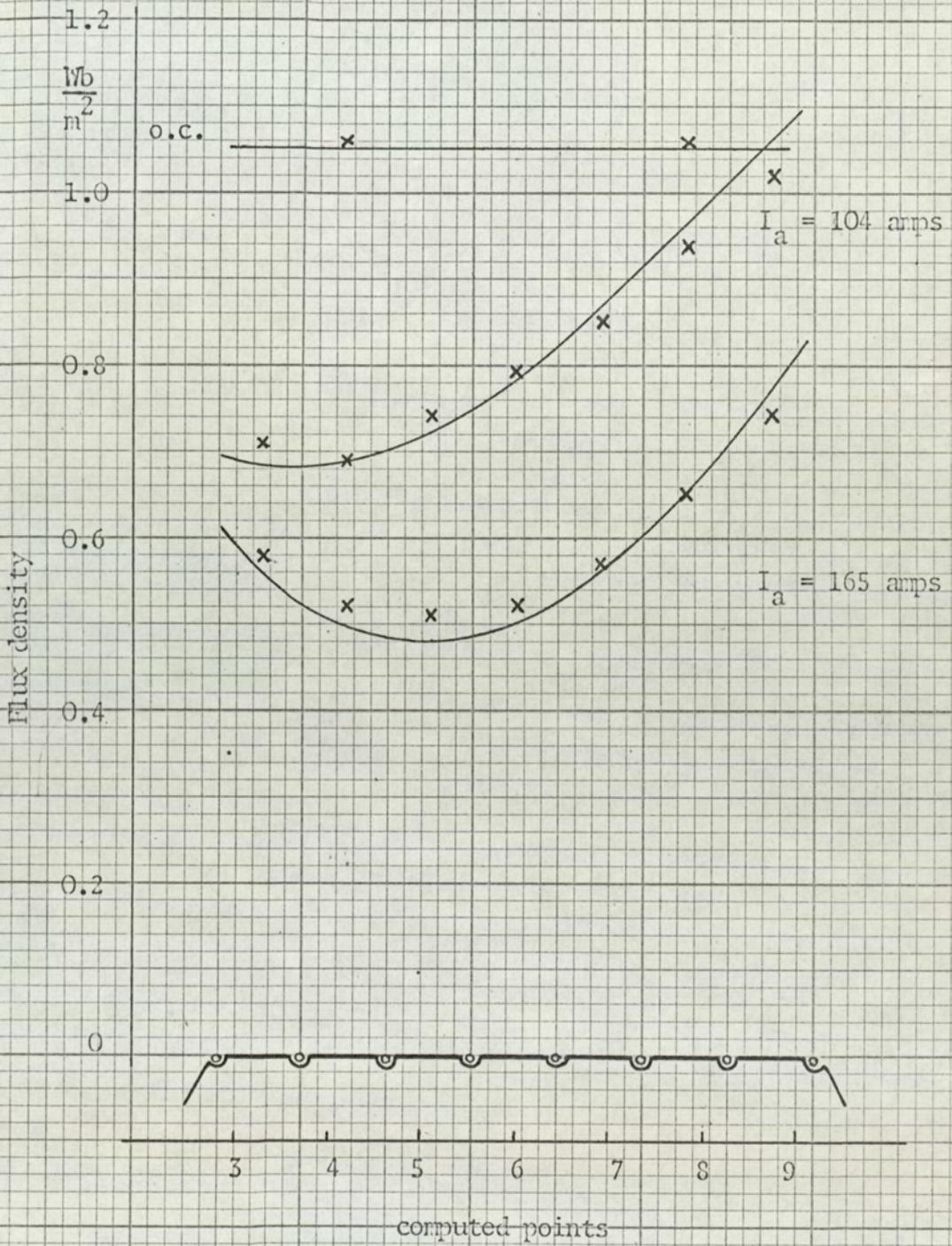
Fig 50(a): Flux density distribution across a rotor tooth surface on open-circuit and load,  $I_F = 1.0A$  see Table 11
