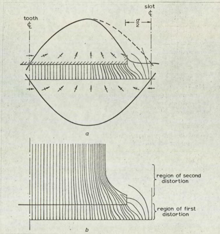
Fig 35: Postulated distortion of second-harmonic flux in tooth 2
