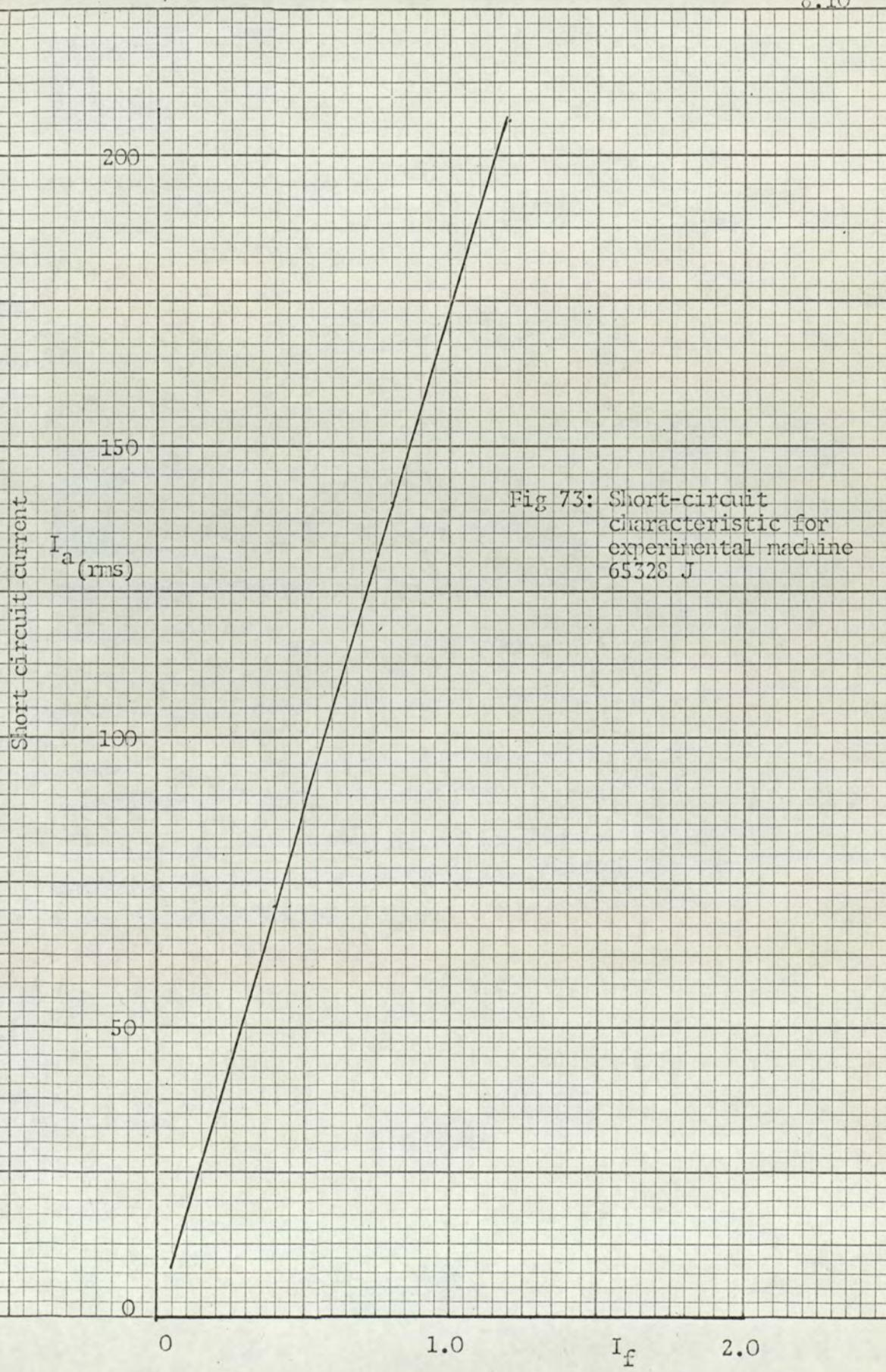
Fig 73: Short-circuit characteristic for experimental machine 65328 J
