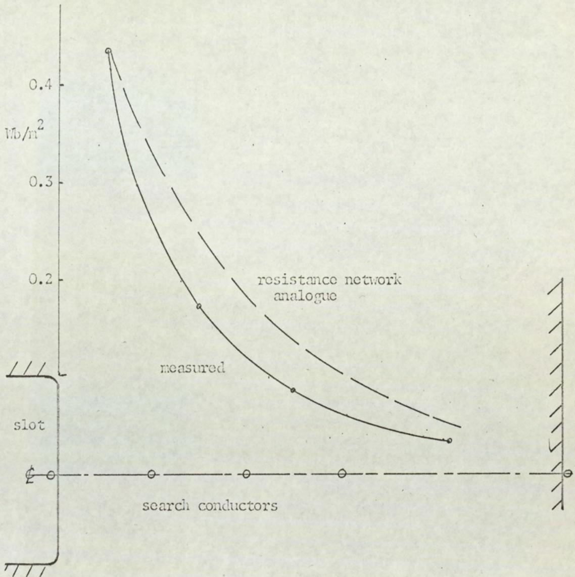
Fig 67: Density of fundamental flux passing behind armature slot, at open circuit rated volts undamped
