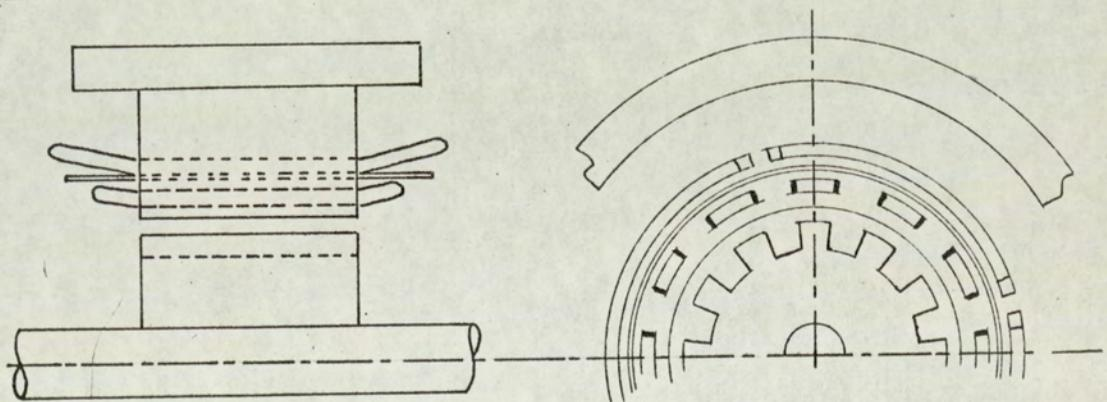
Fig 4: Heteropolar inductor-alternator
