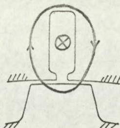
Fig 68: Rotor surface path for armature reaction flux
