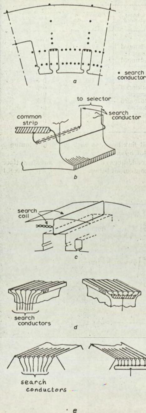
Fig 20: Details of search conductors
