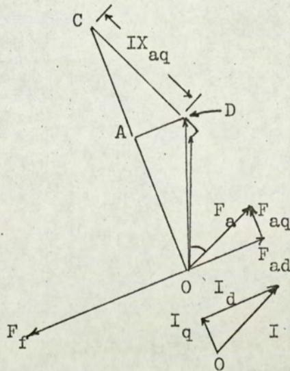
Fig 15: Vector diagram of polyphase inductor generator on-load, reference 30
