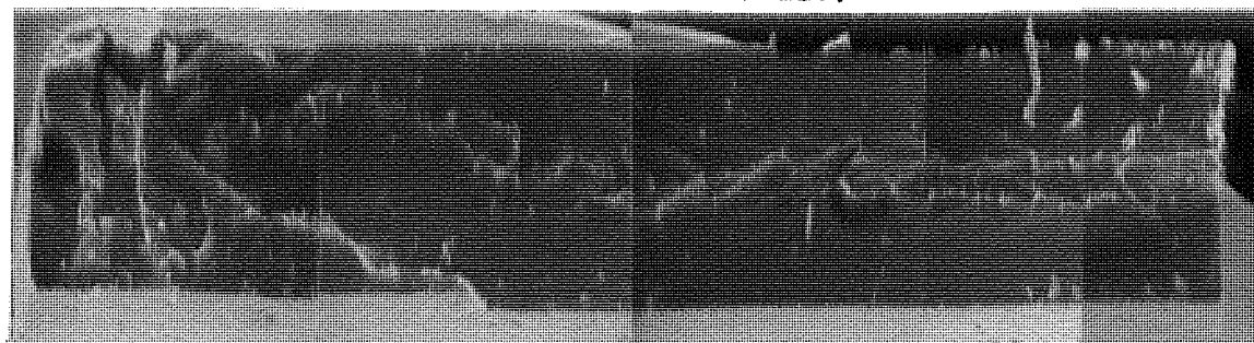
Styrene-Butadiene tear from razor cut at left-hand end.
