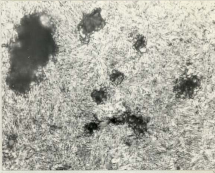
Fig.59. Typical Microstructure of M 1 series of Maraging Steel (M.S.) Compact. Sintered and Heat-Treated (S.H.T.)
