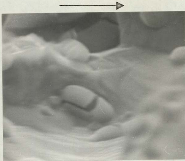
Fig.85(a). Split Ti(C,N) Particle in the Fracture Surface.
