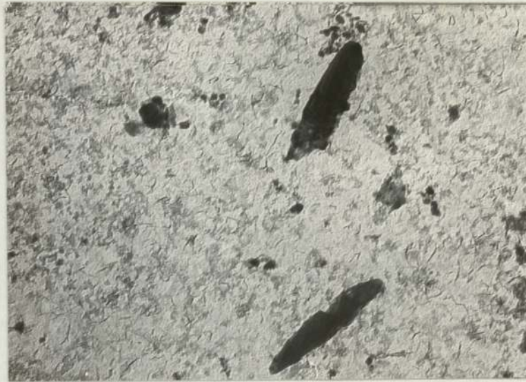
Fig.90. Extraction Replica Micrographs of (a) \text{Ni}_3(\text{Al},\text{Ti}) Precipitates and
