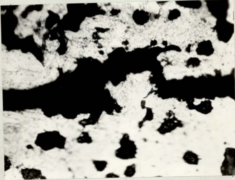
Fig.73. Crack-Forking and Arching.
