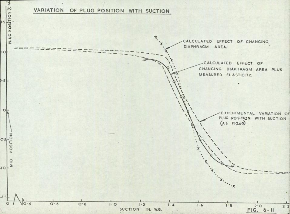
curve of Fig. 6-7 has been re-plotted on Fig. 6-11.
