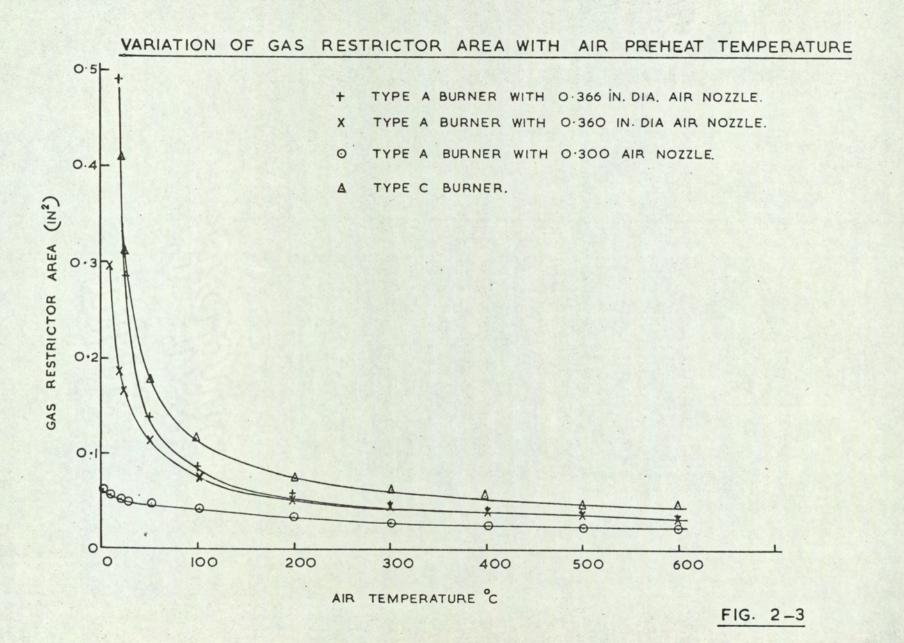
is necessary to compensate for changes in air preheat. In view of this the variation of air/gas ratio with temperature was calculated for an A Type burner having an undersized air nozzle (0.300 in. dia. instead of 0.366 in. dia. for a 1 in. dia. tunnel) and for which the gas restrictor was adjusted to give a stoichiometric ratio at a preheat temperature of  $500^{\circ}C$ .
