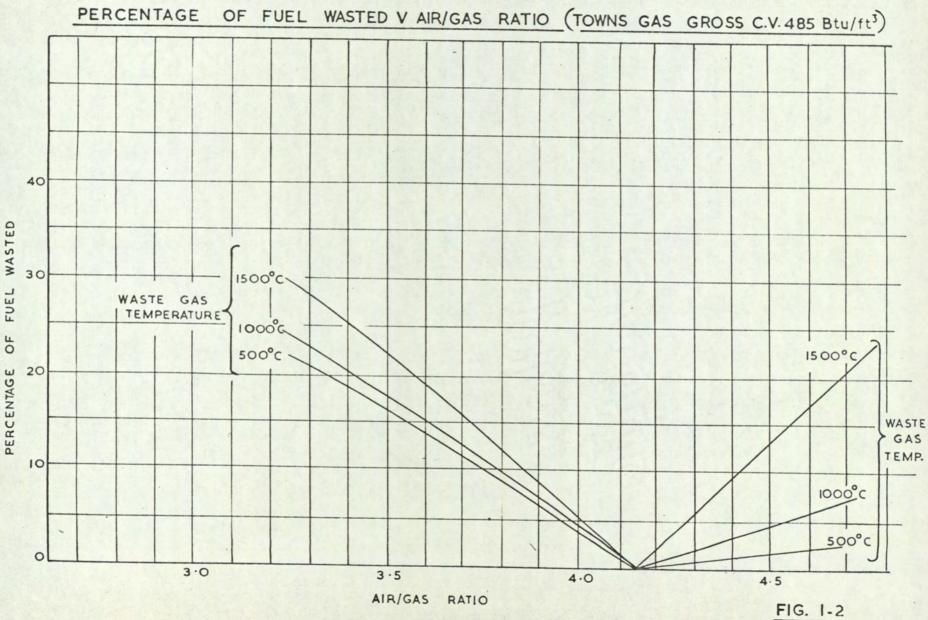
practical value can be obtained by dividing the gross calorific value by 117. During the course of this work a number of changes in gas composition (increasing the calorific value) were made by the West Midlands Gas Board. As a result, various values of the stoichiometric air/gas ratio, ranging from 3.8:1 to 4.15:1, are referred to in this paper.
