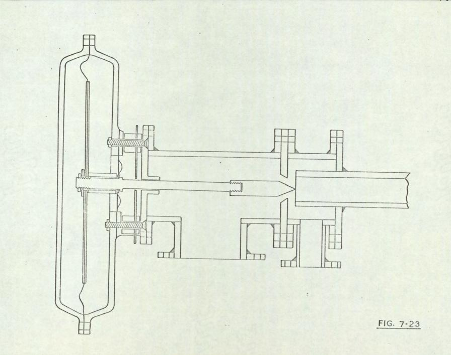
a 1/4 inch thick disc inserted into the inlets to the motor diaphragm chambers, hunting of the system was eliminated.
