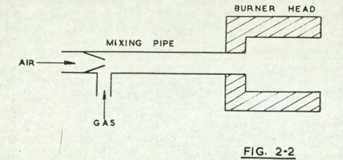
trimming the air/gas ratio to allow for the dimensional tolerances of the burner. The gas restrictor is usually adjusted when the burner is commissioned and thereafter the burner throughput is controlled by means of a valve in the air supply line.
