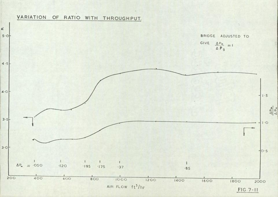
and the results shown in Fig.7-11 were obtained after the system had been disturbed and the bridge readjusted to give  $\frac{\Delta P_a}{\Delta P_g} = 1$  at maximum throughput.
