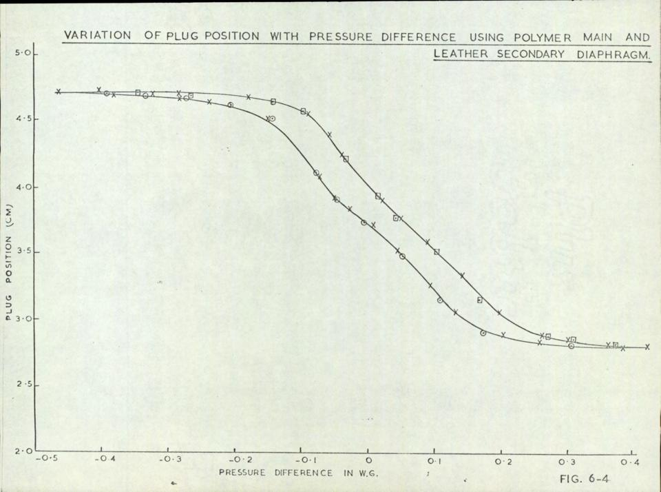
see Fig. 6-5, and the plug position measured with a travelling microscope. In the case of the air diaphragm a measured pressure was applied to the underside of the diaphragm and in the case of the gas diaphragm a measured suction was applied to the upper side of the diaphragm. Thus both diaphragms took up the shape they would have when the injector was working normally.
