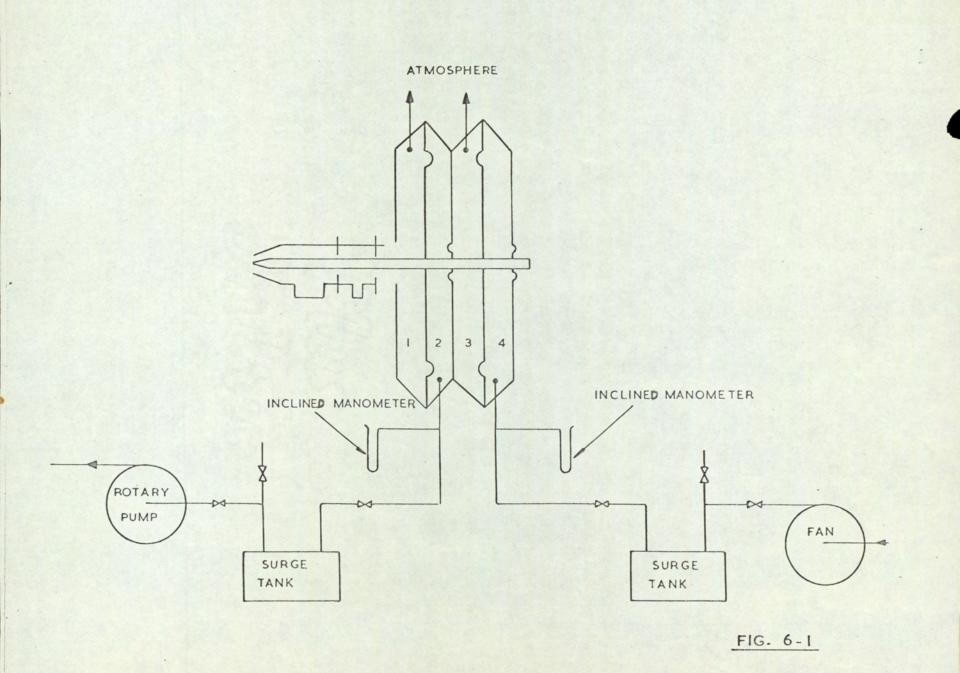
was then slightly reduced and the measurements repeated. This process was continued until the pressure applied to chamber 4 was about 0.25in. w.g. when the process was reversed and measurements taken at a series of increasing pressures applied to chamber 4.
