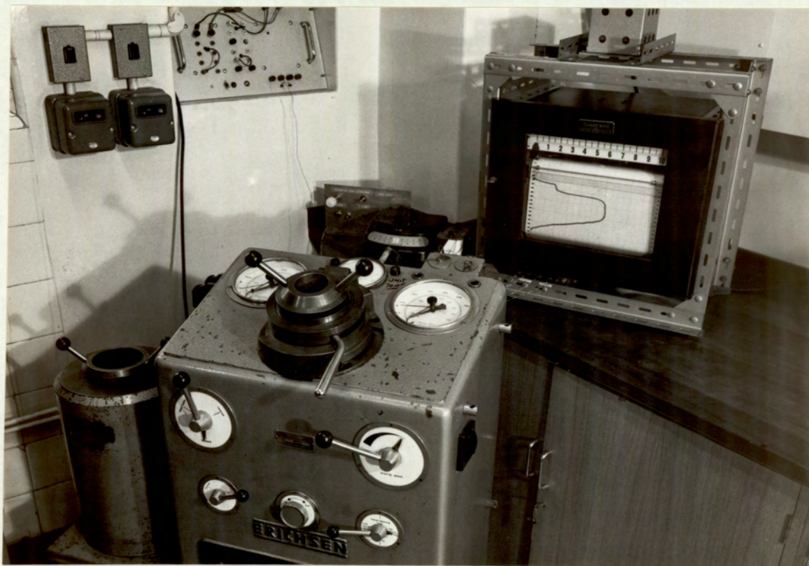
Fig. 3.11. The Erichsen Model 123 Electro-Hydraulic Press with Recording Equipment.
