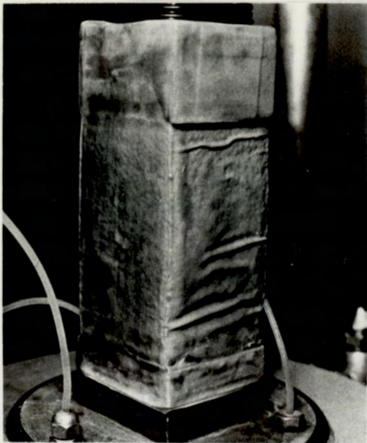
FIG.6.4(b) INT 2, \sigma_x AND \sigma_y FACES AFTER REMOVAL OF SIDE STRESS-CELLS
