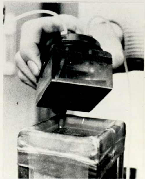
FIG.4.9(c) PLACEMENT OF TOP STRESS-CELL
