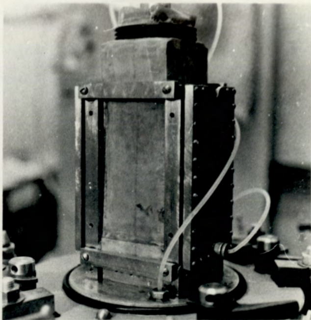
FIG.6.5(a) ATA TRIAXIAL EXTENSION TEST TEST STOPPED AT FAILURE ATA TE 1 e_i = 0.548 , \epsilon_3 = -5.75\%
