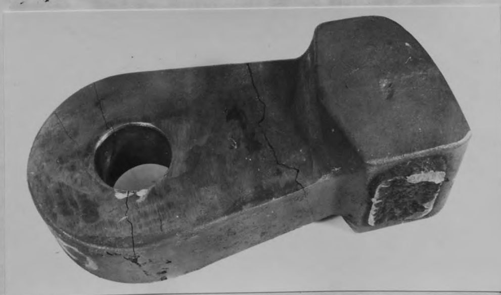
Fig. 2.4. Broken Reinforced Hammer Head.
