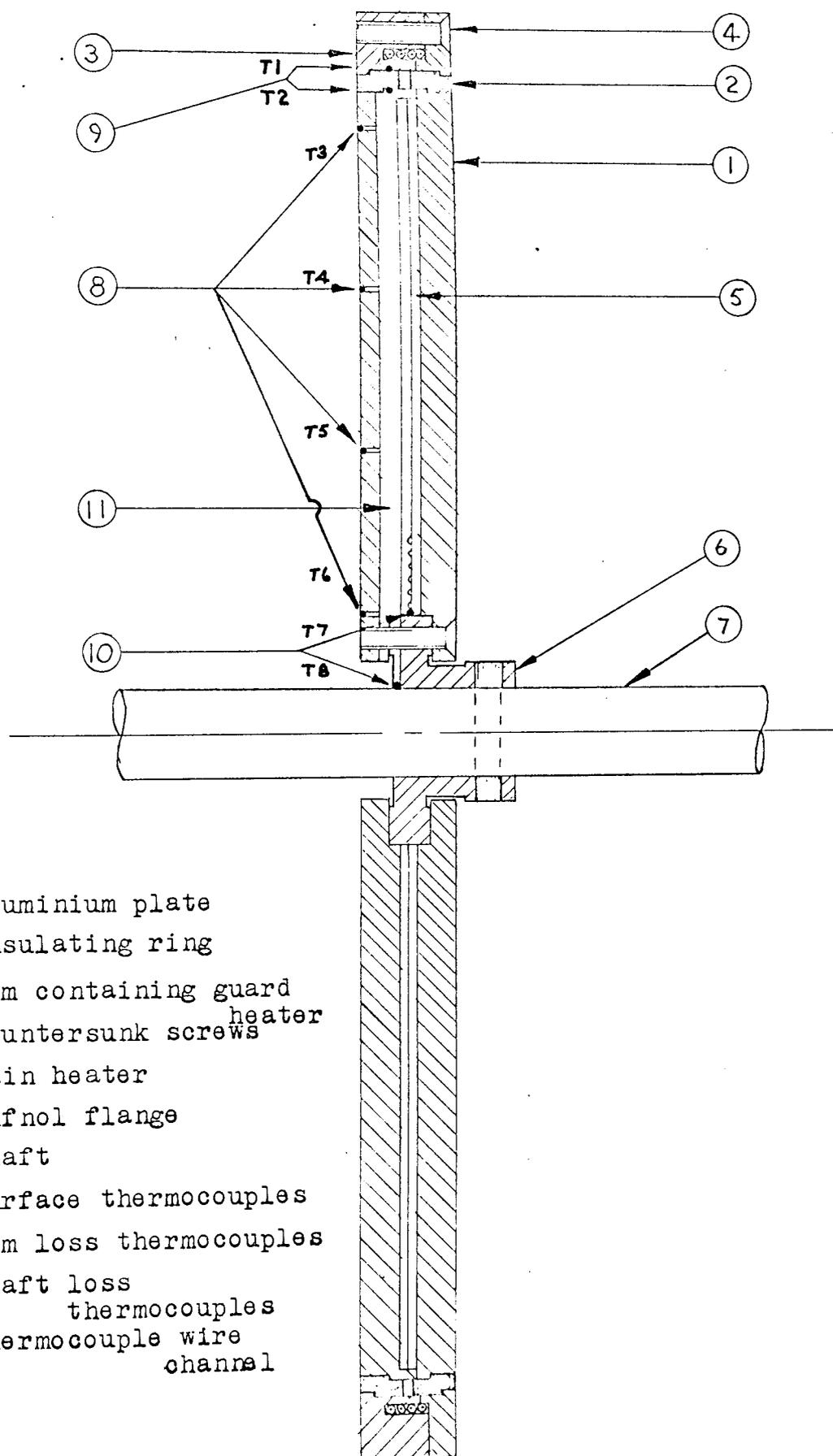
The resistance of the main heater was 120 ohm at 20°C.
