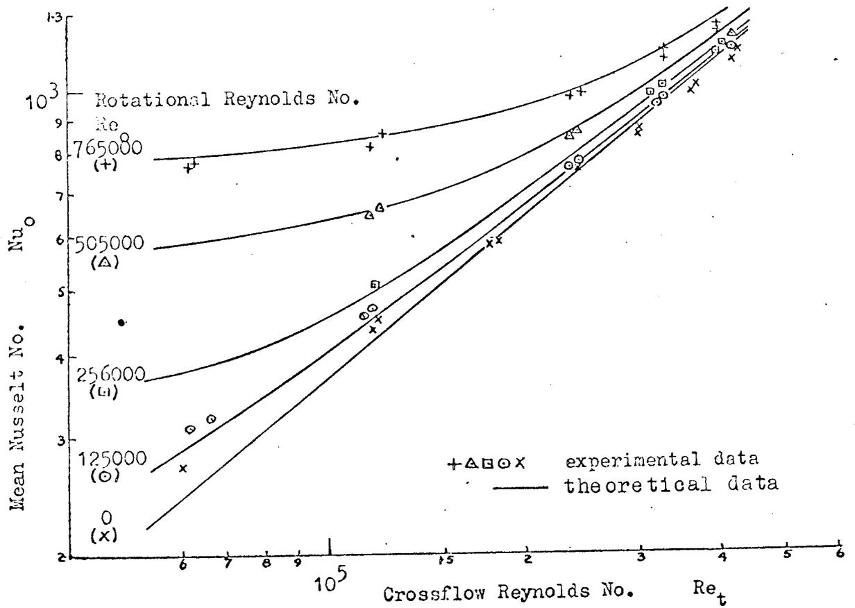
The two systems are superimposed in the manner just explained but the length  $x$  is calculated from the main disc edge instead of from the guard rim edge. The results are presented in non-dimensional form in figure 4.28, which will be used as a data sheet for the prediction of disc brake operating temperatures.
