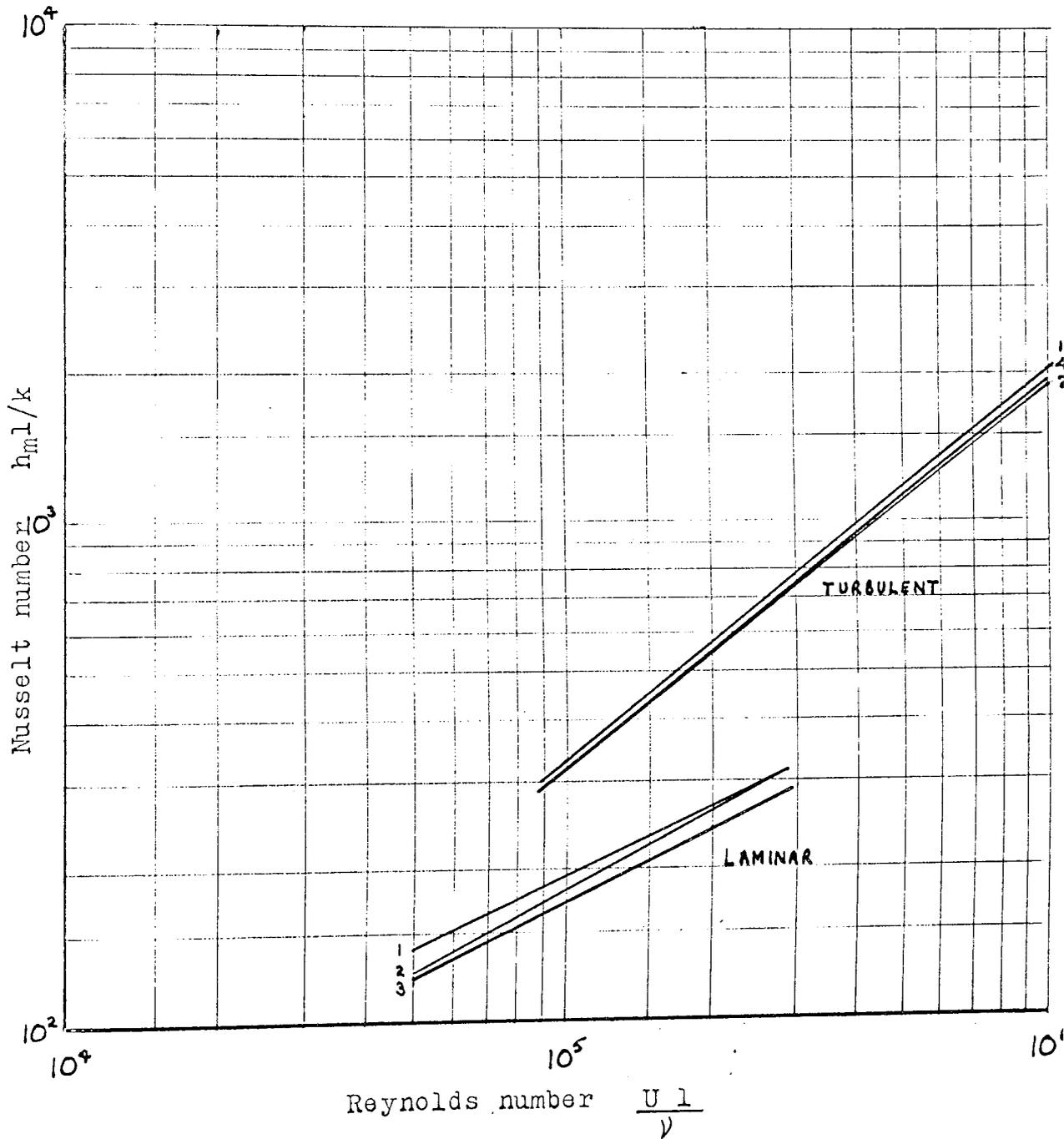
which is dependent on the distance of the point being considered from the leading edge of the plate. In fact  $h_{\text{local}} \propto \frac{1}{x^{0.2}}$  for
