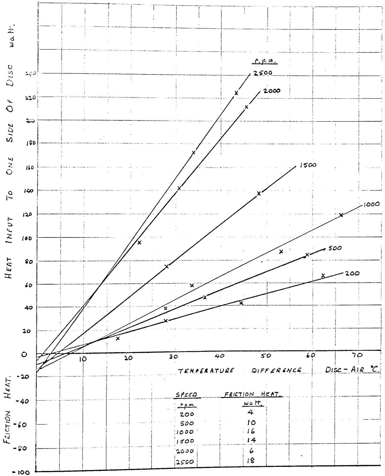
the line back through the origin. This facility is included in the computer programme CVAE 22, which processed the experimental results.
