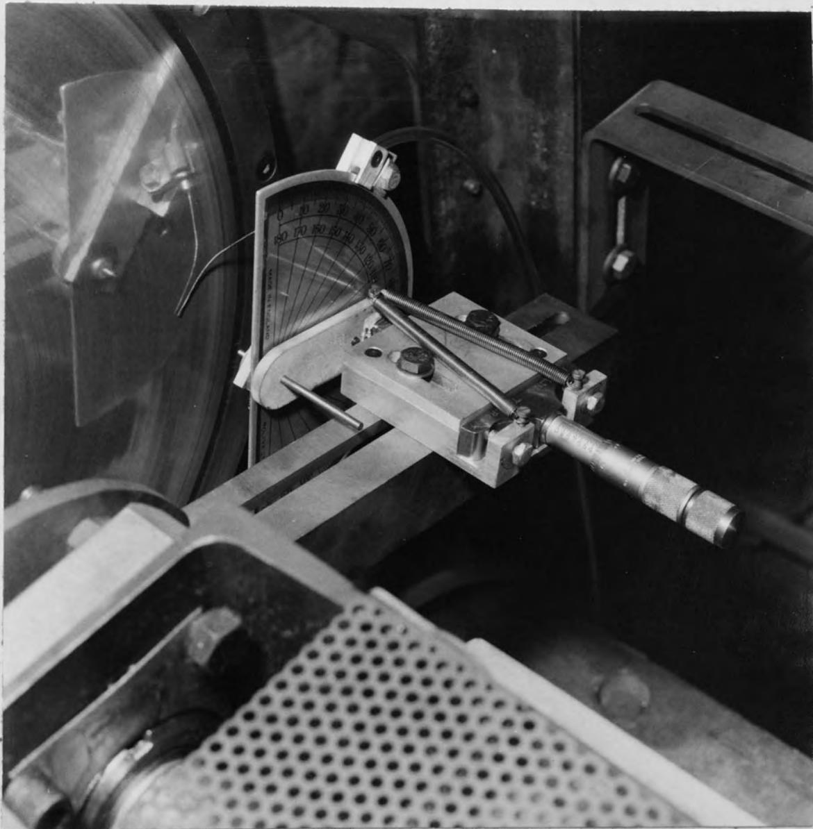
When the ambient temperature was measured in the ambient it was found that those thermocouples on the hotter side of the disc consistently indicated higher temperatures, due to recirculation from the hotter surface. Therefore the best transfer calculations were made on the cool side of the disc only, as the surface whose temperature was
