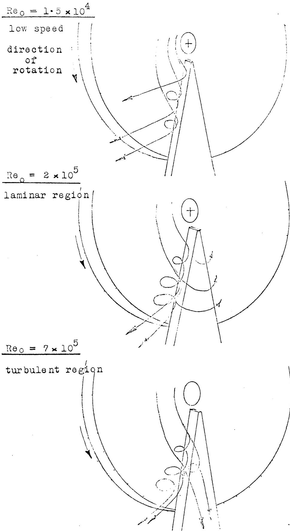
Note: no shield to prevent recirculation of flow
