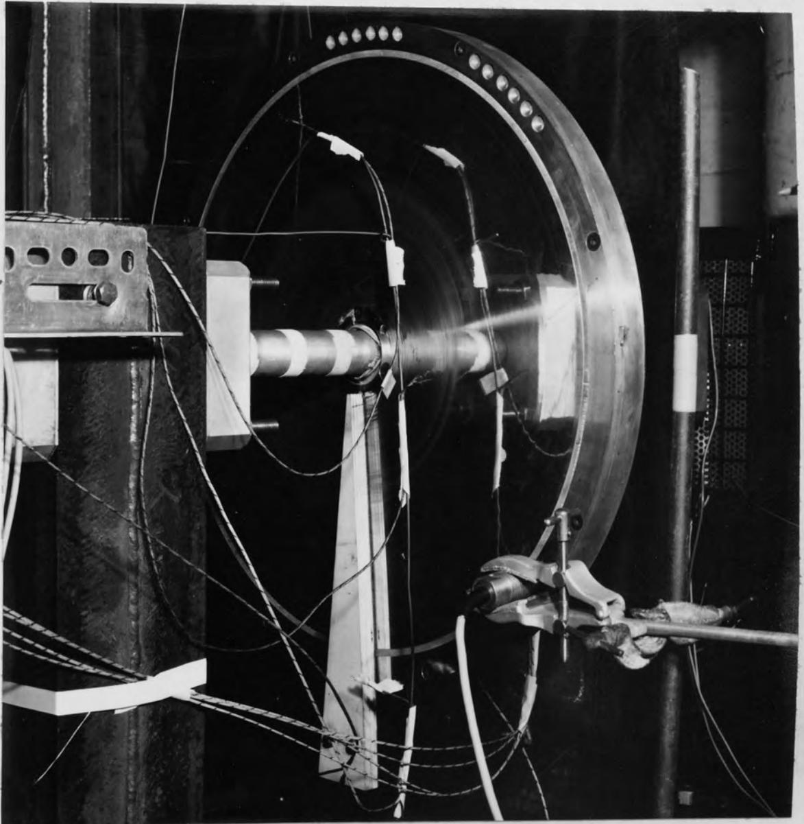
Example of Measurement of Friction Heating on 180° Sector
