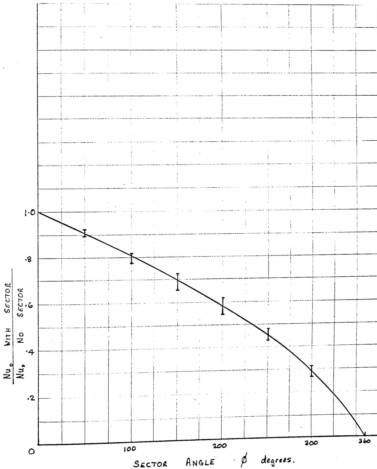
In figure 4.30 the experimental curve, even when corrected for the thermocouples not reading the mean surface temperature, gives results above the theoretical data. This deviation was probably due to separation of the flow at the leading edge, causing a non-uniform surface temperature, which was more marked with the disc stationary than when rotating, and was not allowed for in the analysis.
