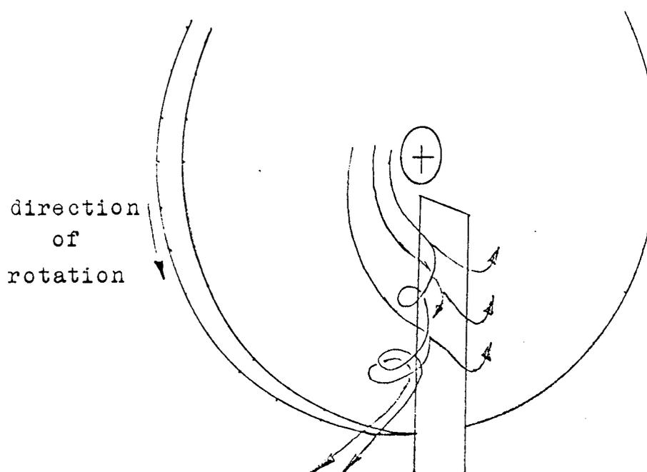
the improvement in the heat transfer due to the slight swirl ahead of the scraper was counteracted by an increase in the area under laminar flow behind the scraper. Without the shield some flow recirculated over the scraper and turbulent flow continued as with a free disc, producing a higher overall heat transfer due to the swirl ahead of the scraper.
