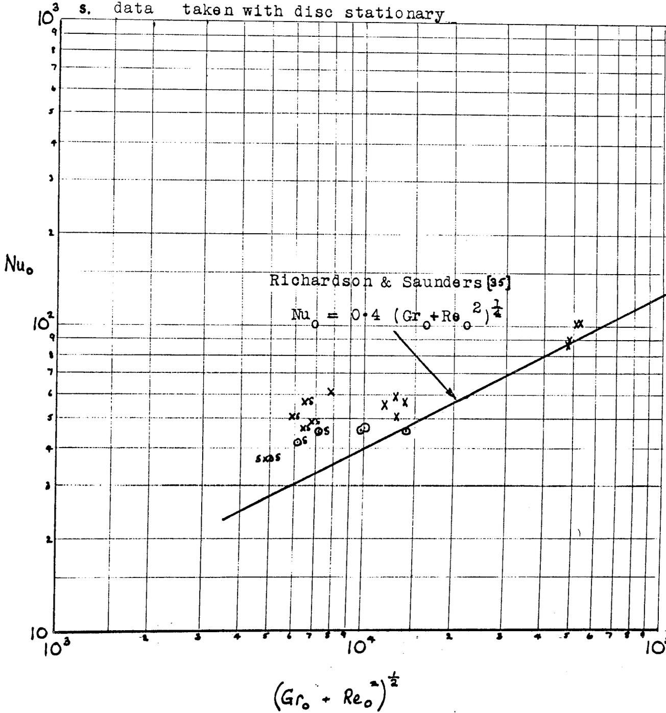
difference whereas the slowly rotating disc was uniform to within 1%. Therefore it is assumed that the heat transfer from the stationary disc was increased due to a non-uniform surface temperature.
