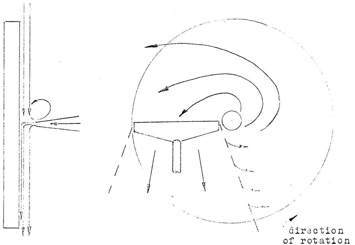
low nozzle jet velocity, high rotational speed
