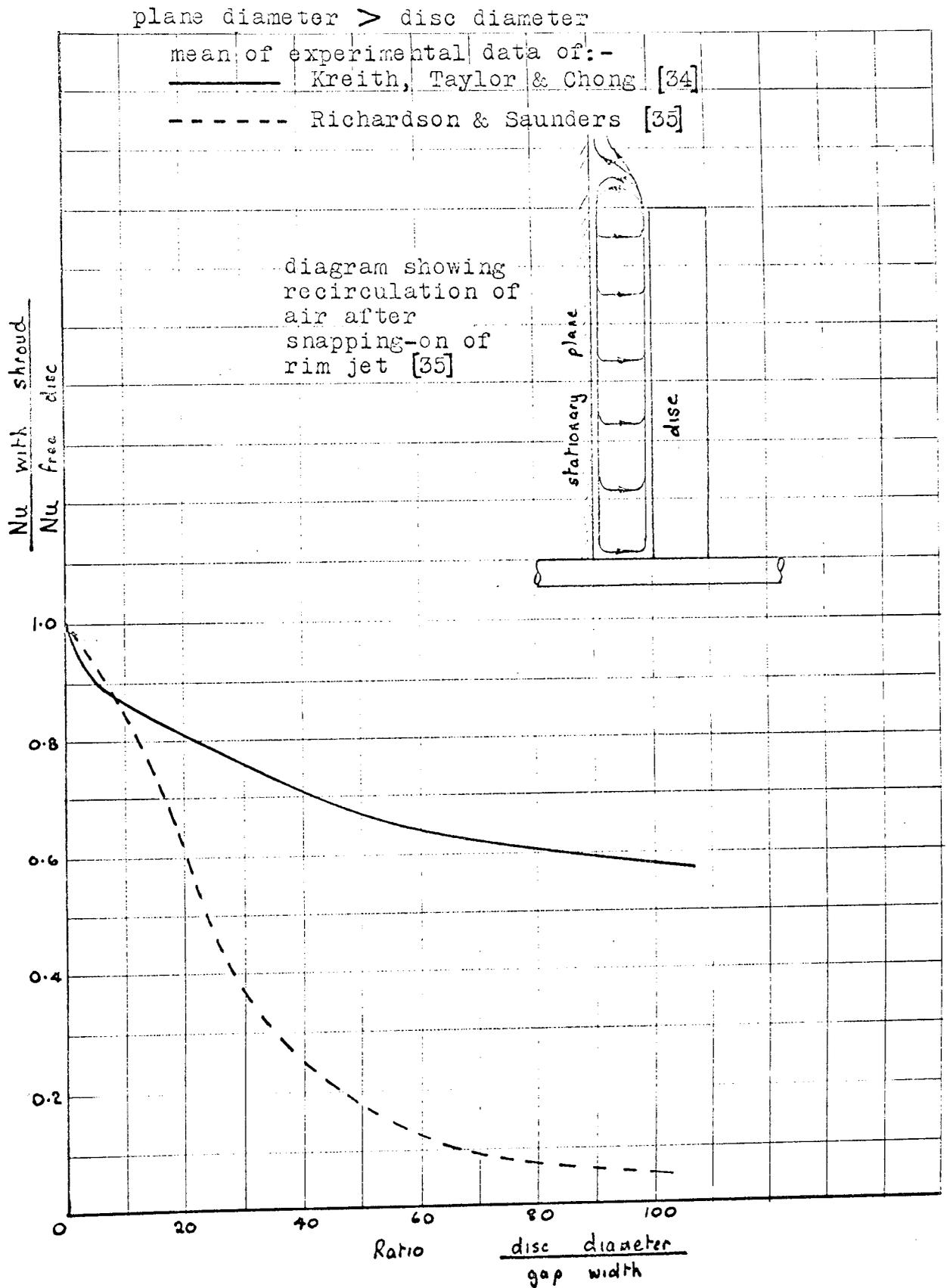
reducing the heat transfer. This accounted for the discrepancy between the results of Kreith, Taylor & Chong and those of Richardson & Saunders, the mass transfer technique could not allow for the increased approach temperature of the entrained fluid.
