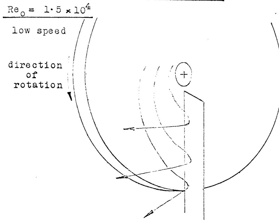
Note: no shield to prevent recirculation of flow
