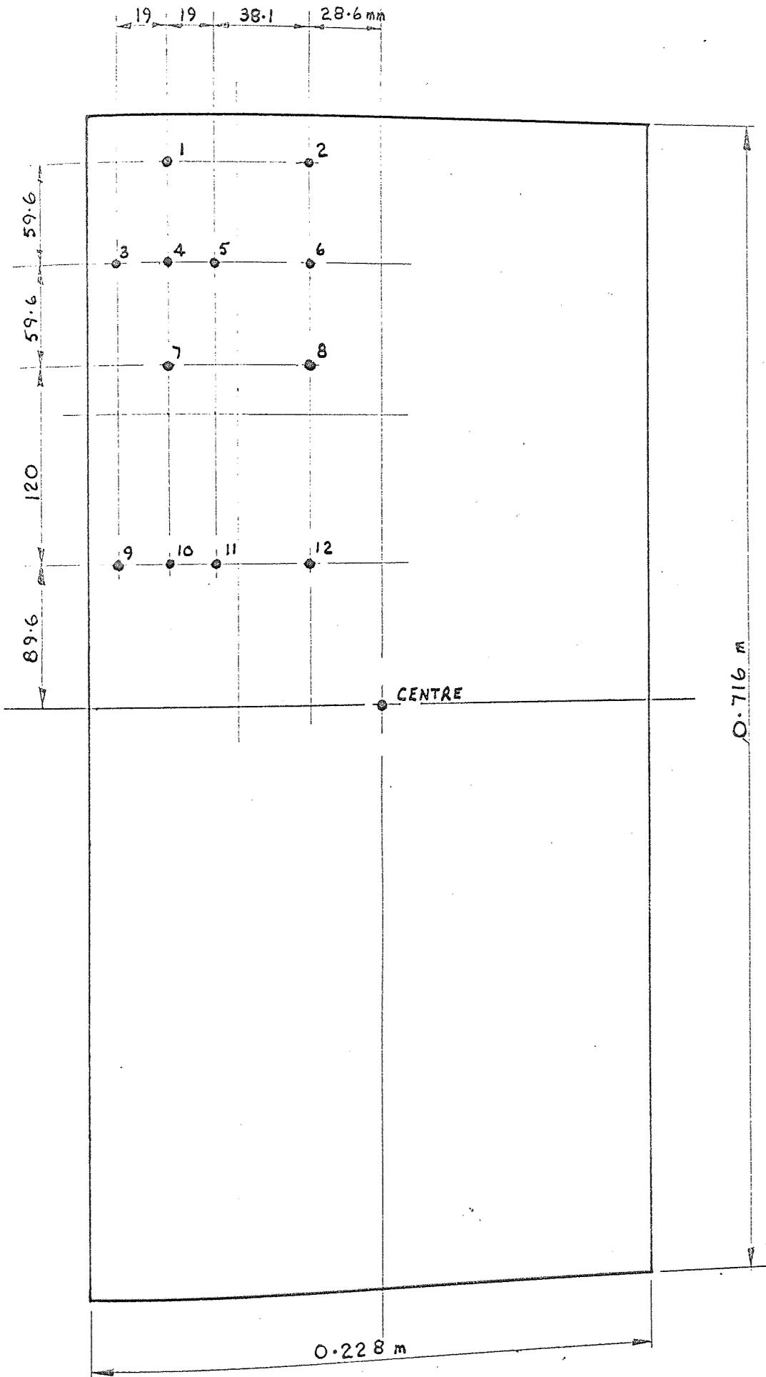
Exploration of Airflow at Entrance to Wind Tunnel
