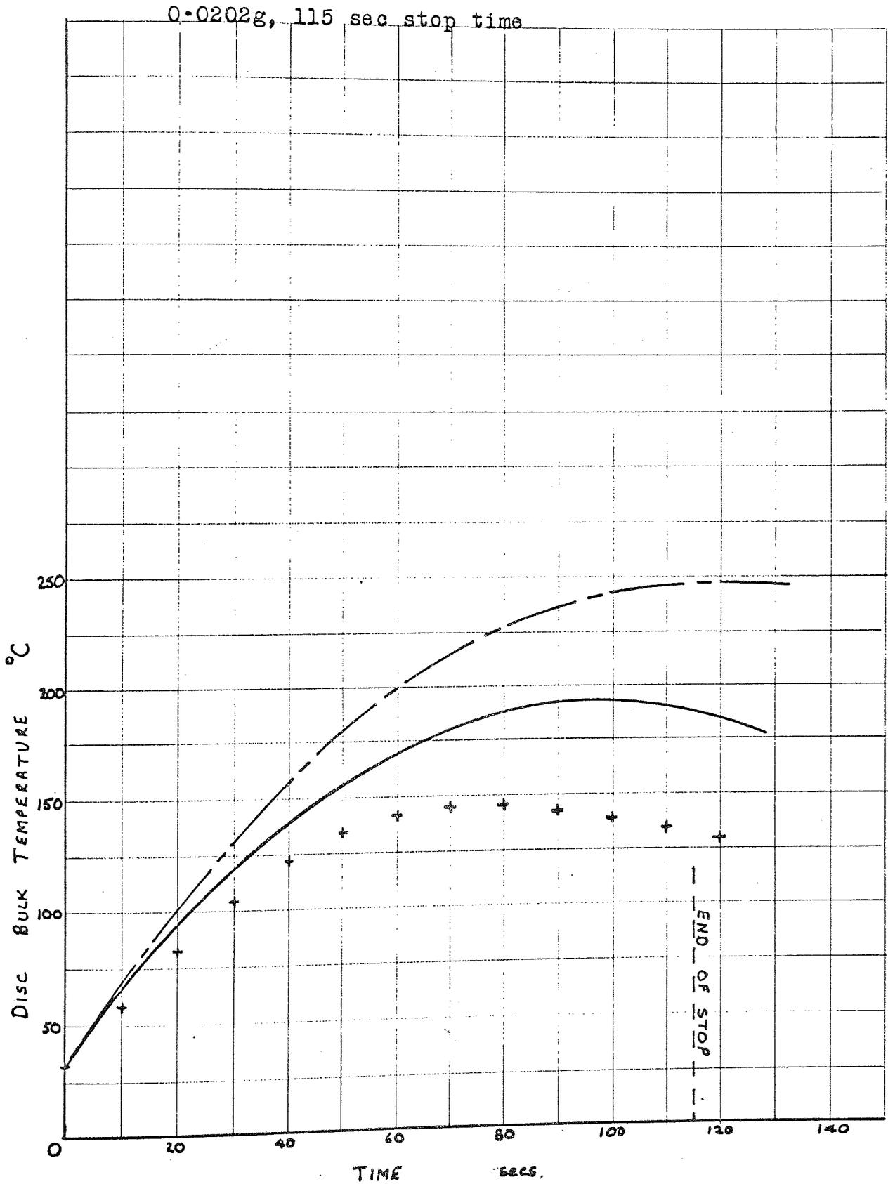
Comparison of Experimental and Theoretical Results for 16P Caliper on 28.1 cm diameter disc with constant energy input
