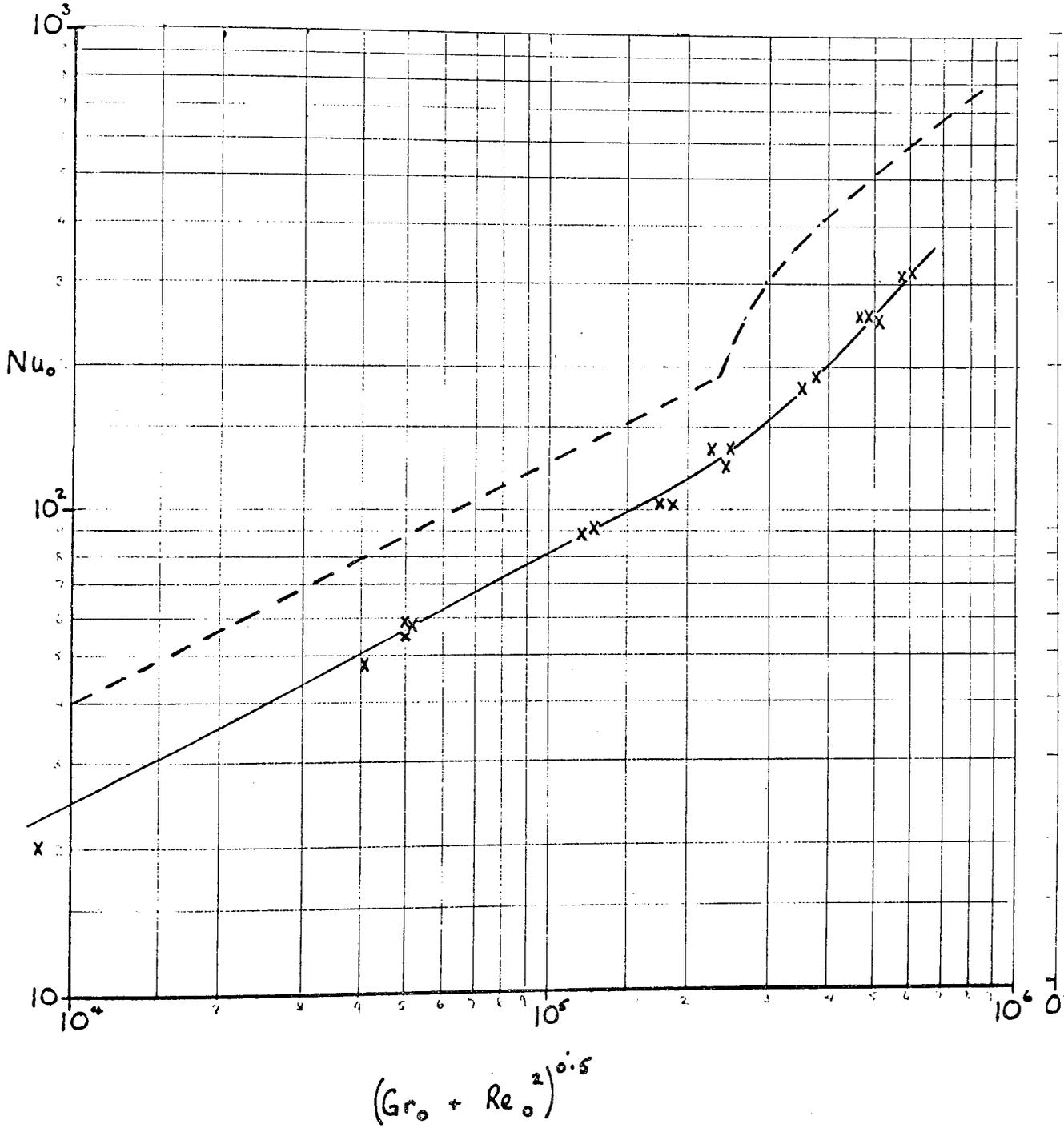
Heat Transfer from a Rotating Disc in Still Air
