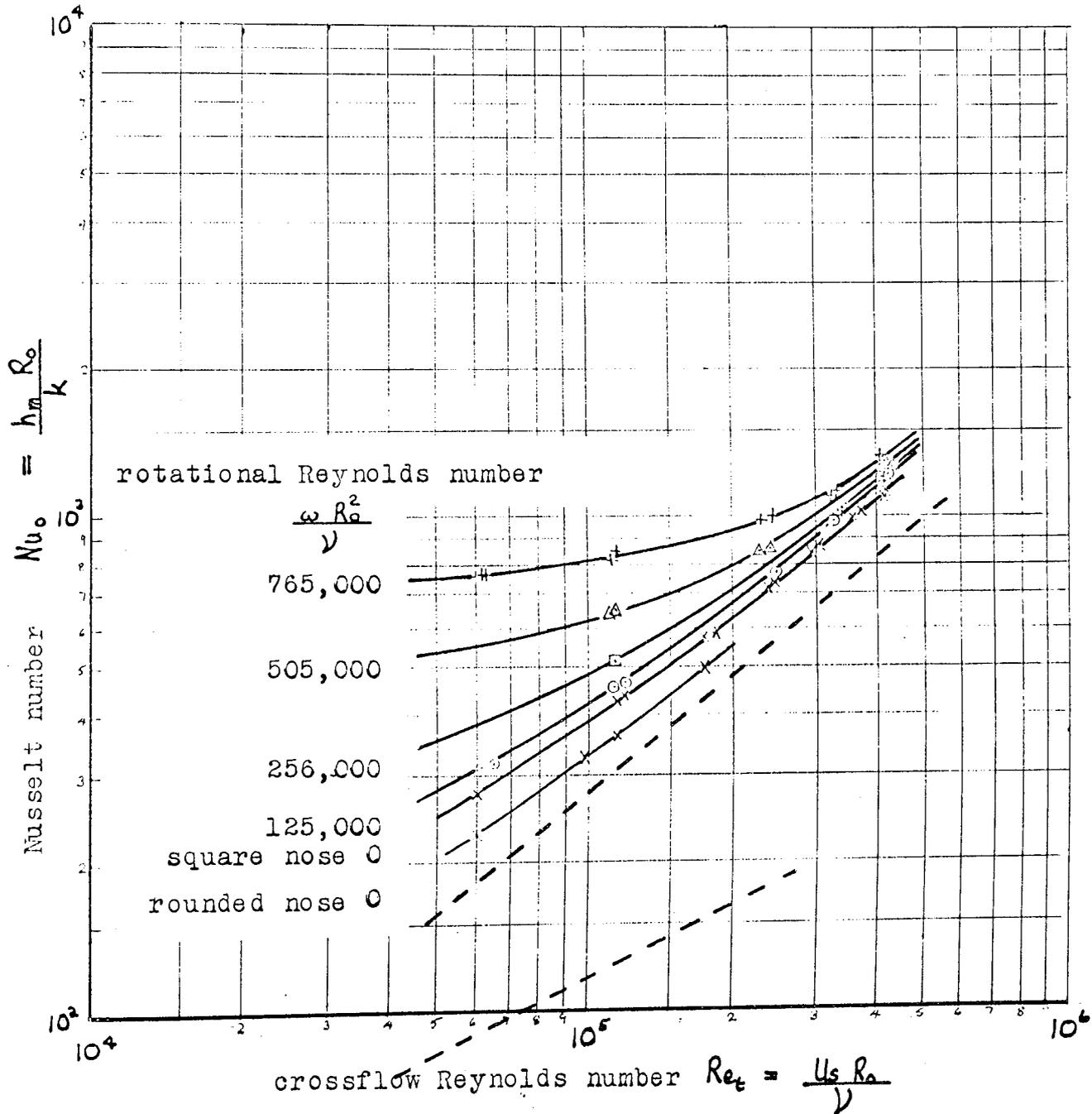
Experimental Data for the Heat Transfer from a
