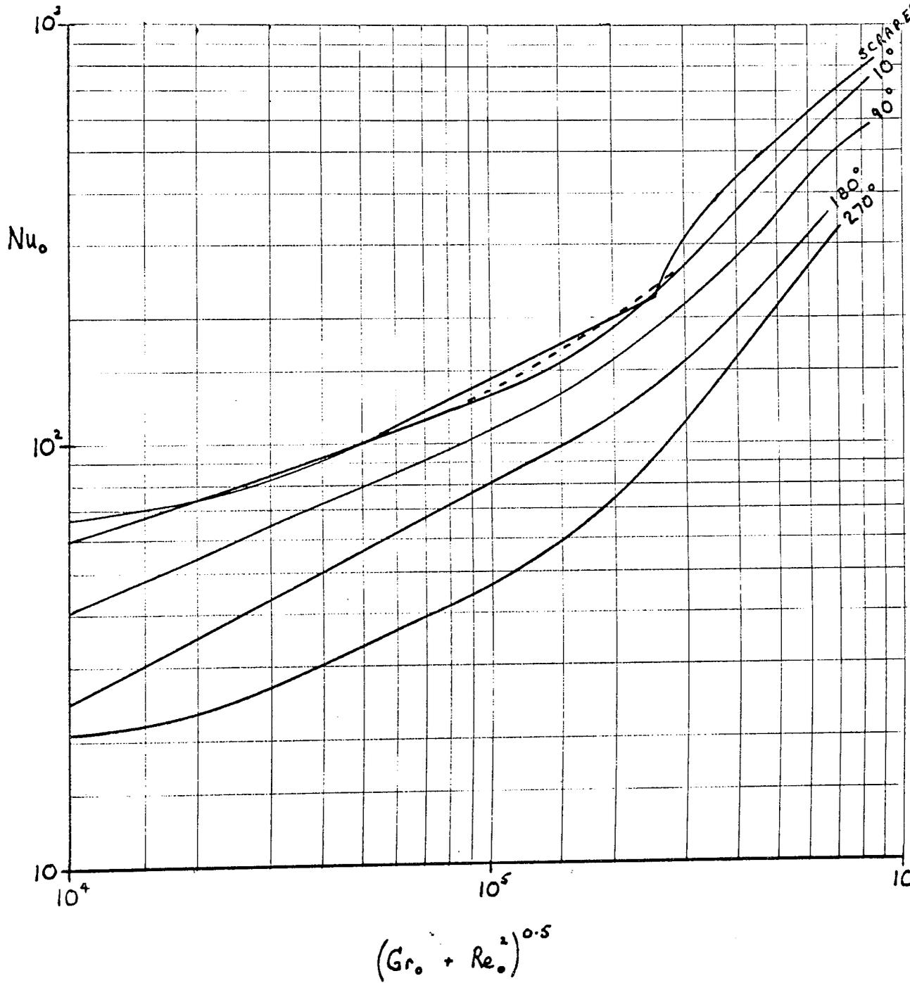
Effect of varying the sector of Disc masked off on the Heat Transfer from a Disc rotating in Still Air at a Reynolds number of 120,000
