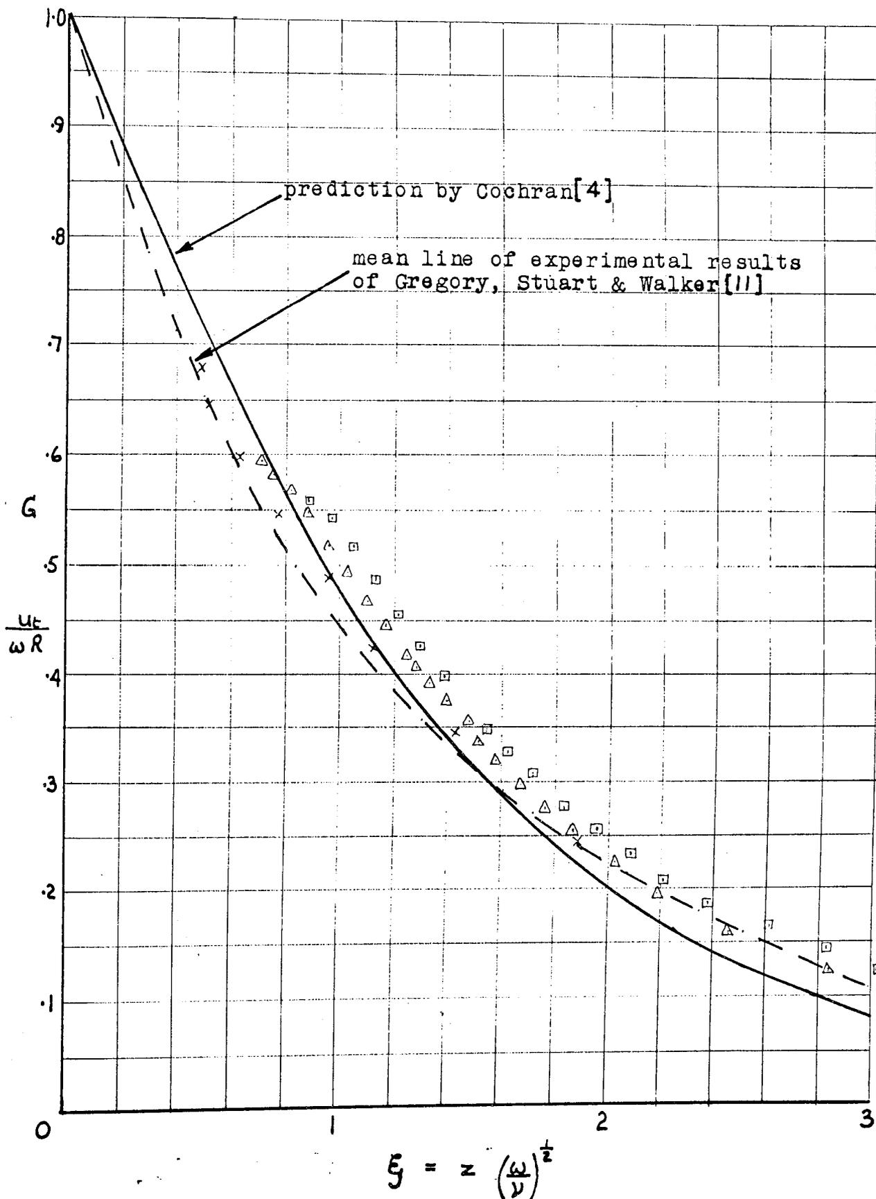
Angle of Yaw of Airflow on a Rotating Disc
