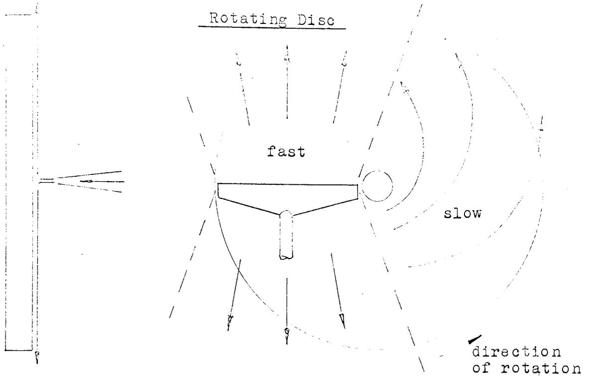
high nozzle jet velocity, low rotational speed
