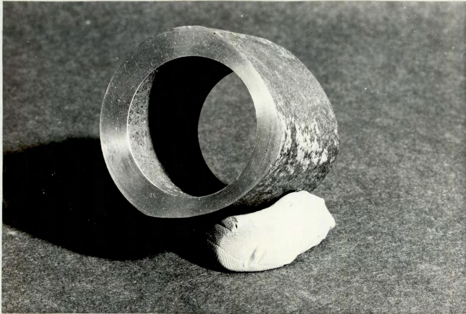
FIG. 2-2 SECTION THROUGH A CORRODED BOILER TUBE
