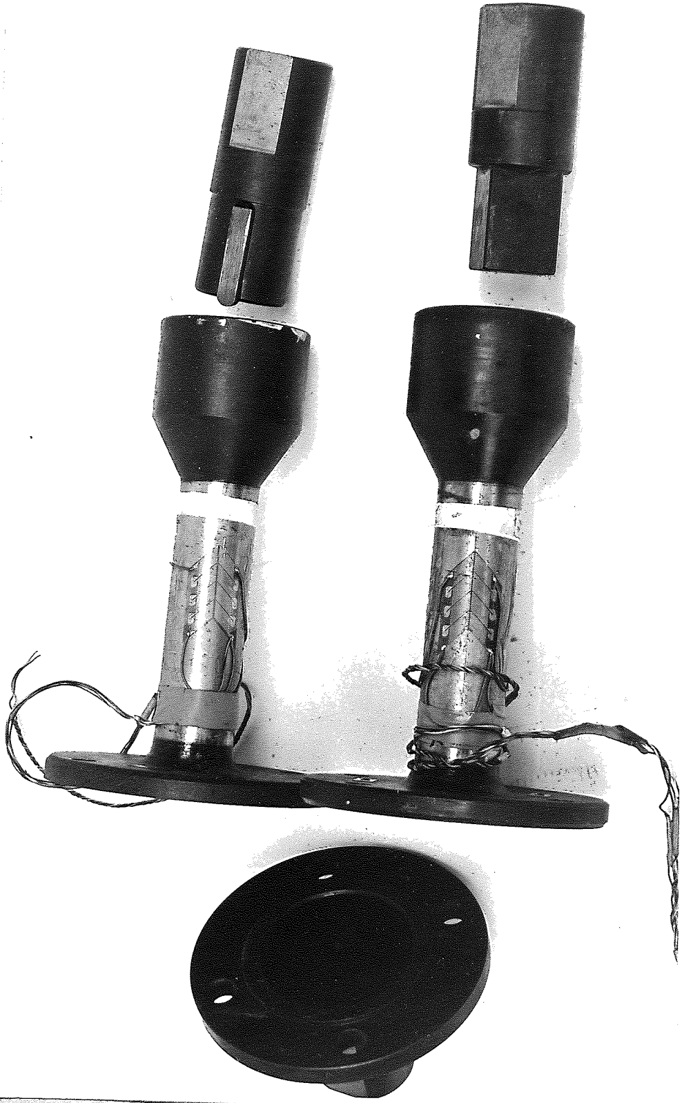
Figure 27. Torque meters with adaptors for calibration.
