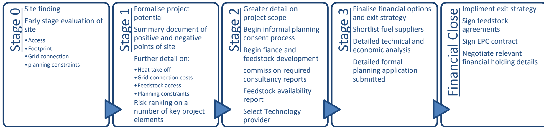
Figure 3.3: Example of a stage-gated project development approach for a bioenergy power scheme
