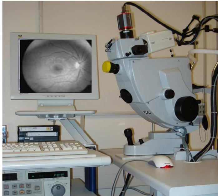
**Figure 3.2 Dynamic retinal vessel analyser (DVA)**
