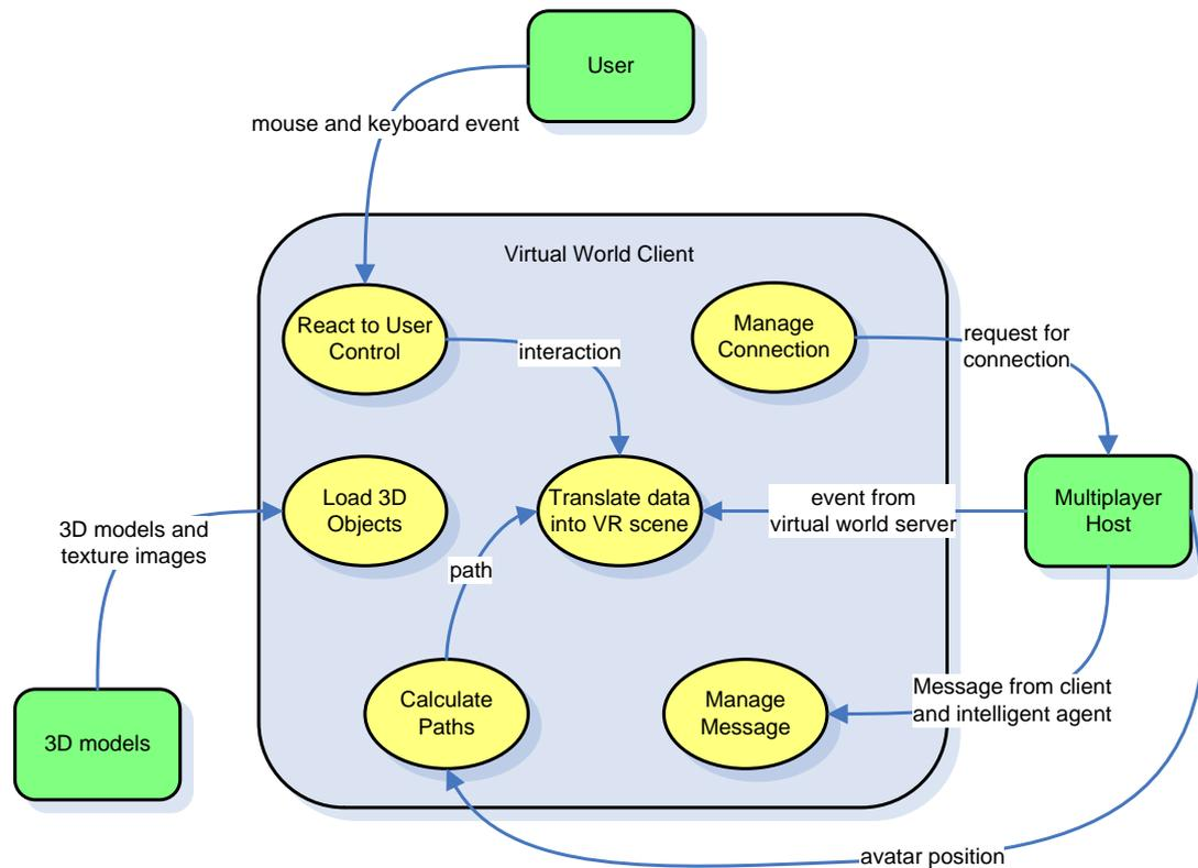
**Figure 9-6: Logical flow of virtual world client**
