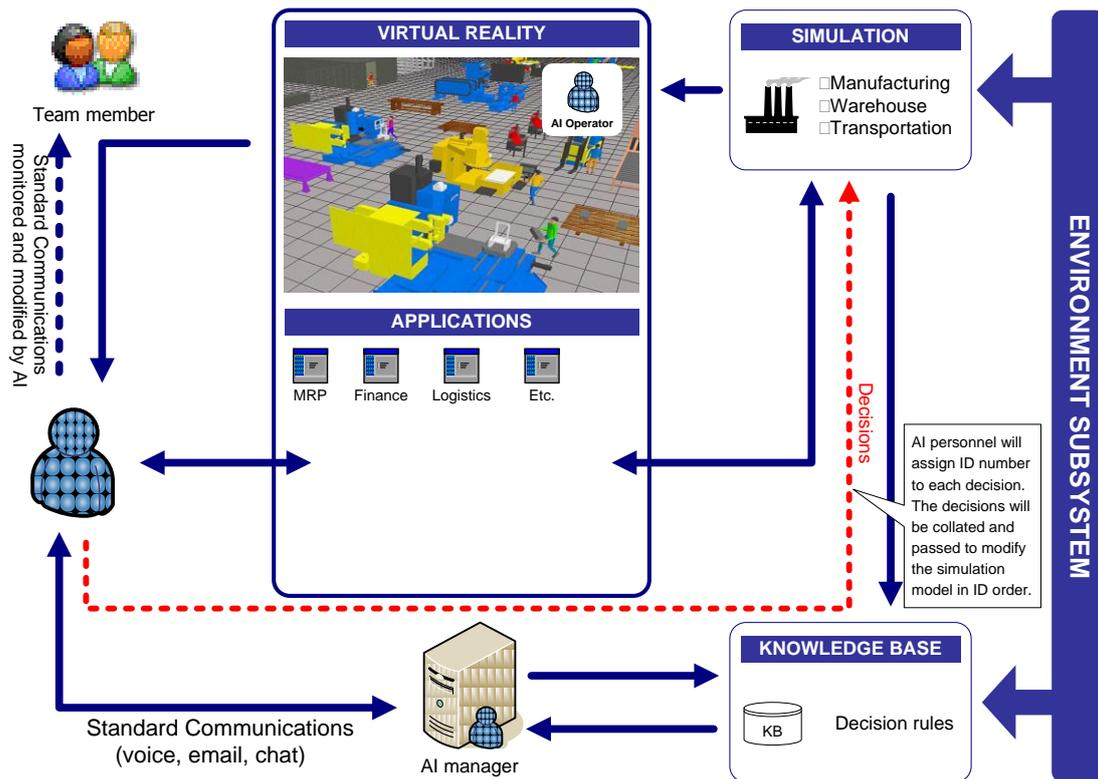
**Figure 7-3: Early technical design of Virtual World prototype**
