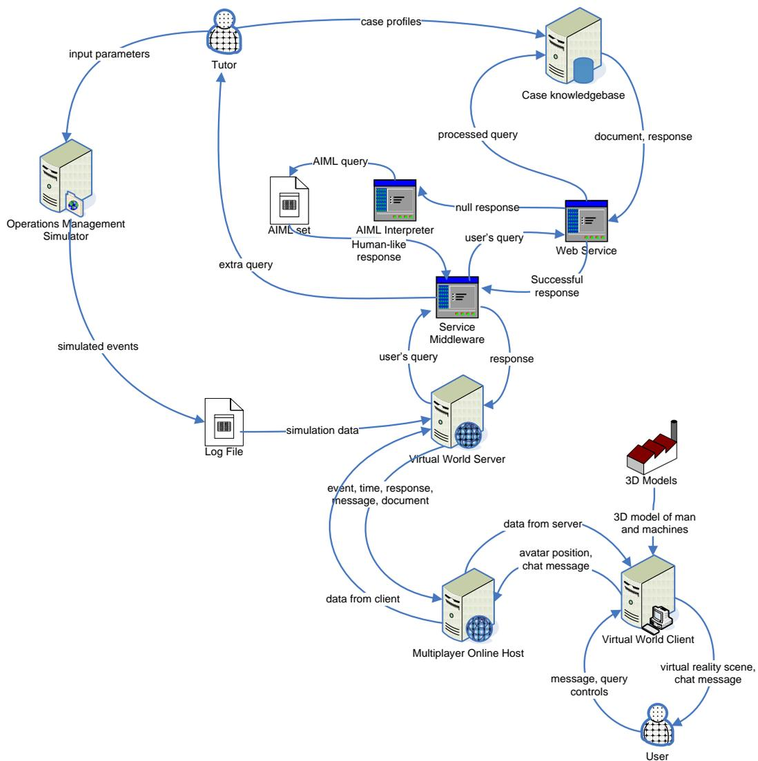
**Figure 8-1: Schematic view of Virtual World prototype's architecture**
