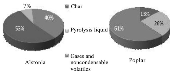
Fig. 1—Product distribution of intermediate pyrolysis (raw material, short-rotation energy crops from a wastewater-irrigated plot of Palwal, Northern India; pyrolysis temperature, 500°C; heating rate, 25°C/min)
