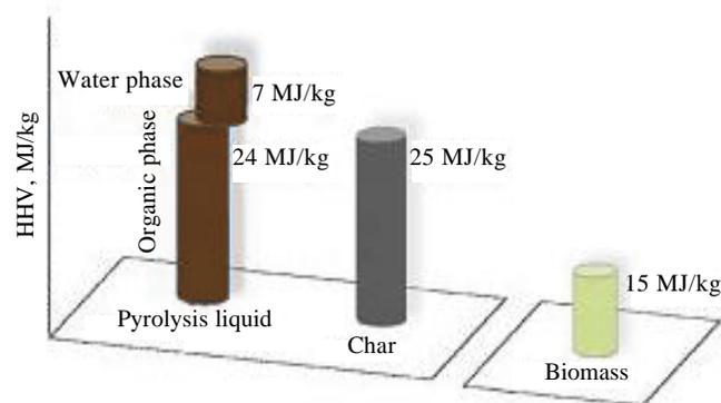
Fig. 2—Energy content of biomass (straw) and its solid and liquid pyrolysis products<sup>73</sup> (raw material, straw pellet; pyrolysis temperature, 500°C; feeding rate, 50 kg/h)
