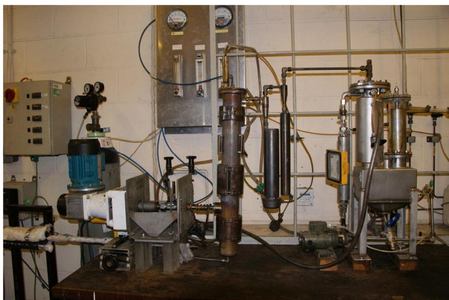
Figure 10-3 Photograph of optimised rig showing alternative feed system and 500g/h reactor
