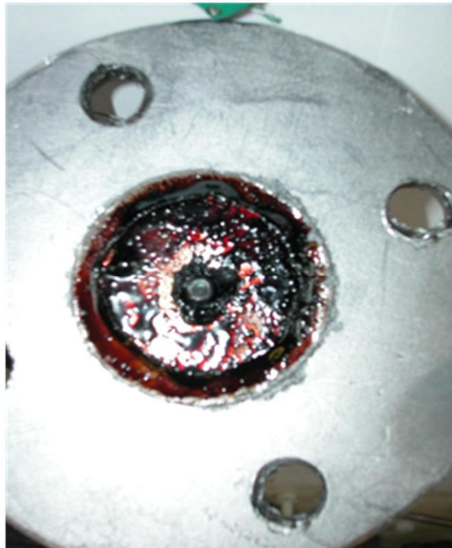
Figure 6-15 Fouling due to inefficient quenching
