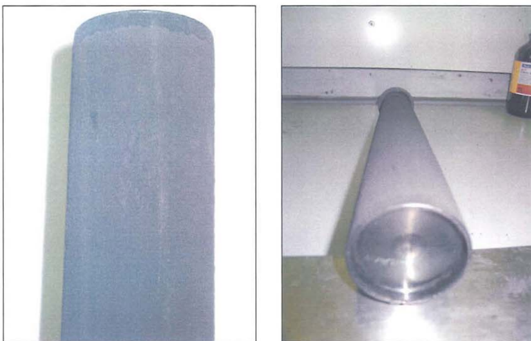
Figure 48: Inconel candle after experiment 191 with precoating prior filtration. The dust cake was removed totally with reverse pulse. Only a thin residual dust layer remained on the candle surface.
