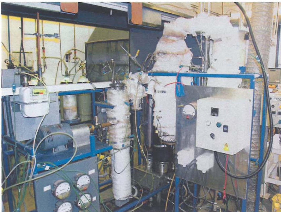
Figure 36: Picture of the experimental set-up showing the 1kg/h fast pyrolysis reactor with filtration unit
