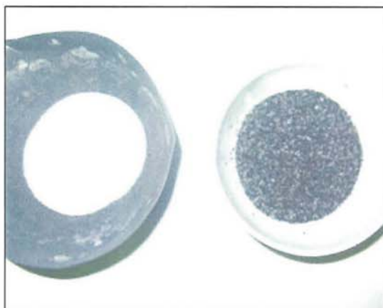
Figure 7: Dolomite before and after use in a fixed bed secondary reactor for catalytic cracking of pyrolysis vapours (Aston University)
