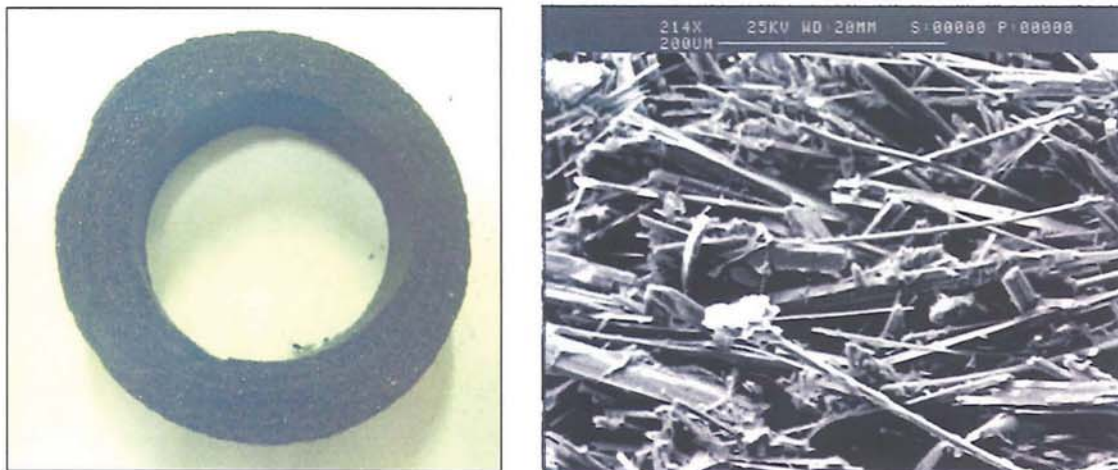
Figure 56: Picture of a slice of used Tenmat candle (left) and SEM-Picture of the same piece (right)
