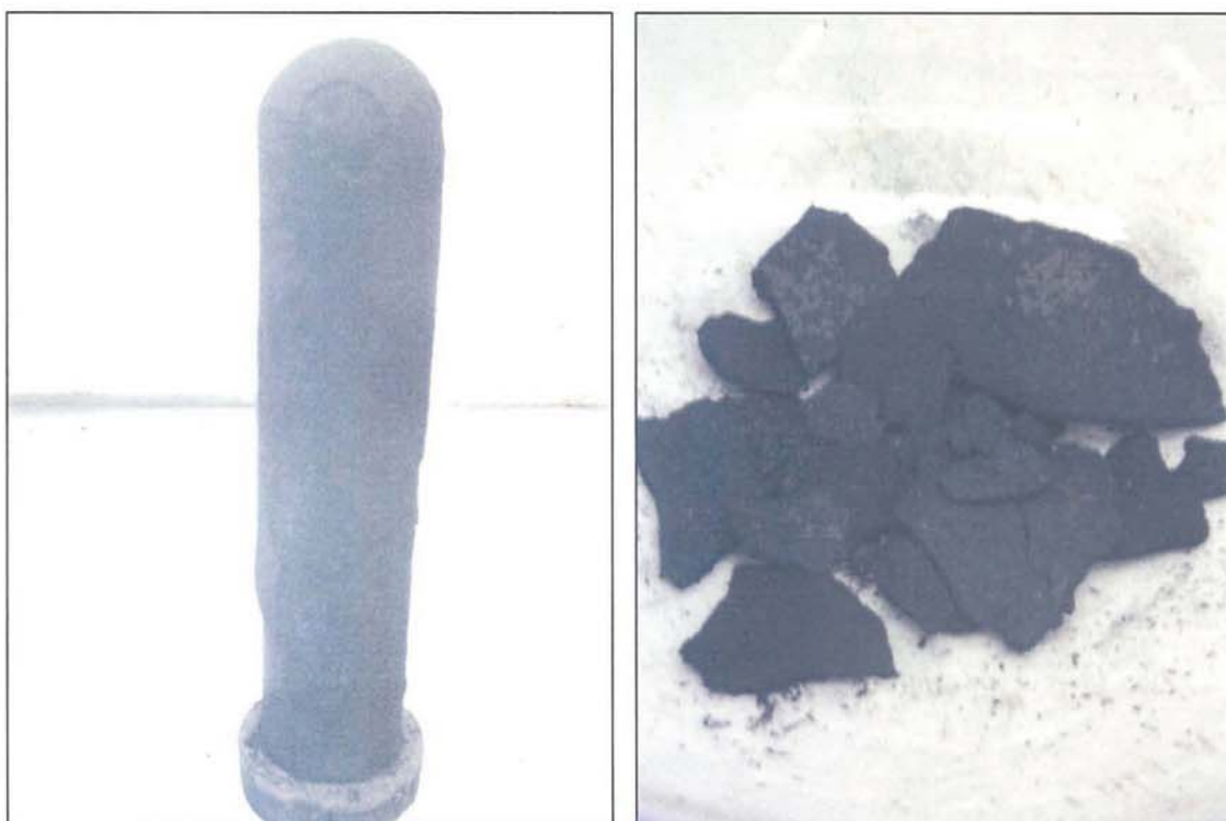
Figure 41: Picture of used Tenmat filter candle (left) and removed patches of filter cake found in the char pot (right) after experiment 161
