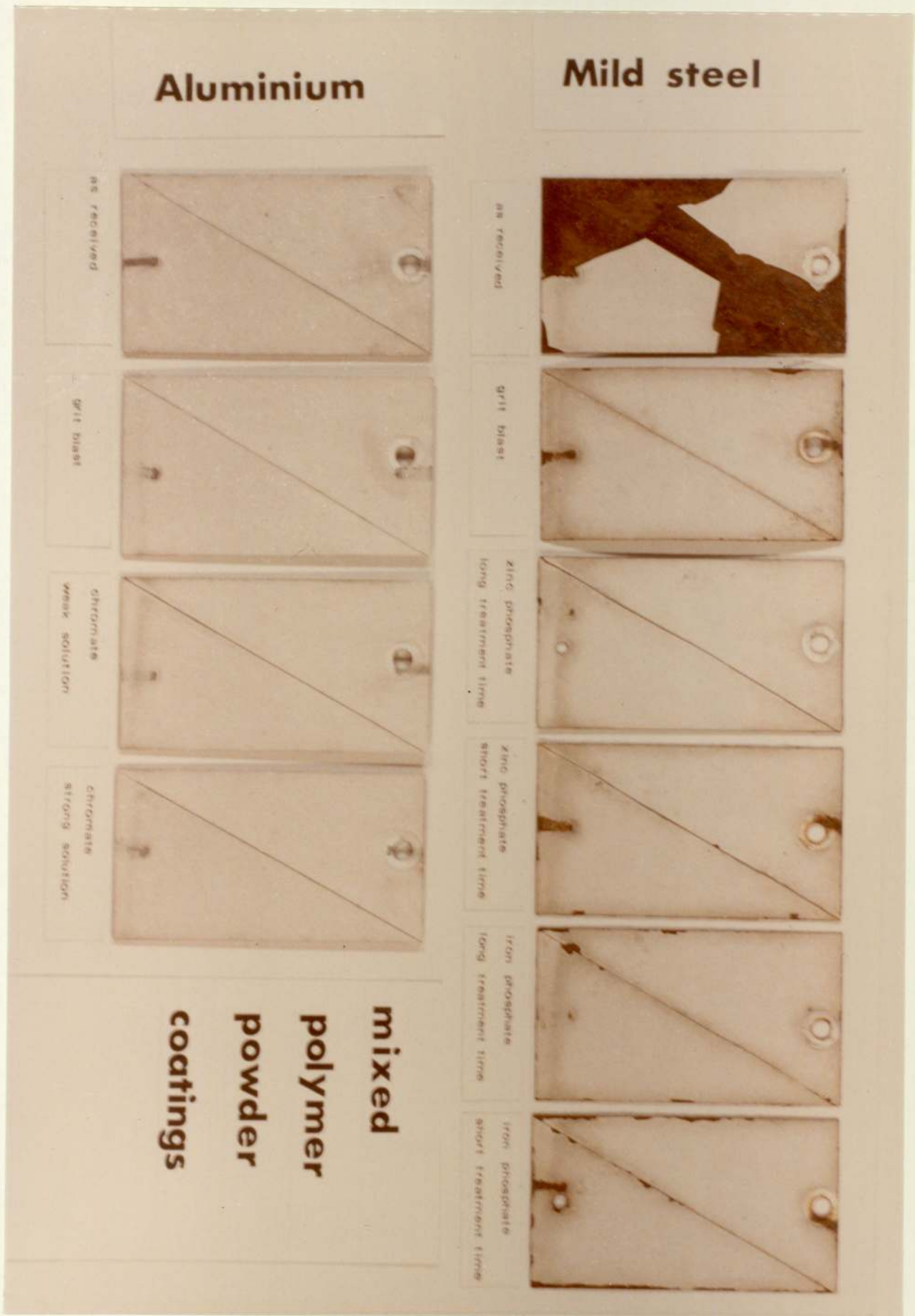
Figure 18 Corrosion panels after static outdoor roof exposure
