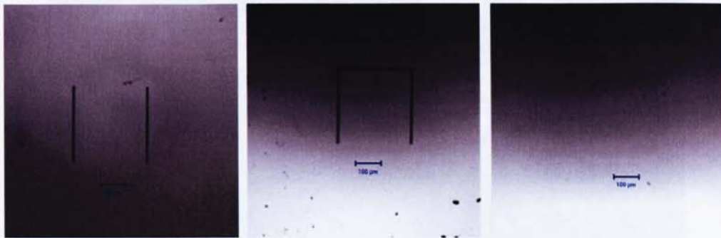
Figure 4.2: LSM images of 300\mu\text{m} microplates (Type C-F-C-F, Type C-F-F-F, Type C-C-C-C)
