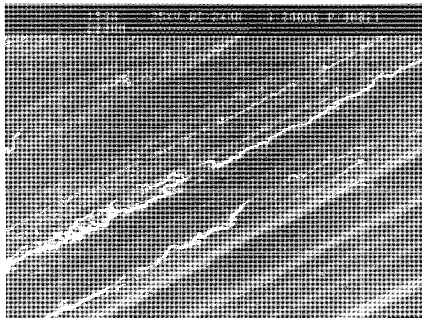
Figure 4.42. SE image of the wear surface of the matrix pin after sliding at 1.0 m/s speed and 60 N load, showing plastic deformation and microchip formation, leading edge to left.
