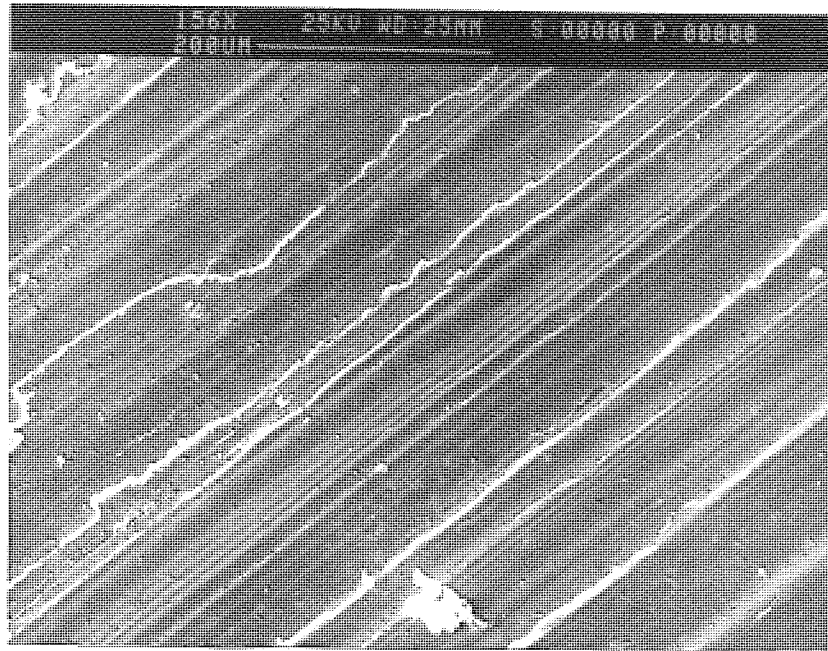
Figure 4.40. SE image of the wear surface of the matrix pin after sliding at 1.0 m/s speed and 24 N load, showing flat ridges deformed metal and grooving at high magnification.
