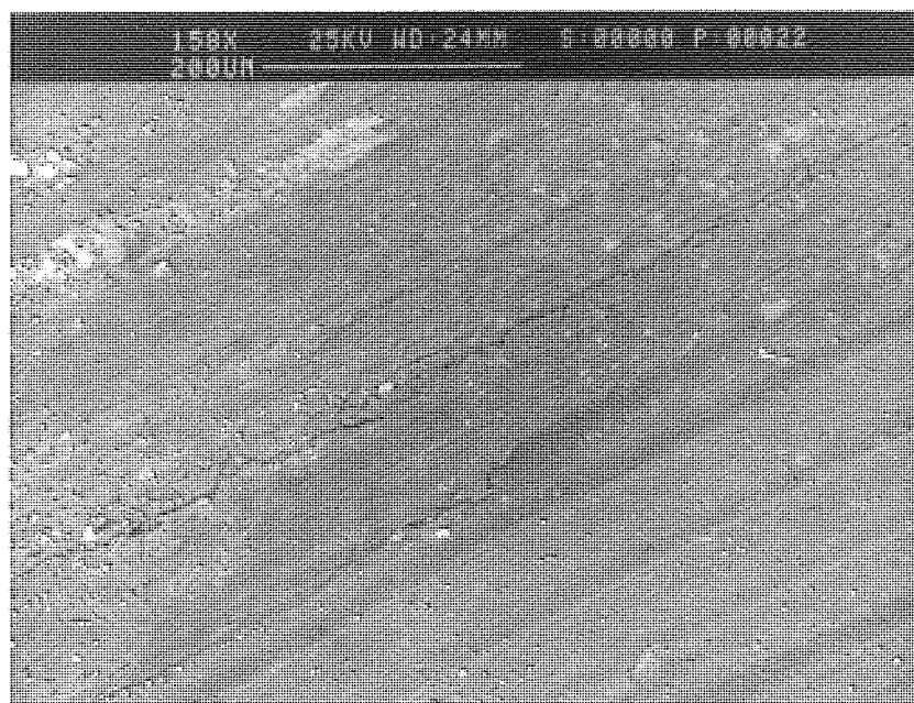
Figure 4.43. BSE image of Figure 42, showing deformed layer and iron transfer to the pin surface.
