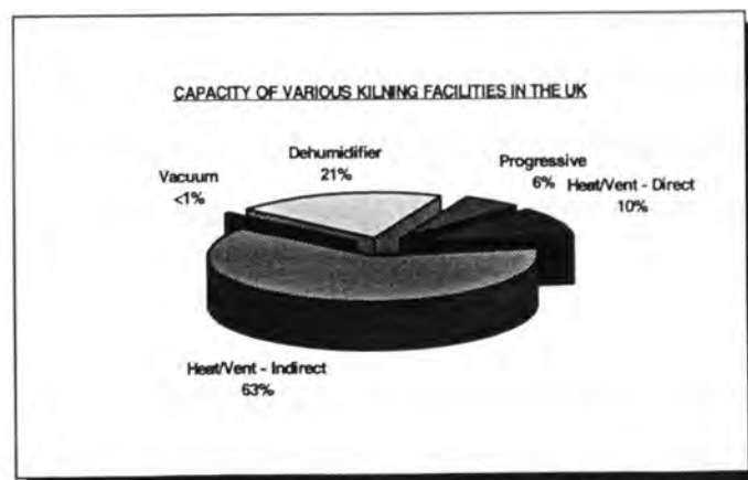
Figure 4 - Proportion of the total capacity for specific kilns types
