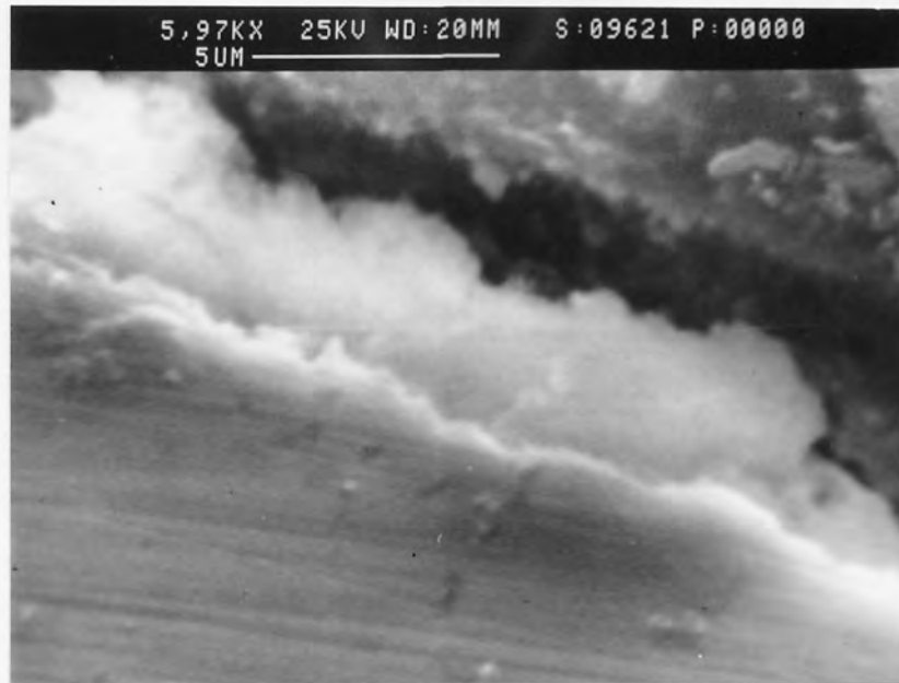
Fig. 96 SEM image of residual lubricant layer: Pressure nozzle semi-angle = 6 degrees; Drawing speed = 47 m/min; Area reduction = 20%; Lubricant: Traxit; Medium carbon steel; Residual lubricant thickness = 5.8 \mu\text{m} .
