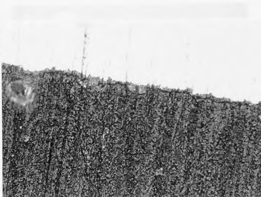
(a) Optical microscope image of an undrawn wire surface (500x)
