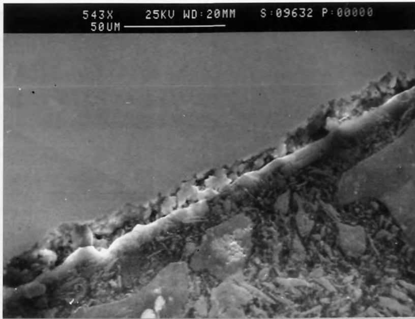
Fig. 99 SEM image of residual lubricant layer: Pressure nozzle semi-angle = 6 degrees; Drawing speed = 20 m/min; Area reduction = 21%; Lubricant: Traxit; Medium carbon steel; Residual lubricant thickness = 9.6 \mu\text{m} .
