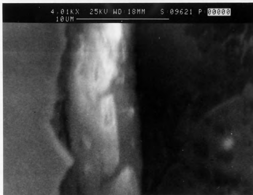
Fig. 102 SEM image of residual lubricant layer: Pressure nozzle semi-angle = 6 degrees; Drawing speed = 47 m/min; Area reduction = 24%; Lubricant: Traxit; Medium carbon steel; Residual lubricant thickness = 7.1 \mu\text{m} .
