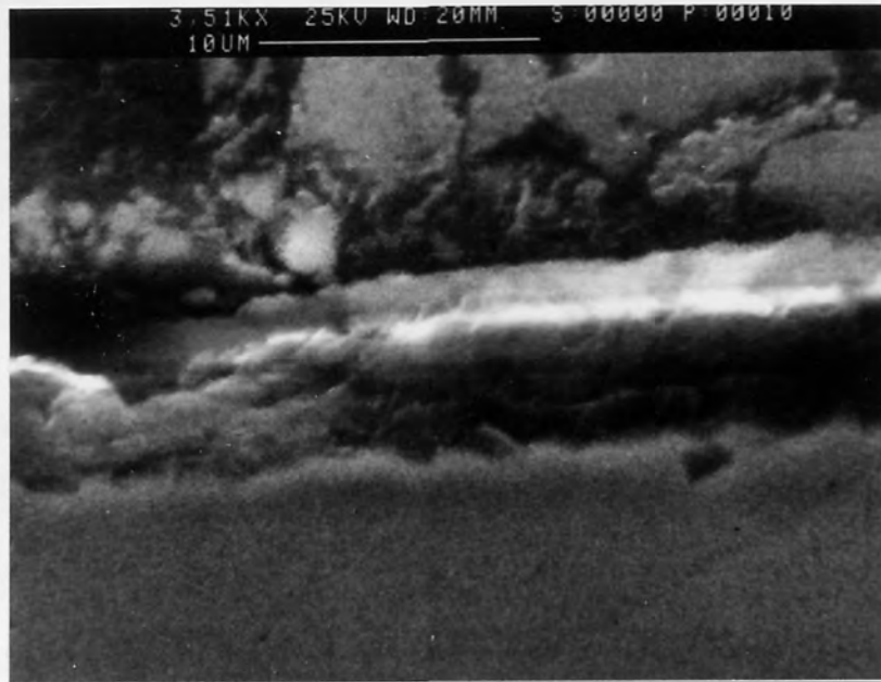
Fig. 93 SEM image of residual lubricant layer: Pressure nozzle semi-angle = 10 degrees; Drawing speed = 27 m/min; Area reduction = 14%; Lubricant: Traxit; Low carbon steel; Residual lubricant thickness = 4.7 \mu\text{m} .
