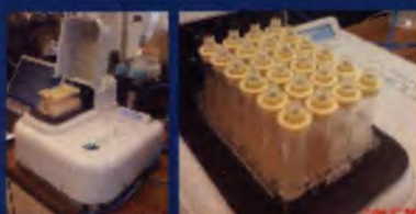
Figure 5. Applikon Micro 24 Bioreactor in use; showing 24 well incubation cassette with S. cerevisiae cultures
