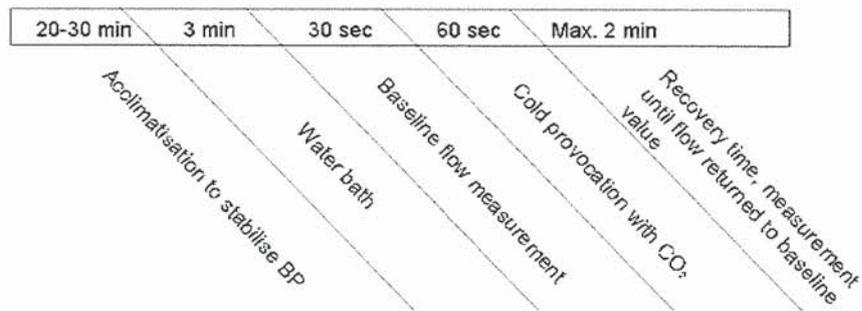
Figure 5.1: Measurement protocol of nail-fold capillary assessment
