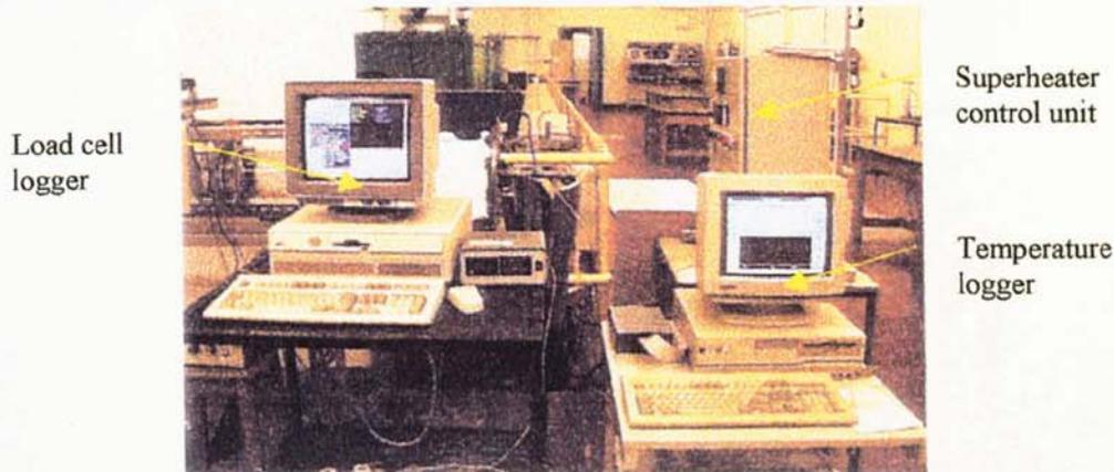
Figure 6.26 Control instrumentation and data logging equipment
