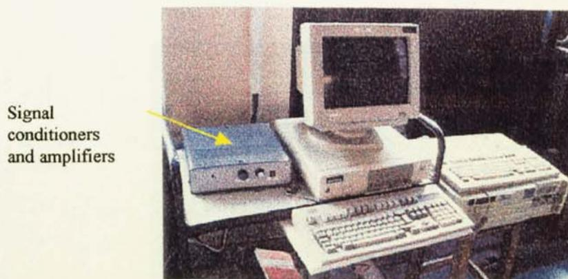
Figure 6.40 Data logging (heat pump dryer)
