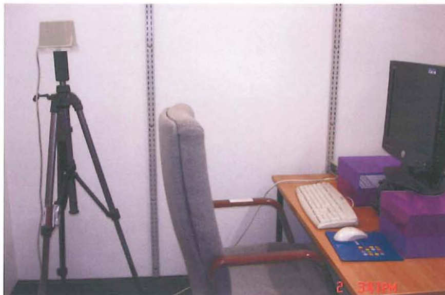
Figure 4.4-4 Set-up of the Eye-Tracking Experiment (participants' side)
