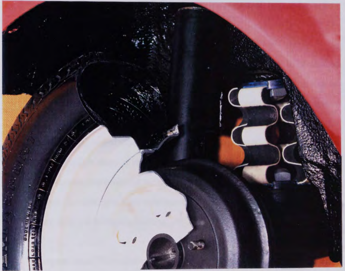
Figure 2.17 Multi-limbed sulcated spring in an automotive suspension application.
