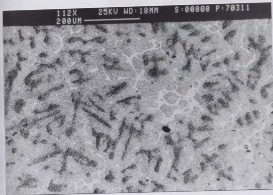
Figure 54. SEM micrograph of ZA-27 taken from a zone near to the chill showing a finer dendritic structure and narrower interdendritic spaces filled with eutectic \eta .
