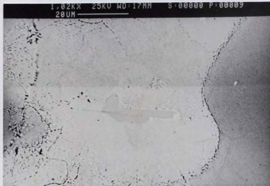
Figure 62. SEM micrograph of Super Cosmal alloy showing the structure of the zinc-rich interdendritic. The irregular particle was identified as T' which is in part surrounded by zinc.
