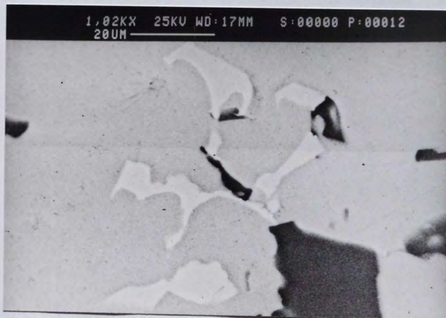
Figure 61. SEM micrograph of Super Cosmal alloy showing particles of clustered \text{CuAl}_2 intermetallics in the Al-rich phase.
