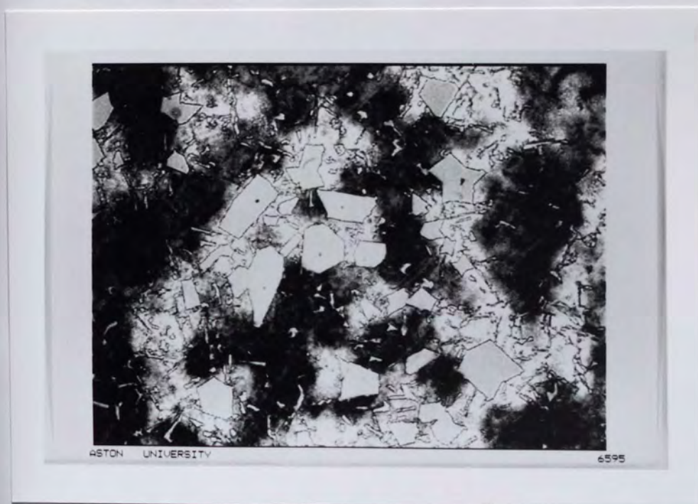
Figure 67. Optical micrograph of HAZCA alloy showing a cluster of large primary silicon particles and eutectic silicon in the Al-rich matrix. x 200.
