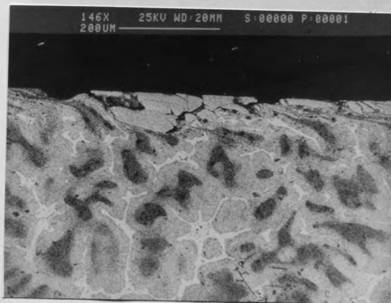
Figure 98. Backscattered electron image of the same sample of Figure 97 showing a section of a thick surface layer where steel fragments are embedded.
