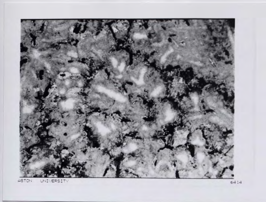
Figure 48. Optical micrograph of ZA-27 alloy from a zone of relatively slow cooling rate showing a coarse dendritic structure of \alpha -cored \beta dendrites with darker eutectic zinc. \times 100 .
