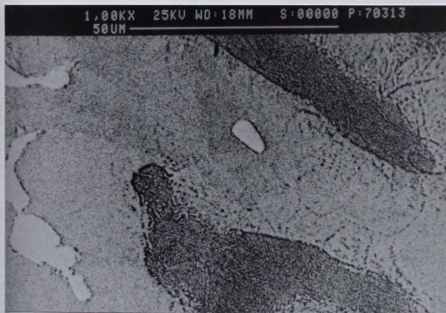
Figure 55. SEM micrograph showing rims of aluminium particles around both the eutectic zinc and the cores of the Al-rich former \alpha' phase. Precipitation of Al particles in sub-grain boundaries.
