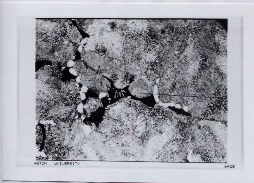
Figure 51. Optical micrograph showing fine decomposition of \alpha' and \beta phases into \alpha and \eta articles. \times 500 .
