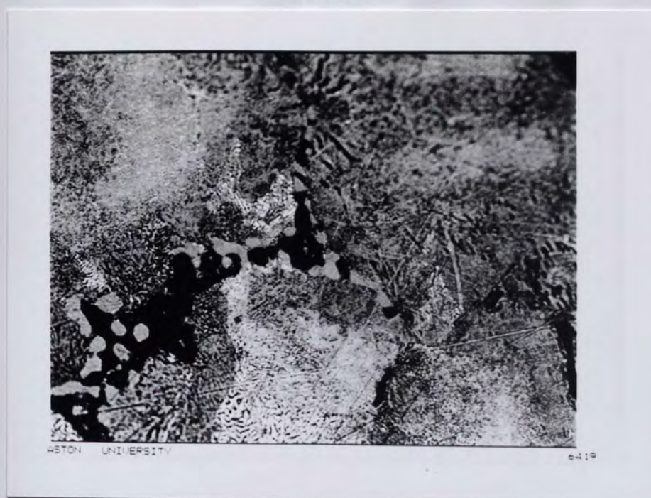
Figure 49. Optical micrograph showing the presence of \epsilon phase as white particles in the interdendritic eutectic and decomposition of former \beta phase into lamellar and particulate structures of \alpha and \eta phases. \times 500 .
