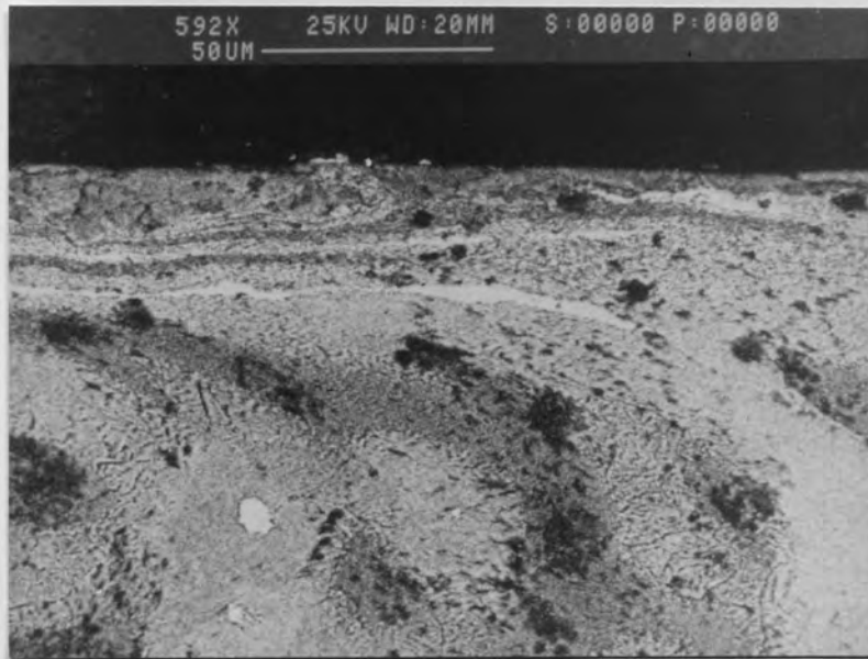
Figure 97. Backscattered electron image of the transverse section of a ZA-27 pin worn at 1 m/s and 15 kgf load. Sliding direction right to left.
