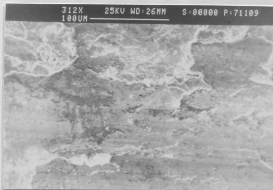
Figure 96. Increased magnification of Figure 95 showing patches of oxide debris adhered to the wearing surface.
