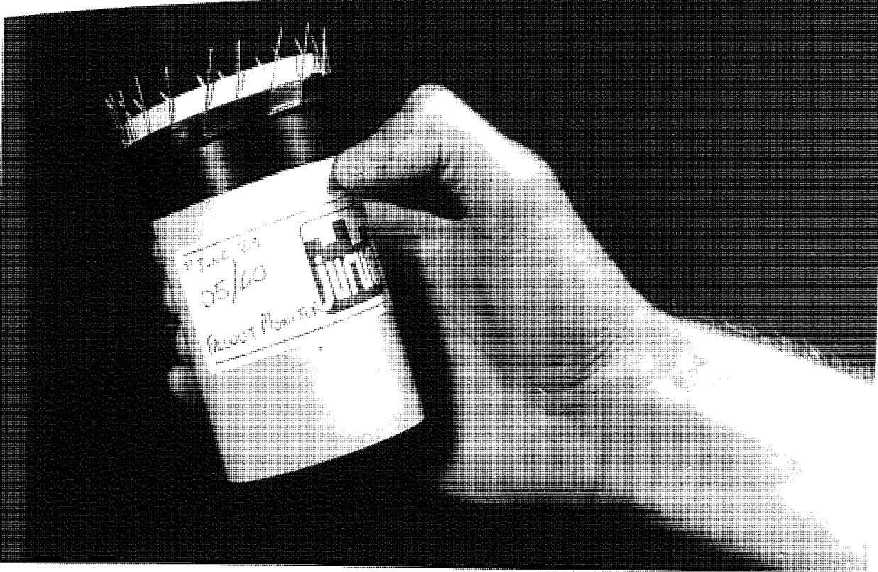
PLATE 6.1: DEPOSIT GAUGE USED IN THE WALSALL STUDY
