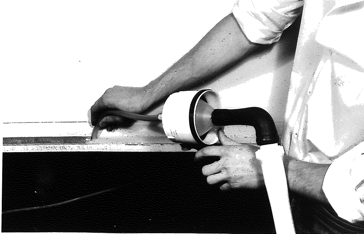
PLATE 6.3: COLLECTION OF SETTLED HOUSE DUST USING A NOVEL FILTER-SUCTION TECHNIQUE
