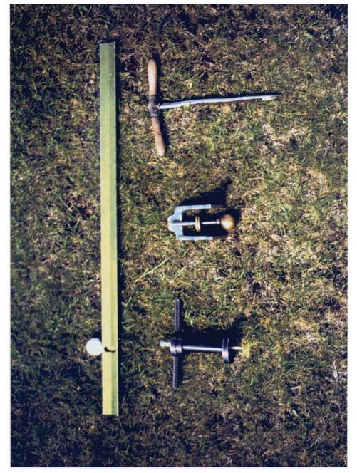
FIGURE 2.15. The Stimpmeter, above, and below, from left to right, the USGA penetrometer, the USGA green hardness tester and the 180mm soil corer.
