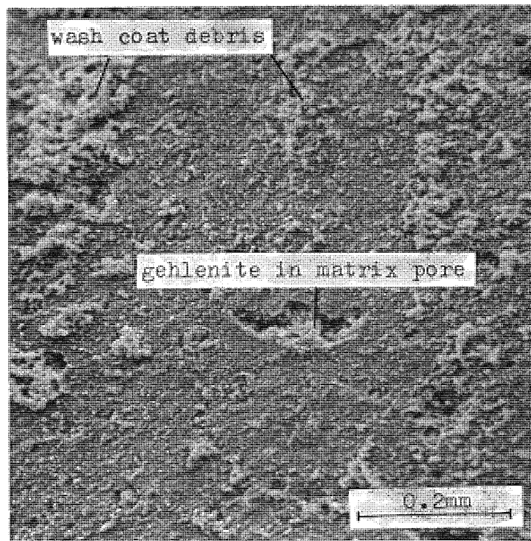
Figure 6.8. : Scanning electron micrograph of catalyst M2 after ageing in an engine dynamometer rig for the equivalent of 5000 miles. The wash-coat has been lost leaving only debris on the surface of the matrix wall
