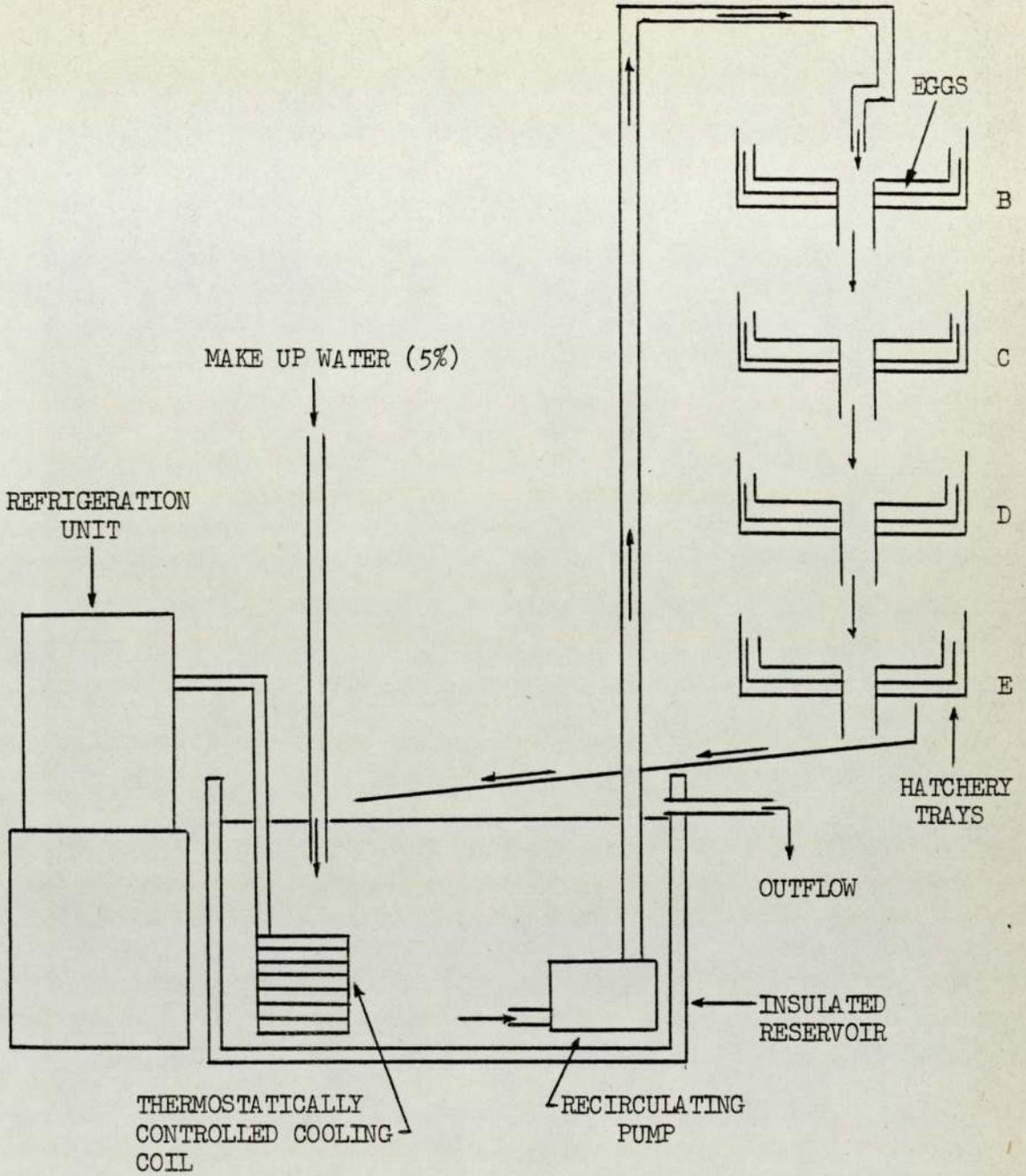
FIG. 5.2. ARRANGEMENT OF THE APPARATUS IN THE COOLED INCUBATION SYSTEM USED TO EXTEND THE HATCHING TIME OF RAINBOW TROUT EGGS.
