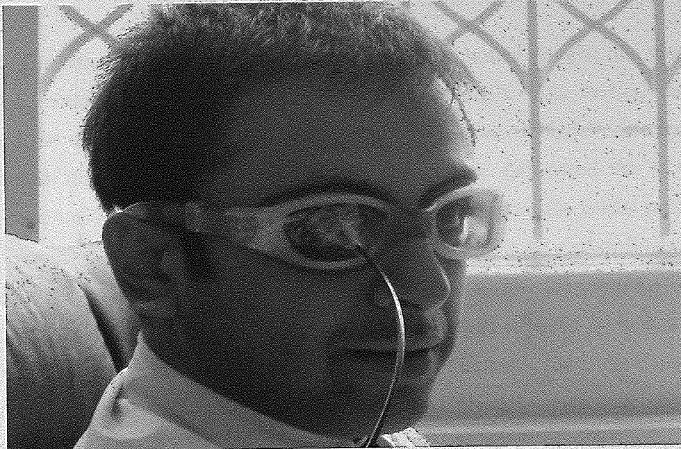
Figure 5.8 The goggle and oxygen sensor in situ on a subject. The black lead is the POF.
