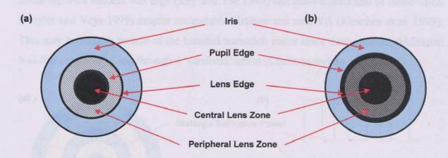
Figure 1.9 Pupil dependency of simultaneous vision contact lenses – produced based on the description in Borish (1988)
