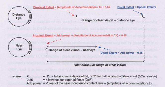
Figure 5.2 The binocular range of clear vision in monovision is governed by the amplitude of accommodation (AoA), depth of focus (DoF) and the contact lens power of the 'near eye'
