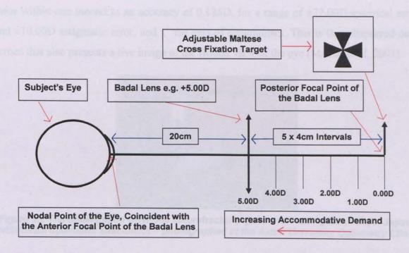
Figure 3.1 Objective measurement of the amplitude of accommodation (AoA) with an optometer and a Badal system – produced based on the equipment shown in Figure 3.2
