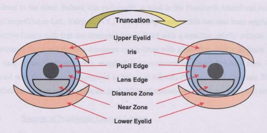
Figure 1.11 Lens truncation creates flat top and bottom edges so that the eyelids can act to prevent lens rotation – produced based on a description in Borish and Soni (1982)
