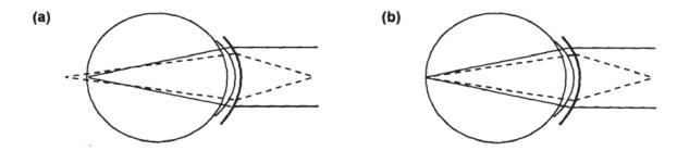
Figure 1.7 (a) A single vision distance contact lens on a presbyopic eye. Distance light (----) is focussed onto the retina but near light (----) is not (b) A simultaneous vision contact lens on a presbyopic eye. Both distance
