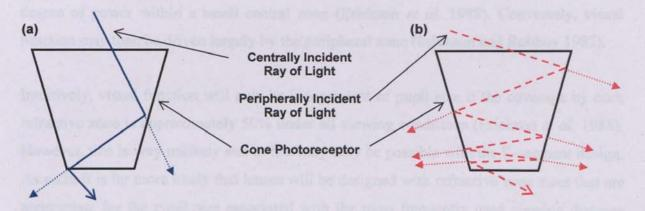
Figure 1.8 The Stiles-Crawford Effect – produced based on the description given above
