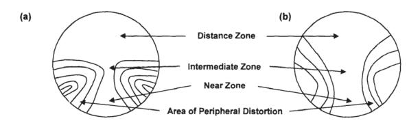
Figure 1.5 Astigmatism plots displaying the type of progression expected of (a) Varilux 1 lens and (b) Varilux 2 lens – reproduced and modified from Meister and Fisher (2008)
