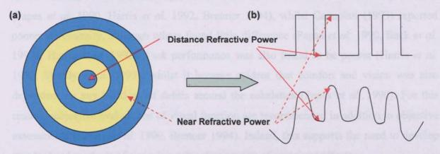
Figure 1.10 (a) Design of the Acuvue™ bifocal contact lens, and (b) the intended (top) and actual (bottom) power profiles – produced based on a figure in Hough (2002)
