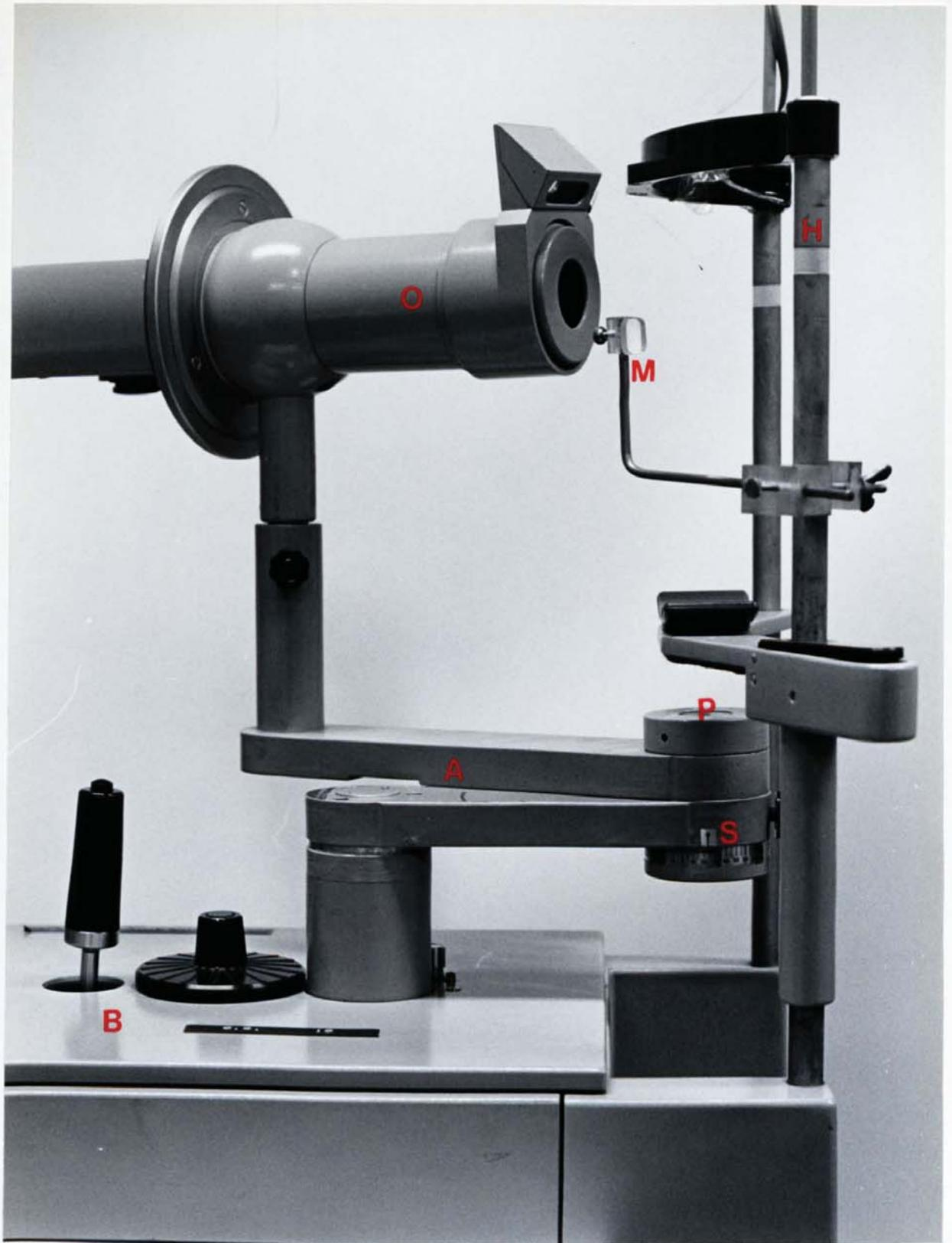
**Fig. 3.3** Photograph of the modified arm built for the Hartinger coincidence optometer. Key: *O* -optometer; *A* -modified arm; *P* -point of rotation; *B* -moveable base; *S* -scale; *H* -headrest; *M* -mirror. See text.
