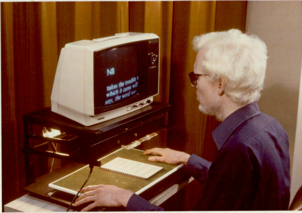
Fig. B.3 Experimental CCTV Magnifier used in Reversed-contrast mode, showing improved X-Y Platform.
