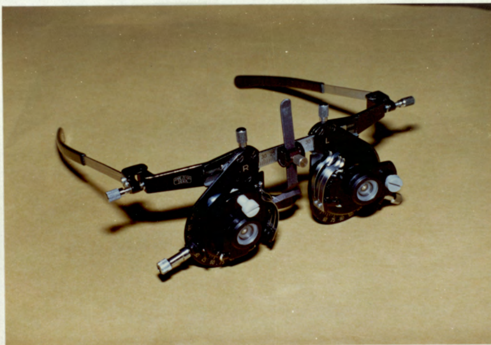
Fig. 9.5 Experimental Binocular Field Expander fitted to Trial-Frame.
