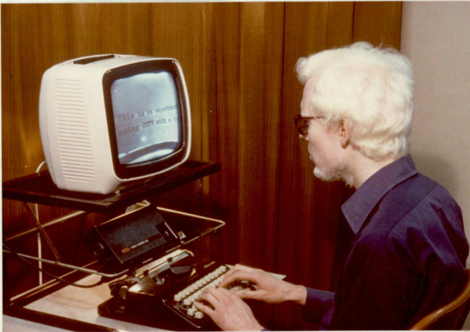
Fig. B.4 Experimental CCTV Model with simple Focussing/Tilt Mechanism designed for Typing.
