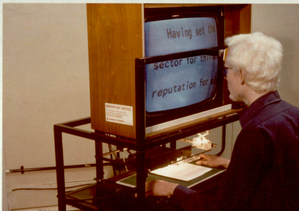
Fig. 8.1 60 cm. CCTV Apparatus for Assessment of Effect of Magnification and Field on Reading.
