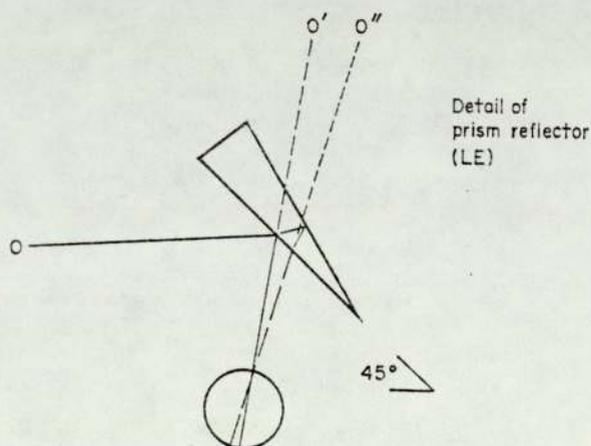
Fig. 11 The method of displacing secondary reflections is shown above.
