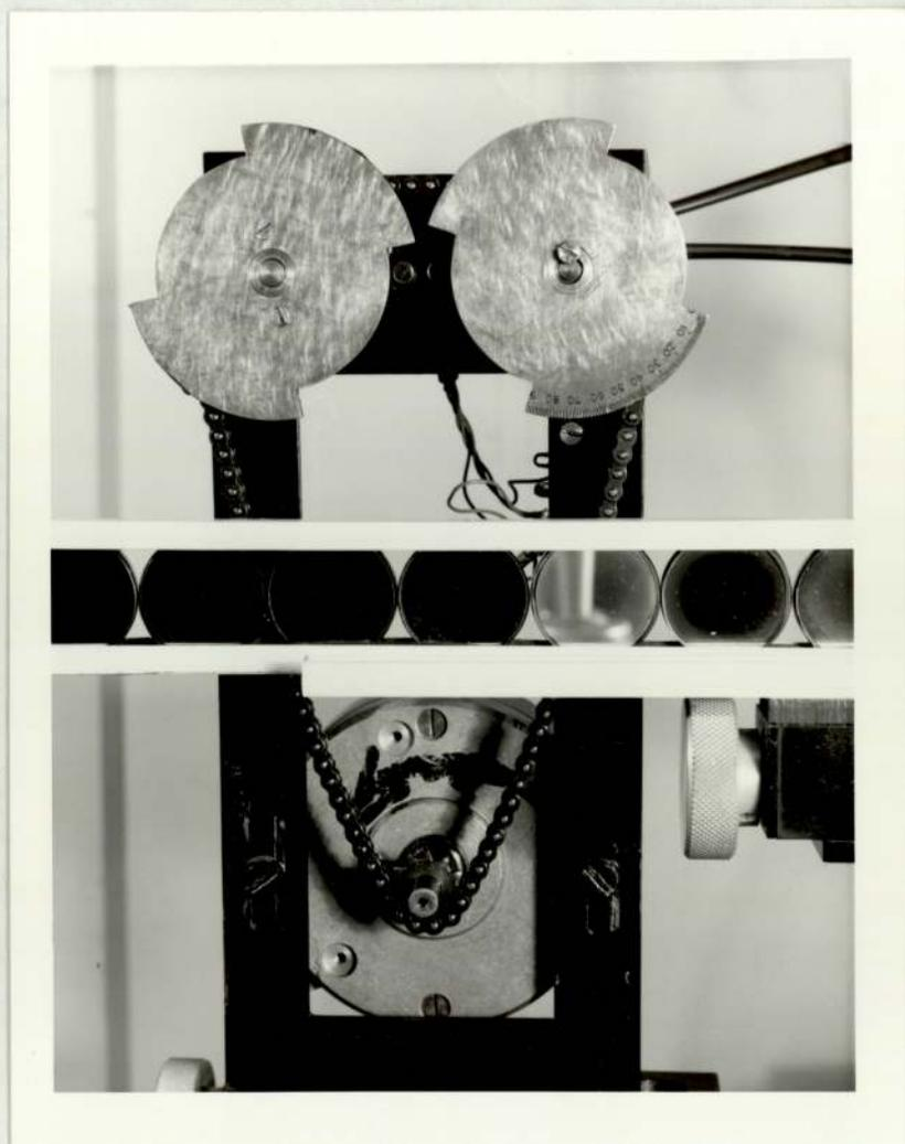
Fig. 13 The sector discs used on the apparatus and their chain drive are shown above. The ends of the two fibre optic bundles are seen behind the sector discs. The interference filters in their rack may also be seen.
