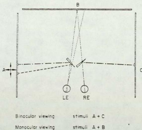
Fig. 10 The method by which the stimuli were presented to the observer is shown above. Stimuli A and B were seen by the left eye. Stimulus C consisted of a fixation spot.
