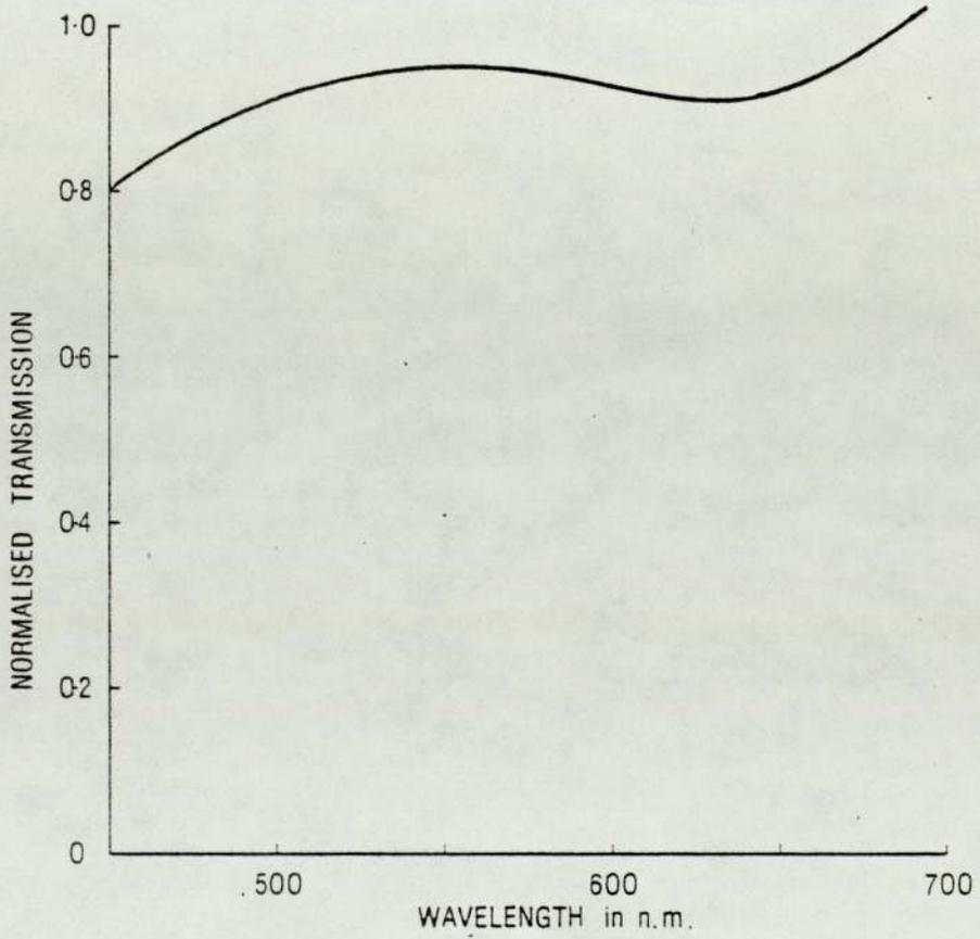
Fig. 14 Spectral transmission curve for 1m. long fibre optic light guide (Rank Optics Technical Publication).
