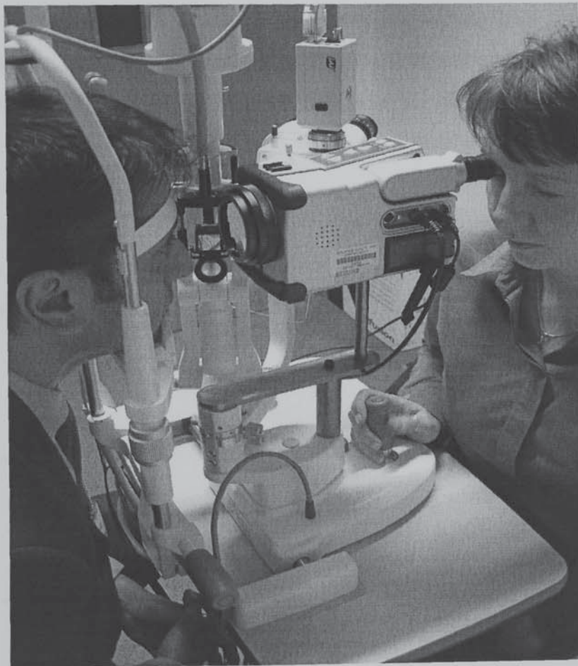
Figure 2.2 Thermo-camera mounted on slit lamp base
