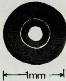
The tip of a Meinhard showing the narrow (10-35 \mu m) annular gap for the gas flow.
