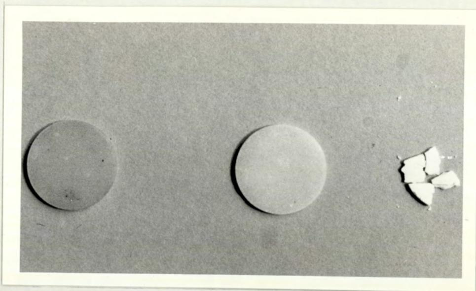
Plate 3.1 Melt Pressed 300PHB (20%PHV) Discs: Undegraded (Left);
