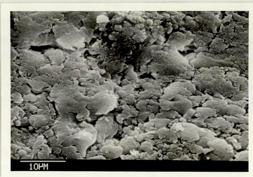
Plate 6.4 SEM of the surface of a non-dissolved 350PHB (12%PHV) / FITC40 Tablet containing 7.5% MCC (X 2000)
