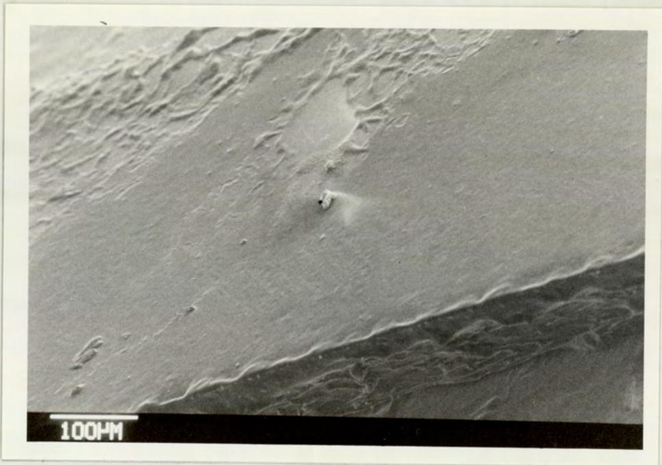
Plate 4.6 SEM (X 200) of an Undegraded 300PHB (20%PHV) Solvent Cast Film
