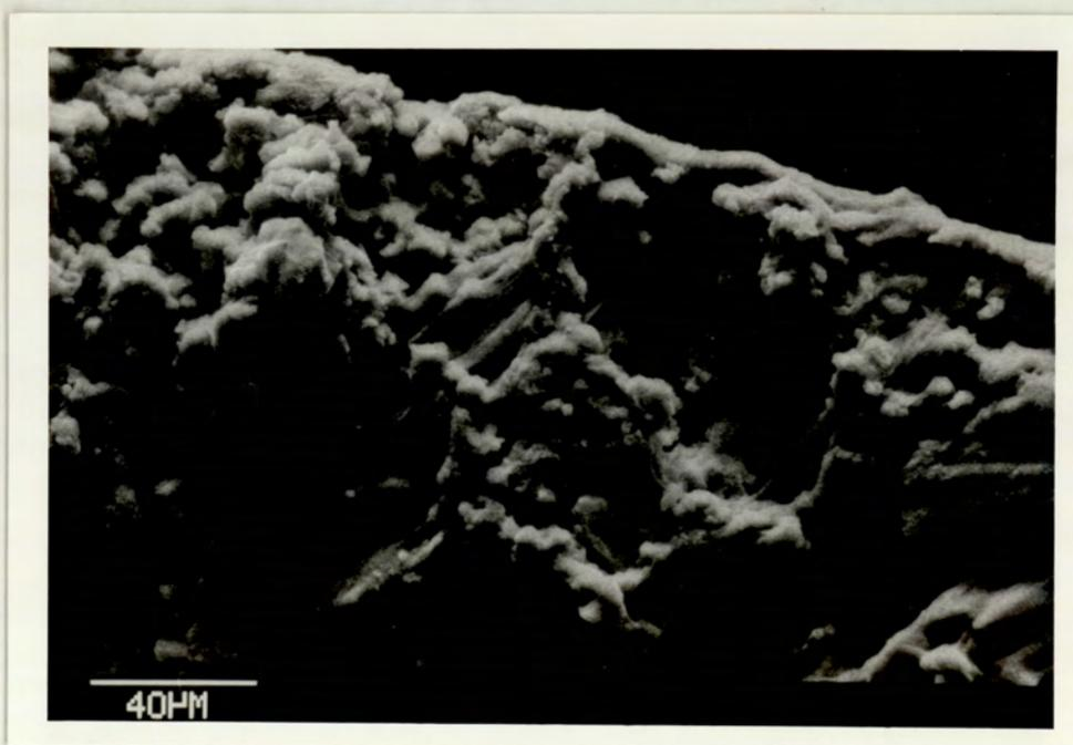
Plate 6.6 SEM of the cross section of a USP dissolved 300PHB (20%PHV) / FITC40 Tablet containing 7.5% MCC (X 500)
