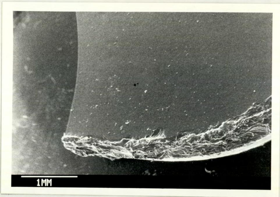
Plate 4.5 SEM (X 20) of an Undegraded 350PHB (12%PHV) Melt Pressed Disc
