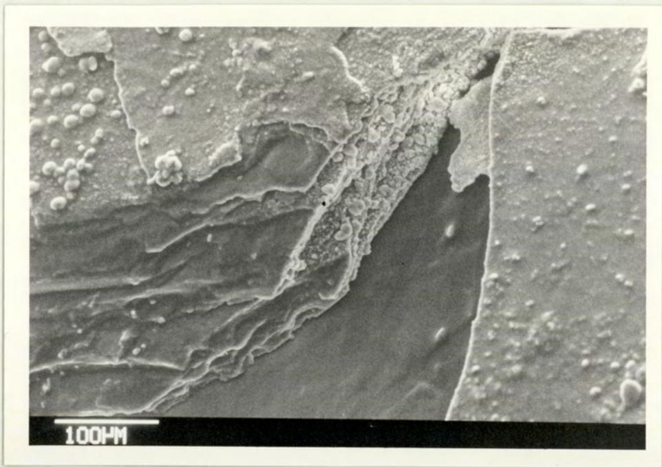
Plate 4.7 SEM (X 200) of a degraded 750PHB (10%PHV) Solvent Cast Film (pH 7.4 buffer at 70°C for 2760 Hours, 66% Weight Loss)
