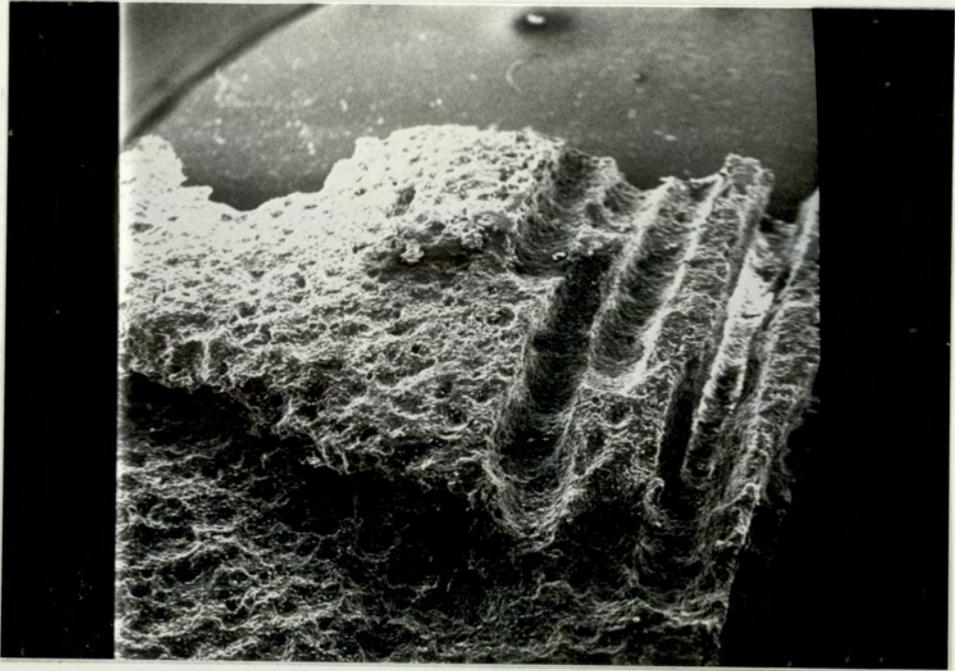
Plate 4.1 SEM (X 22) of a degraded 350PHB (12%PHV) Melt Pressed Disc (pH 10.6 buffer at 70°C for 1385 Hours, 60% Weight Loss)
