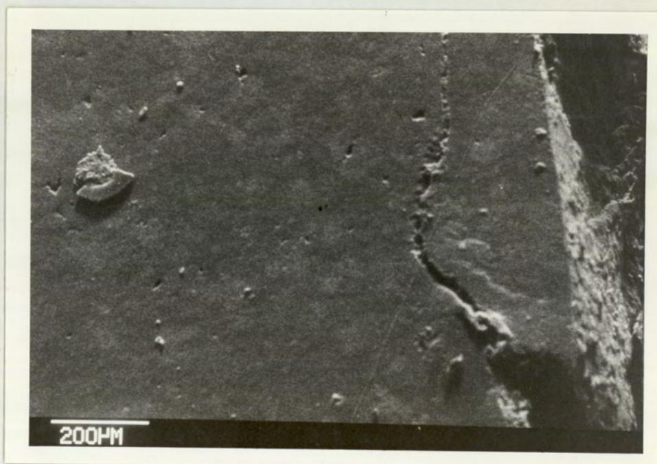
Plate 4.4 SEM (X 100) of an Undegraded 300PHB (20%PHV) Melt Pressed Disc
