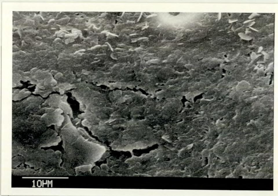
Plate 6.3 SEM of the surface of a USP dissolved 350PHB (12%PHV) / FITC40 Tablet containing 7.5% MCC (X 2000)
