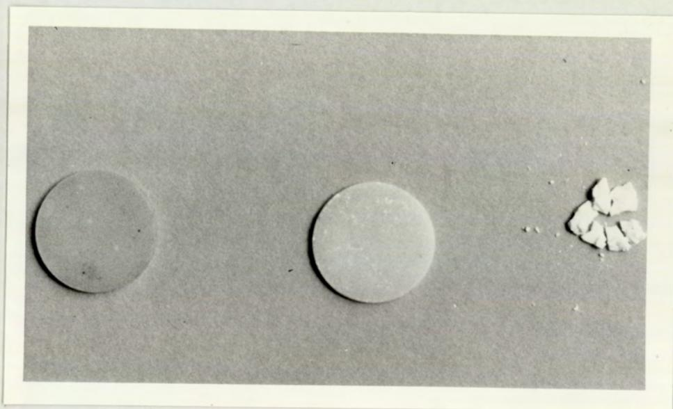
Plate 3.2 Melt Pressed 350PHB (12%PHV) Discs: Undegraded (Left);
