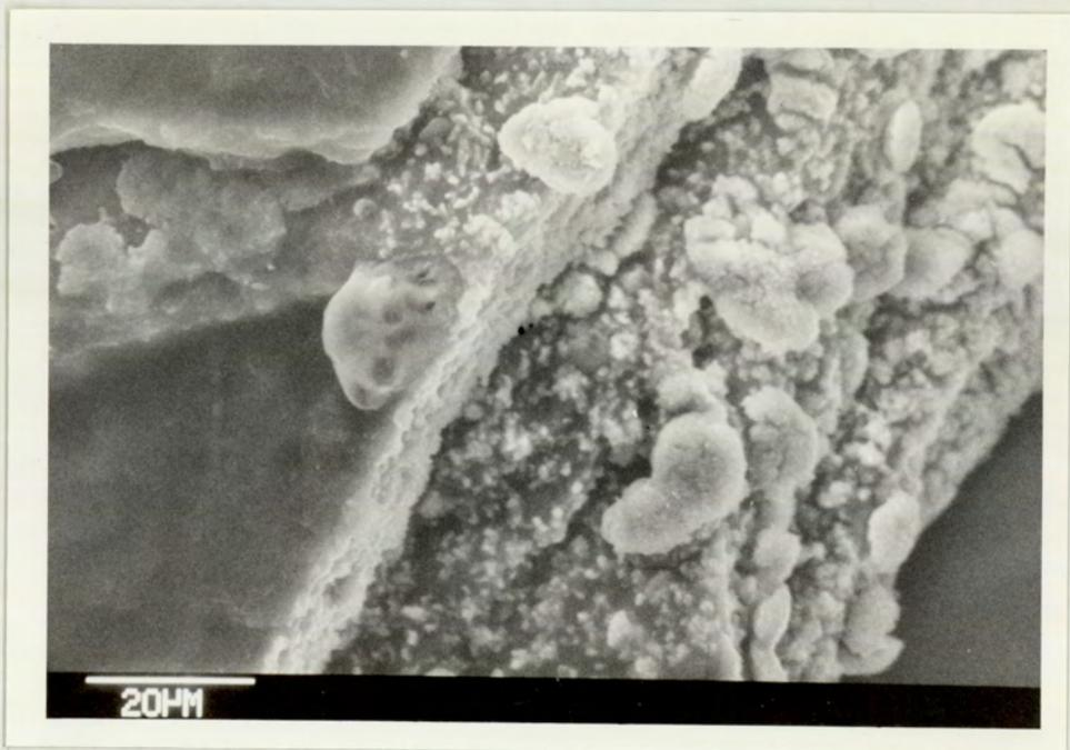
Plate 4.8 SEM (X 1000) of a degraded 750PHB (10%PHV) Solvent Cast Film (pH 7.4 buffer at 70°C for 2760 Hours, 66% Weight Loss) Showing the calcium phosphate surface deposits
