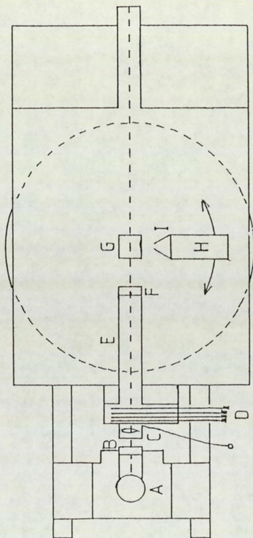
A = Mercury vapour lamp; B = Wavelength filter; C = Shutter unit; D = Series of neutral filters; E = Collimating tube; F = Polariser and variable slit aperture; G = Mounted specimen; H = PhotoceII; I = PhotoceII analyser and variable slit aperture
