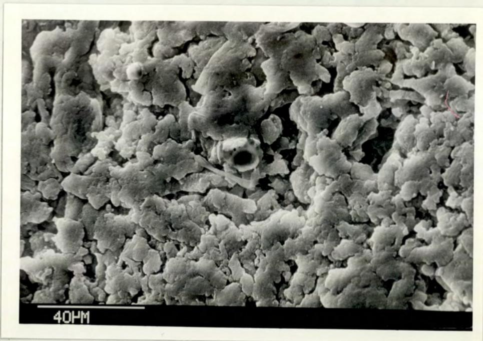
Plate 6.1 SEM of the surface of a USP dissolved 300PHB (20%PHV) / FITC40 Tablet containing 7.5% MCC (X 500)
