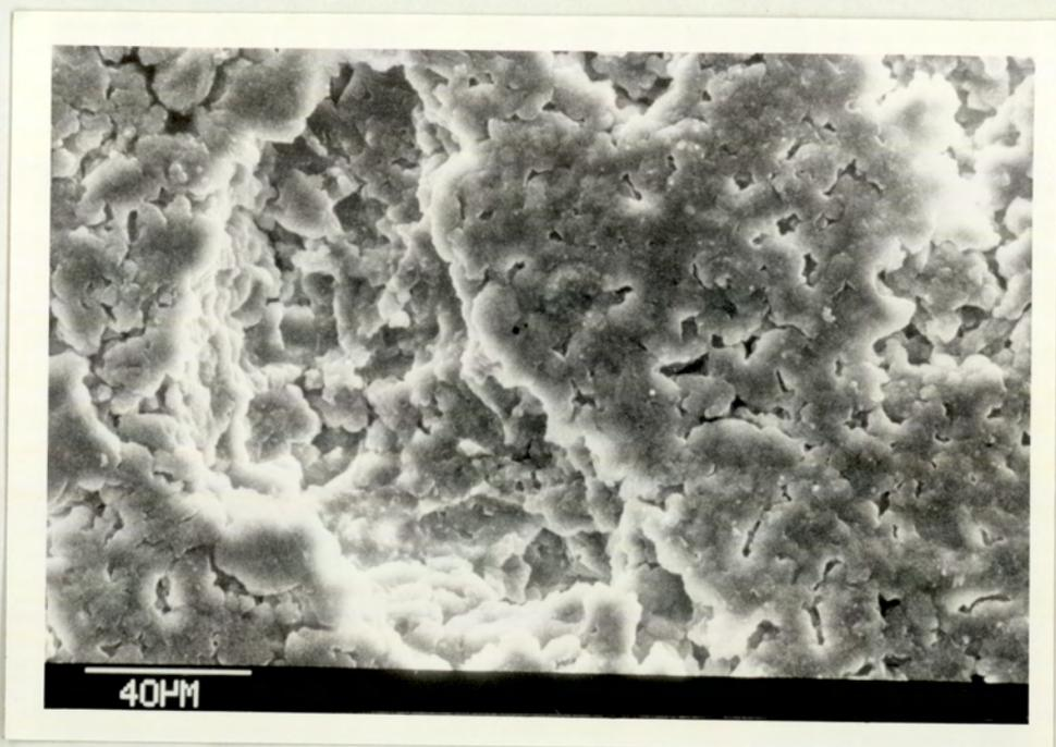
Plate 6.7 SEM of the surface of a USP dissolved 300PHB (20%PHV) /
