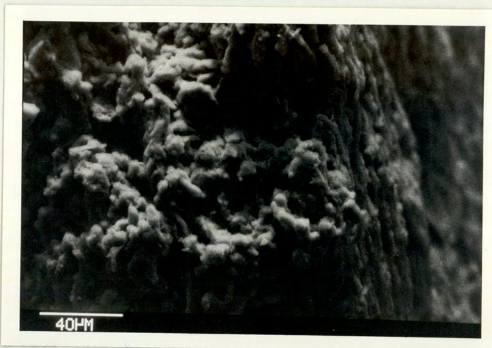
Plate 6.5 SEM of the cross section of a non-dissolved 300PHB (20%PHV) / FITC40 Tablet containing 7.5% MCC (X 500)
