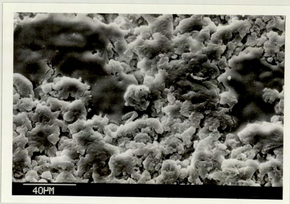
Plate 6.2 SEM of the surface of a non-dissolved 300PHB (20%PHV) / FITC40 Tablet containing 7.5% MCC (X 500)
