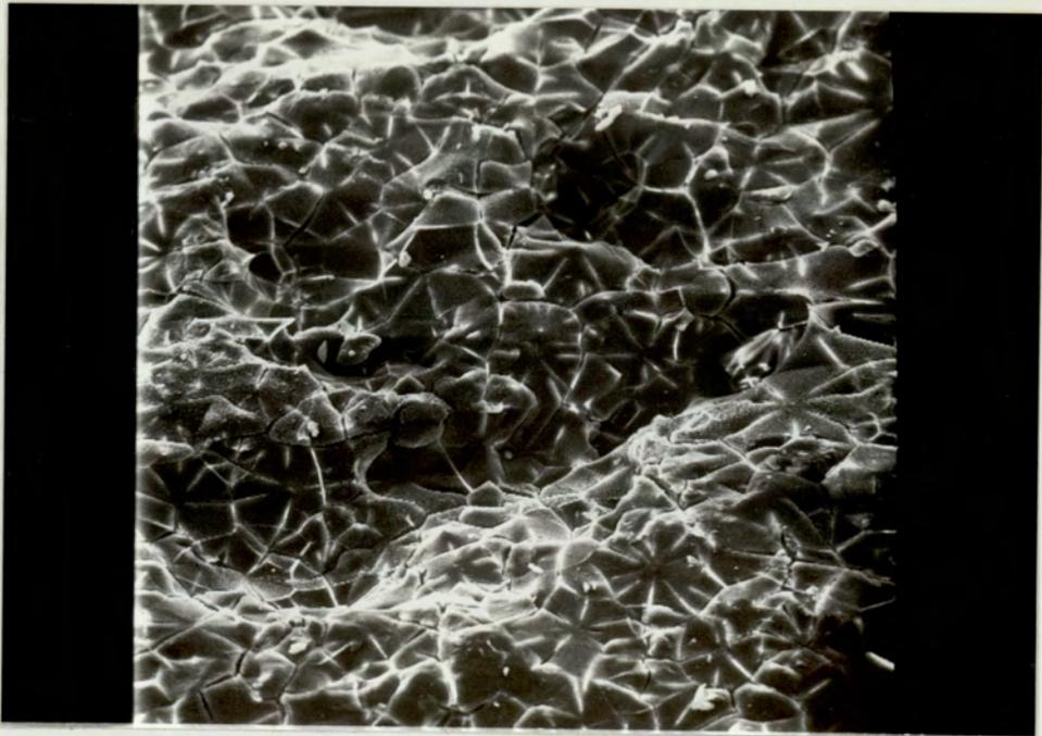
Plate 4.2 SEM (X 222) of a degraded 350PHB (12%PHV) Melt Pressed Disc (pH 10.6 buffer at 70°C for 1385 Hours, 60% Weight Loss)
