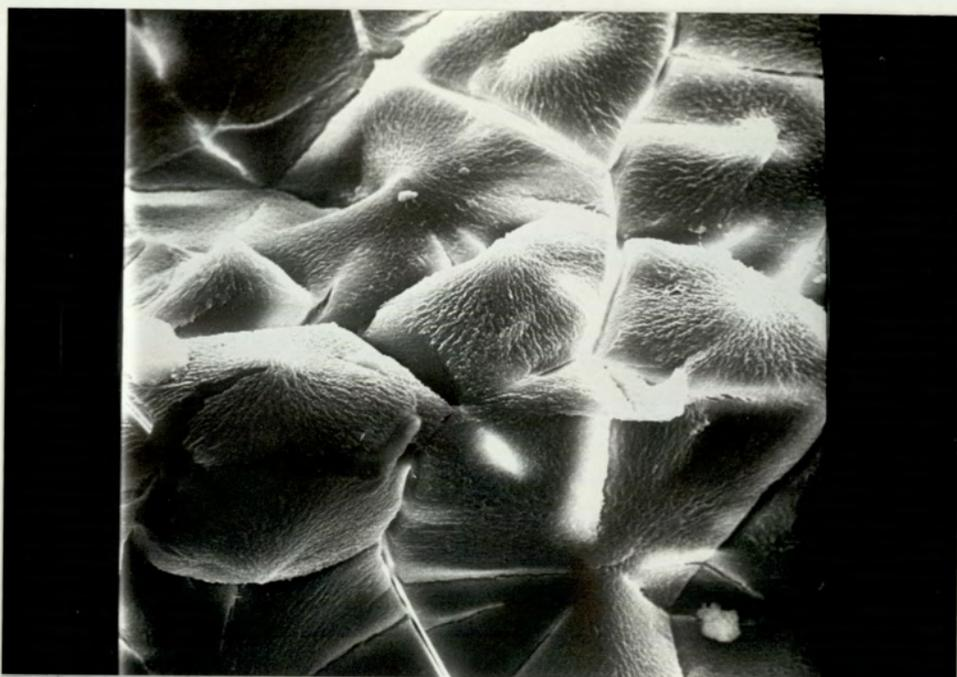
Plate 4.3 SEM (X 1120) of a degraded 350PHB (12%PHV) Melt Pressed Disc (pH 10.6 buffer at 70°C for 1385 Hours. 60% Weight Loss)
