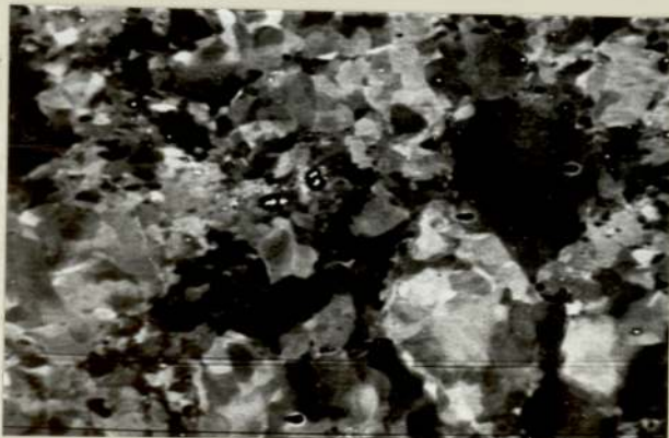
PHOTO. 6.13 C-Mn-Nb STEEL DEFORMED BY 1 REVOLUTION AT 740°C AND AIR-COOLED (MAGNIFICATION x 1000)
