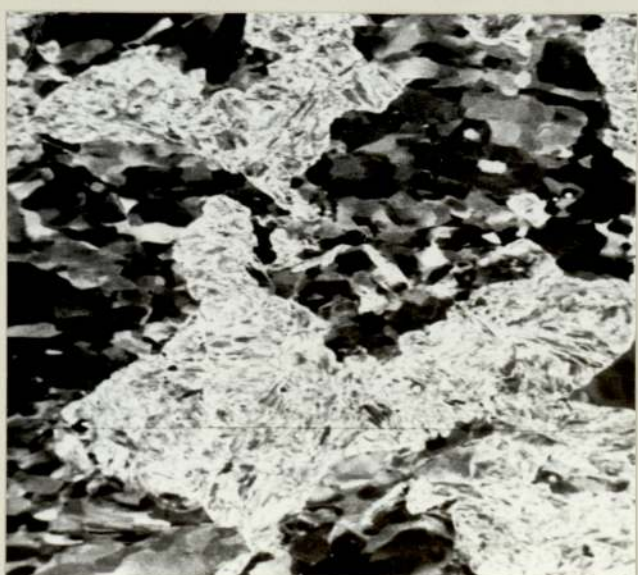
PHOTO. 6.10 C-Mn-V STEEL DEFORMED BY 1 REVOLUTION AT 740°C AND WATER SPRAYED (MAGNIFICATION x 1000)
