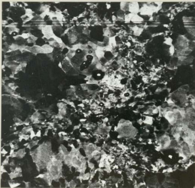
PHOTO. 6.5 C-Mn STEEL DEFORMED 1 REVOLUTION AT 740°C AND AIR-COOLED (MAGNIFICATION x 1000)
