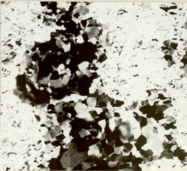
PHOTO. 6.12 C-Mn-V STEEL DEFORMED BY 4 REVOLUTIONS AT 755°C AND WATER SPRAYED (MAGNIFICATION \times 1000 )
