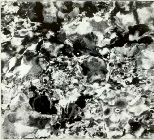
(a) Niobium steel - magnification x 1000
