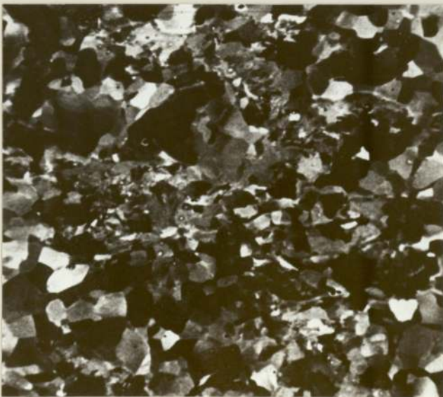
PHOTO 6.7 C-Mn STEEL DEFORMED BY 4 REVOLUTIONS AT 740°C AND AIR-COOLED (MAGNIFICATION x 1000)
