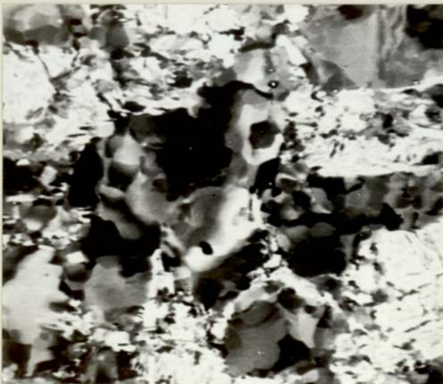
PHOTO. 6.6 C-Mn STEEL DEFORMED 1 REVOLUTION AT 740°C AND WATER SPRAYED (MAGNIFICATION x 1000)
