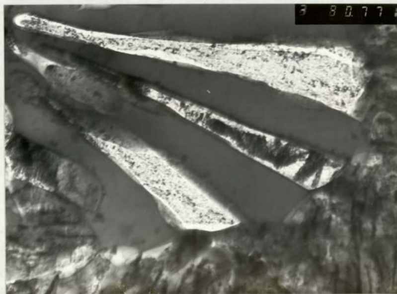
Fig. 123 Transmission electron micrograph of alloy AlZn60Cu3Si2 aged at 100°C for 48 hrs. x42.4K
