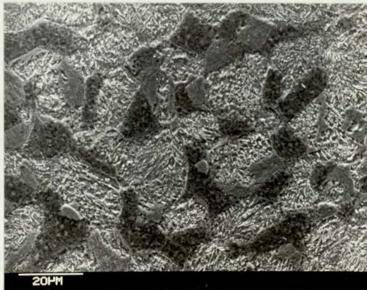
Fig.48 Scanning electron micrograph for alloy ZnAlCuSi, ZnAlCuSi5 at 300°C.
