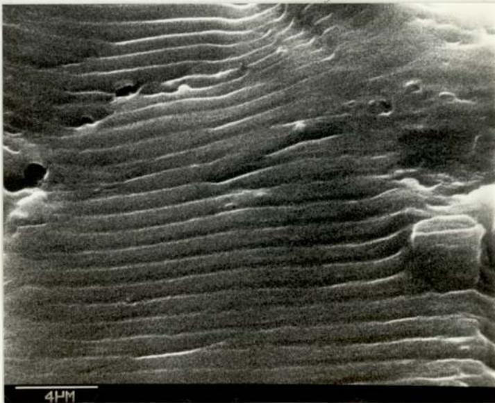
Plate 9.47 SEM fractograph taken from a site 9.39mm from the notch root, 55° correction.
