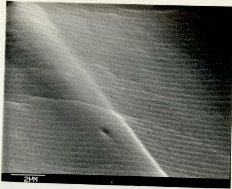
Plate 9.56 SEM fractograph taken from the site 0.05mm after the overloads, which is marked with the letter d in Plate 9.52
