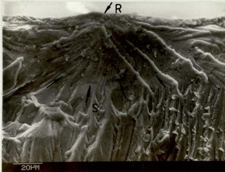
Plate 9.13 SEM micrograph showing the initiation site in Plate 9.12 at high magnification
