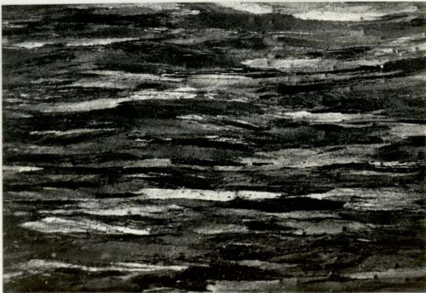
Plate 9.6 Grain structure in transverse section. Etching in Barker's reagent, X27
