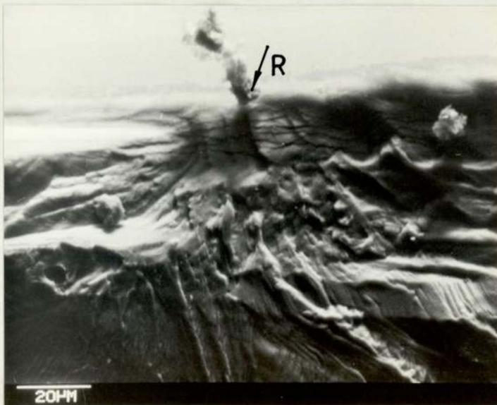
Plate 9.15 SEM micrograph showing the initiation site in Plate 9.14 at high magnification
