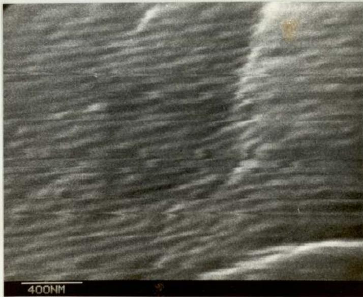
Plate 9.20 SEM fractograph taken from a site 3.80mm from the notch root
