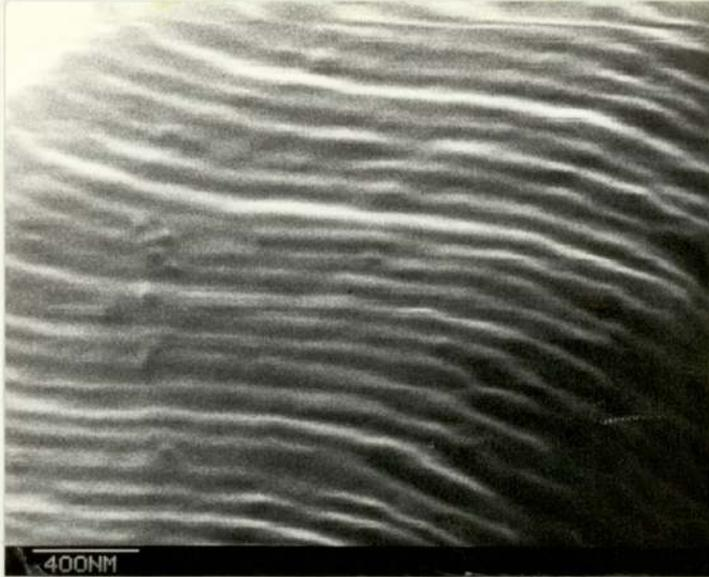
Plate 9.23 SEM fractograph taken from a site 4.39mm from the notch root.
