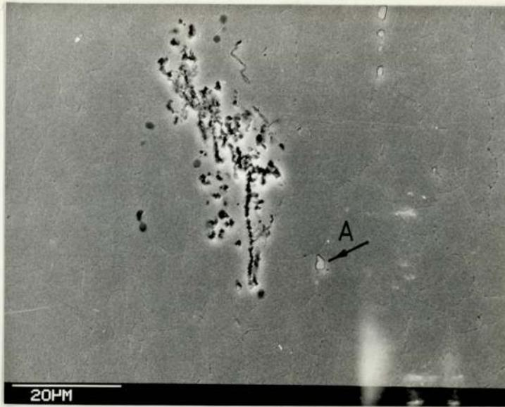
Plate 10.2 Microstructure of alloy 7010 - T736
