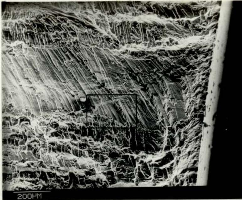
Plate 9.51 SEM fractograph showing the effect of 20% multiple overloads on crack growth in near surface region in alloy 7010 - T736.
