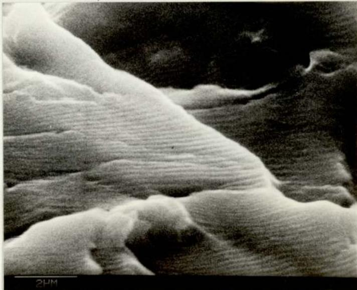
Plate 9.33 SEM fractograph taken from a site 4.72mm from the notch root
