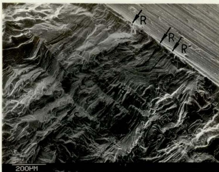
Plate 9.8 SEM micrograph showing multiple crack initiation sites ( $a_0 = 5.00\text{mm}$ ,  $\rho = 0.11\text{mm}$ )
