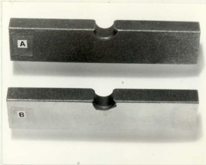
Plate 8.5 The shot-peened specimens.
