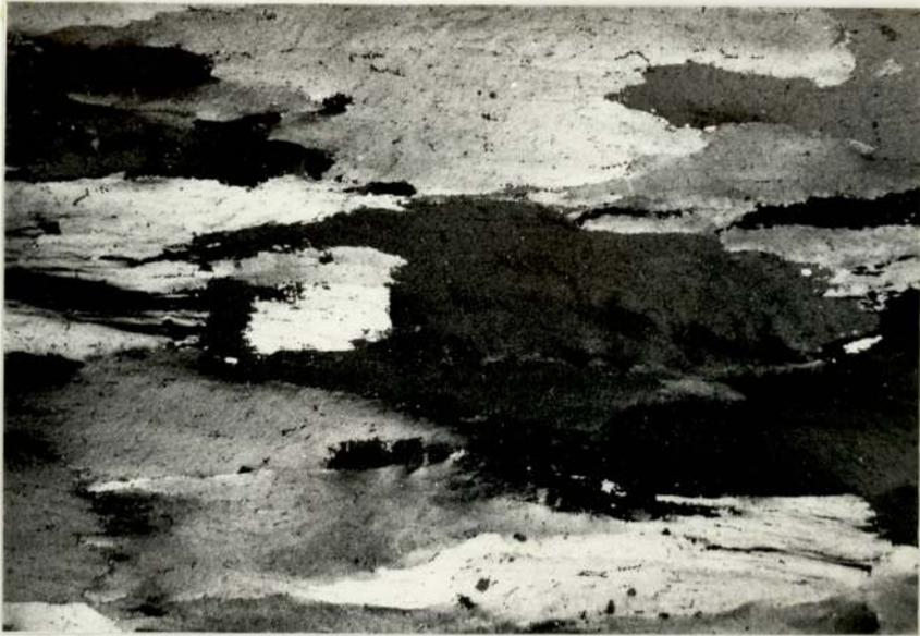
Plate 9.5 Grain structure in normal cross section. Etching in Barker's reagent, X27
