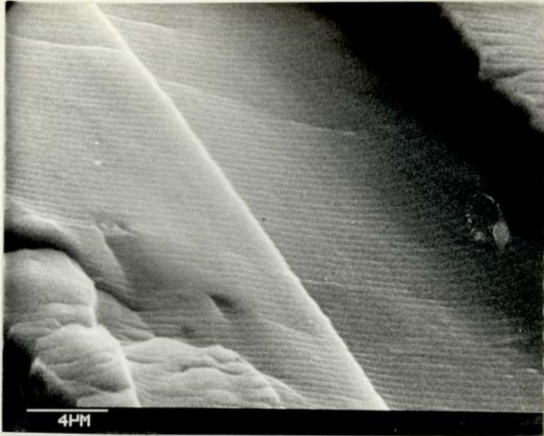
Plate 9.58 SEM fractograph taken from the site 0.1mm after the overloads, which is marked with the letter f in Plate 9.52
