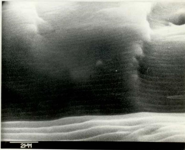
Plate 9.59 SEM fractograph taken from the interior of the specimen before overloads. The site is marked with the letter g in Fig.9.31.
