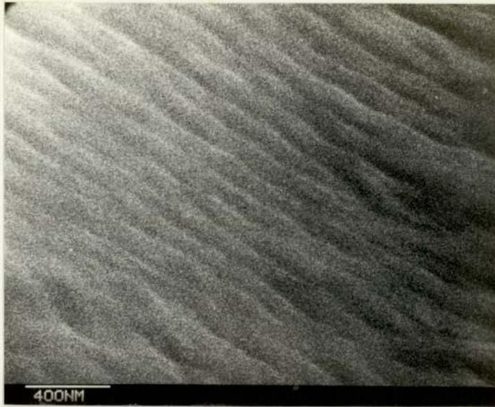
Plate 9.30 SEM fractograph taken from a site 3.96mm from the notch root.
