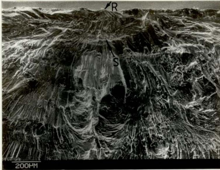
Plate 9.12 SEM micrograph showing crack initiation site in blunt notch specimen
