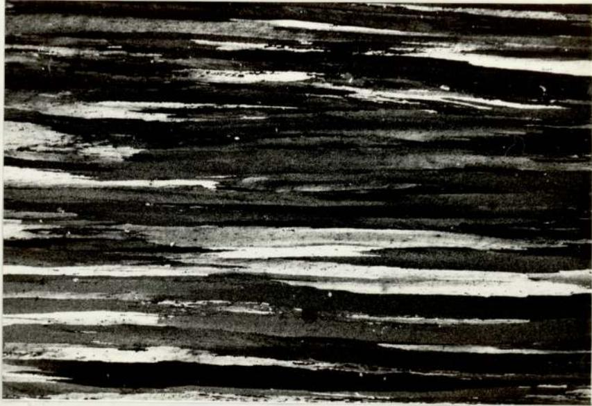
Plate 9.7 Grain structure in longitudinal section. Etching in Barker's reagent, X27
