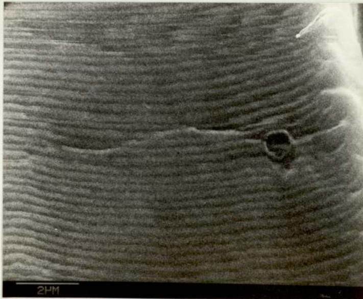
Plate 9.31 SEM fractograph taken from a site 4.34mm from the notch root, 55° correction.
