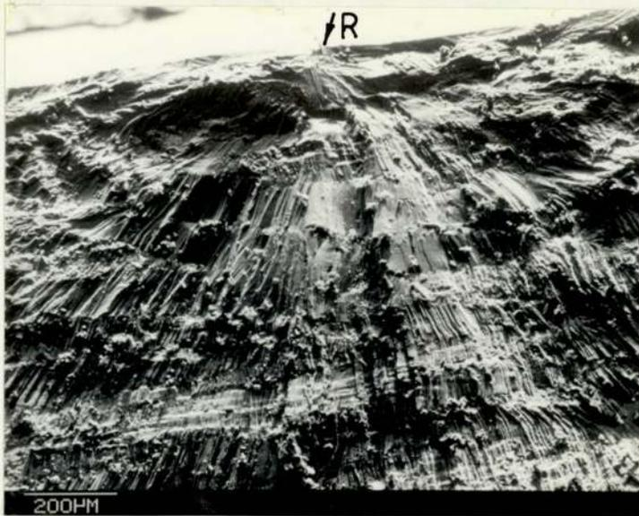
Plate 9.14 SEM micrograph showing crack initiation site in blunt notch specimen
