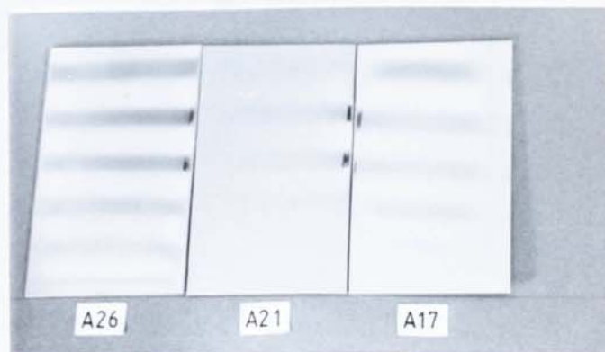
Fig.8.4: 30 minutes sputter etched specimens at 30 mTorr pressure.
