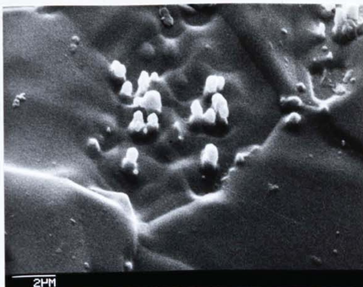
Fig.8.6: Pillar type segregates on sputter etched surface of specimen A16.
