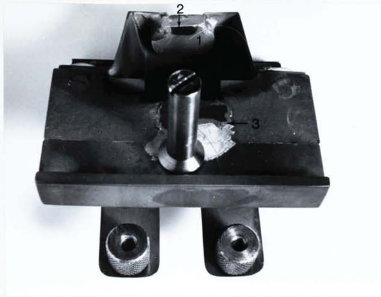
Fig.7.10: The electron beam gun assembly 1. The tungsten block, 2. place of impingement of the electron beam, 3. Remaining of the molybdenum sheet.
