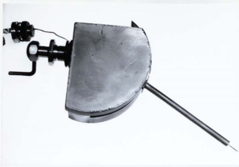
Fig.A8: The operational position. The thermocouple is out of the holder tube.
