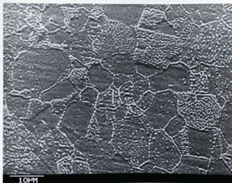
Fig.8.7: Sputter etched surface of specimen A22. Average depth of erosion: 0.44 \mu\text{m}
