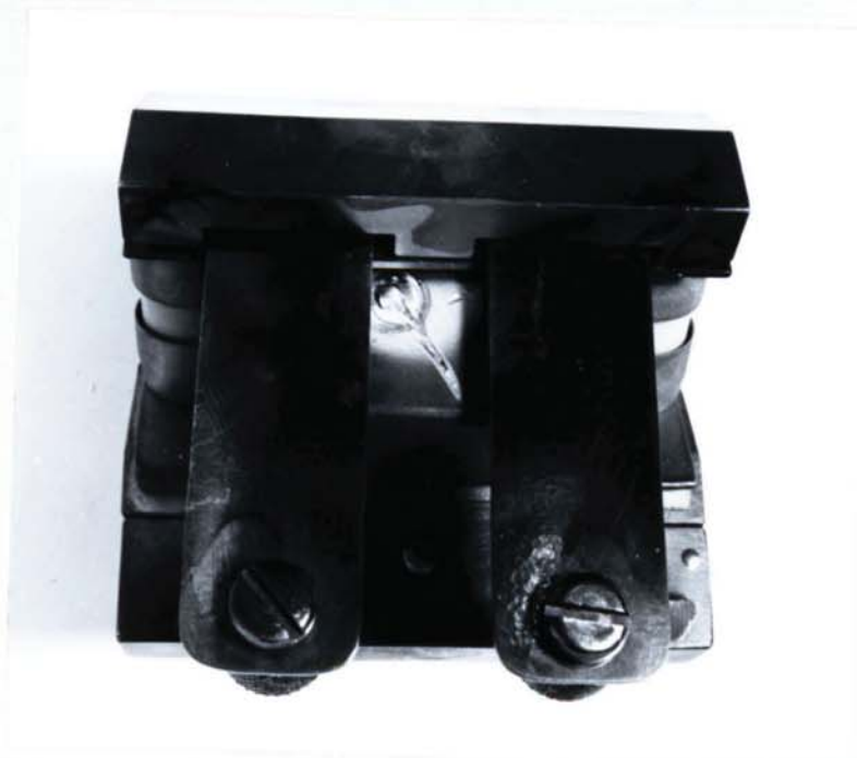
Fig.7.11: Signs of arcing underneath the anode bowl. Operation voltage 10 KV.
