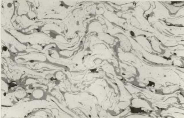
b; TYPICAL SPRAYED COATING
