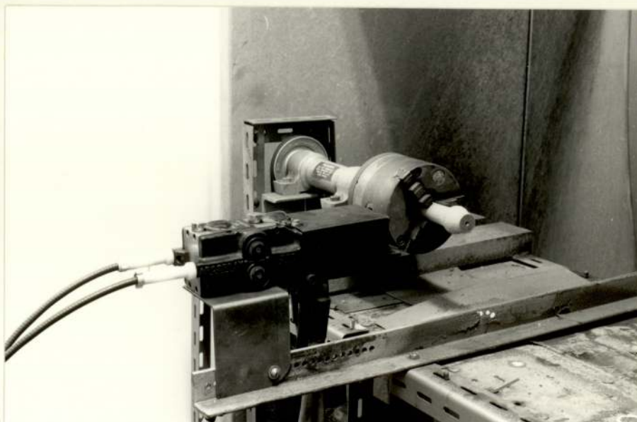
FIGURE 23 : Arc Spray Gun in Position to Spray Shear Test-Pieces
