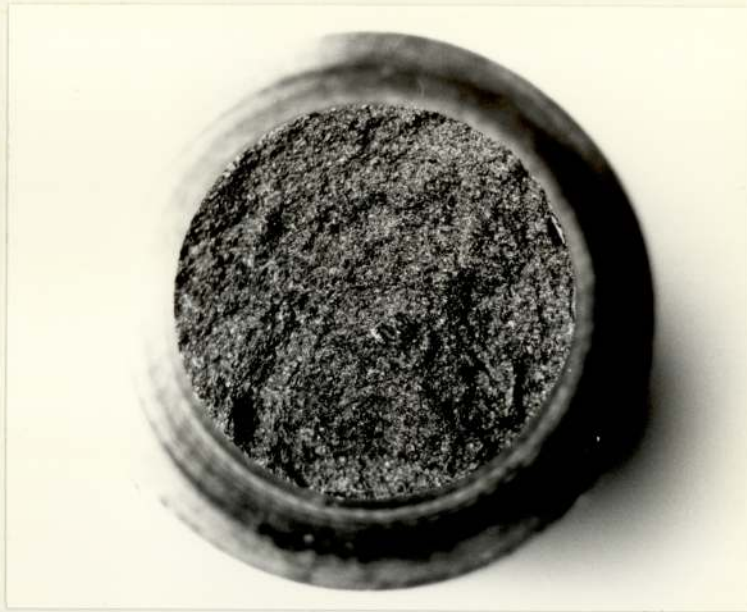
FIGURE 78 : Fracture Face : Tensile Specimen
