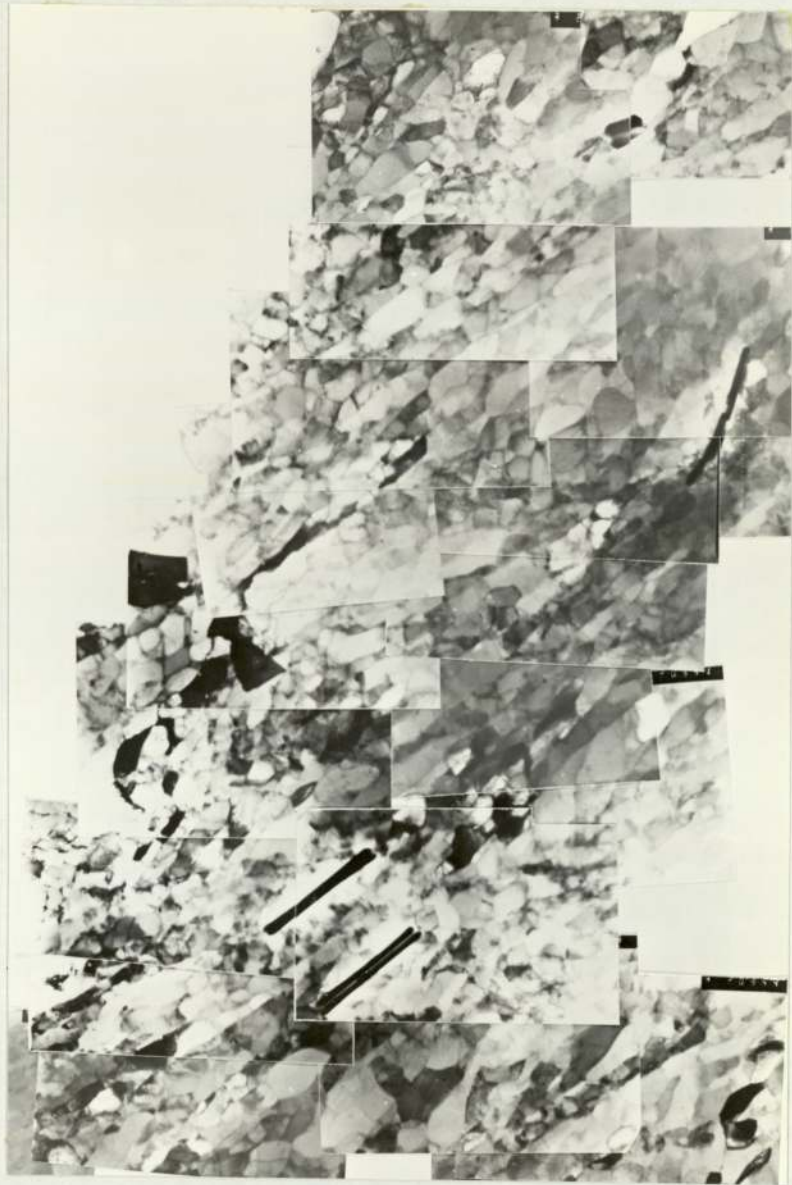
Figure 41 (b) Montage of Al-Mg-Si single crystal B cold rolled 71% (Longitudinal Section) showing the deformation microstructure
