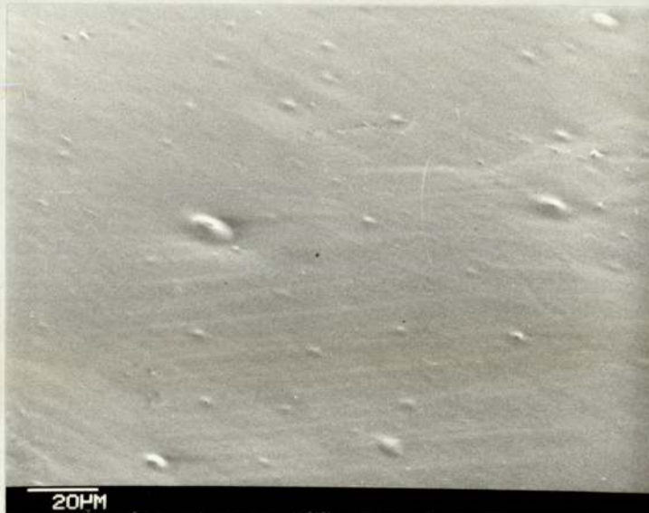
Fig. 3.44 S.P.Al electropolished for 90 secs at 10 \text{ A/dm}^2 , showing a few gassing defects. T.a. 70^\circ
