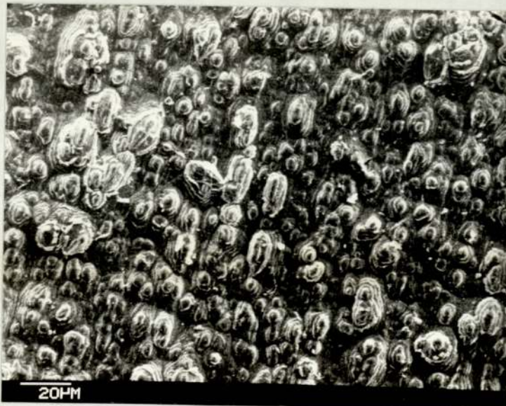
Fig. 3.14(i) C.P.Al "As rolled", after 8 minutes anodizing at 33 A/dm 2 . Shows how at high glancing angles the hillock shaped features resemble "rosettes". T.a. 10°.
