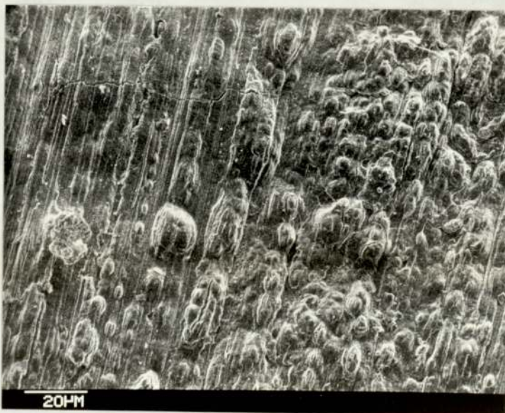
Fig. 3.15 Alloy I, P180 abraded, after 15 minutes anodizing in 5% H_2SO_4 at 22.1 A/dm^2 . T.a. 45^{\circ}
