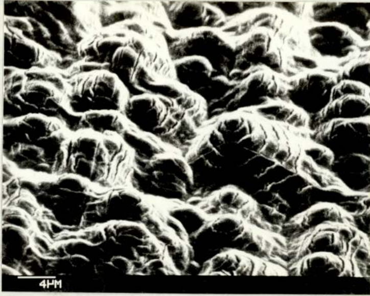
Fig. 3.5(ii) As Fig. 3.5(i), showing greater detail of the concentric ring cracks formed due to growth of the alumina. T.a.70 o
