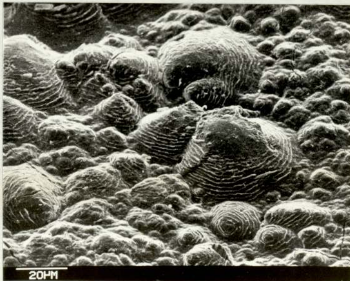
Fig. 3.30(i) As Fig. 3.25, after 57 minutes anodizing at 11 \text{ A/dm}^2 . T.a. 45^\circ
