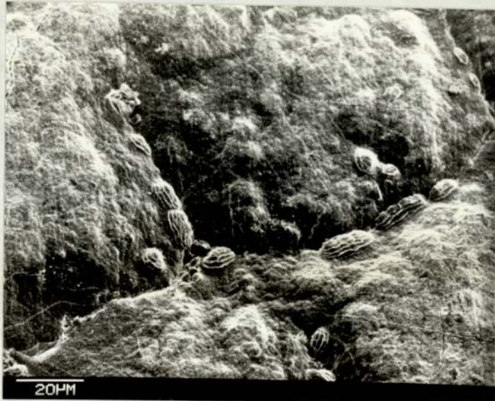
Fig. 3.19(ii) As Fig. 3.19(i), showing oxide growth at grain boundaries. T.a. 45°
