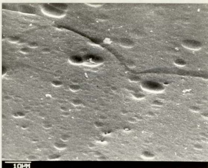
Fig. 3.93(i) C.P.Al etched in 10% NaOH, anodized for 2 minutes at 15.4 A/dm 2 in 27.6% H 2 SO 4 at 0°C. T.a. 45°
