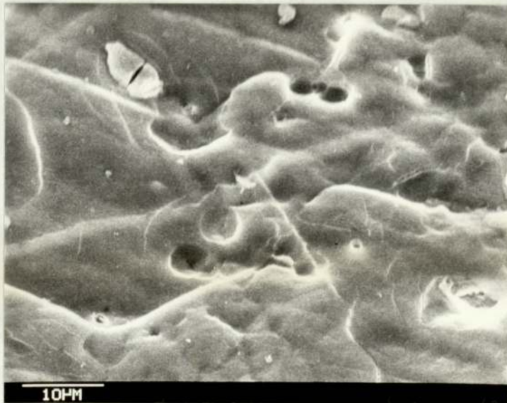
Fig. 3.36 Alloy 609 (etched), after 14½ minutes anodizing at 10.4 A/dm 2 . T.a. 45°
