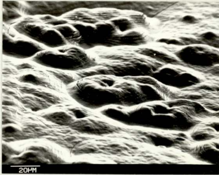
Fig. 3.45 As Fig. 3.44, after anodizing for 37 minutes at 10 \text{ A/dm}^2 . Showing the replication of the gassing defects and the characteristic nodular oxide growth. T.a. 70^\circ
