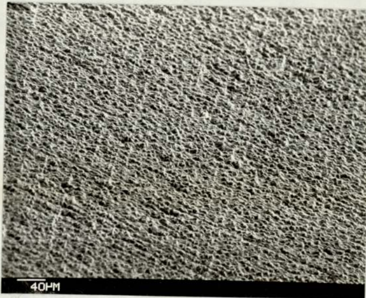
Fig. 3.21(i) H30 alloy, 1 μm polish, after 2 minutes anodizing at 33 A/dm 2 . T.a. 70°
