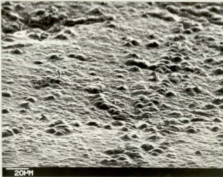
Fig. 3.51 Alloy I, heat treated and water quenched and mechanically polished to 1\mu\text{m} , after 12 minutes anodizing at 22\text{ A/dm}^2 . T.a. 70^\circ
