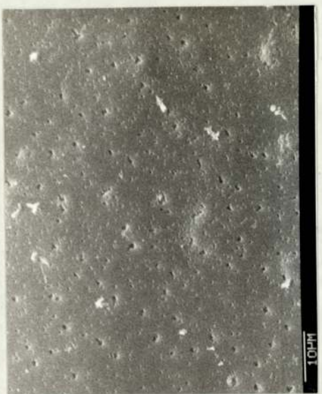
Fig. 3.89(iii) 60 minutes anodizing at 5.8 A/dm 2
