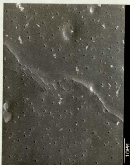
Fig. 3.87(vi) 30 minutes anodizing at 10.7 A/dm 2
