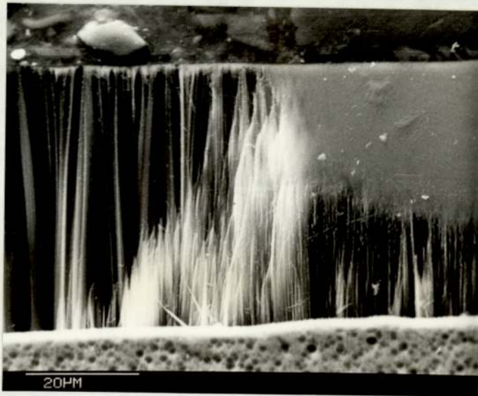
Fig. 3.82(i) Cross-sectional view of C.P. Al, chemically polished and anodized for 13 minutes at 18.9 \text{ A/dm}^2 , after chemical dissolution of oxide. T.a. 10^{\circ}
