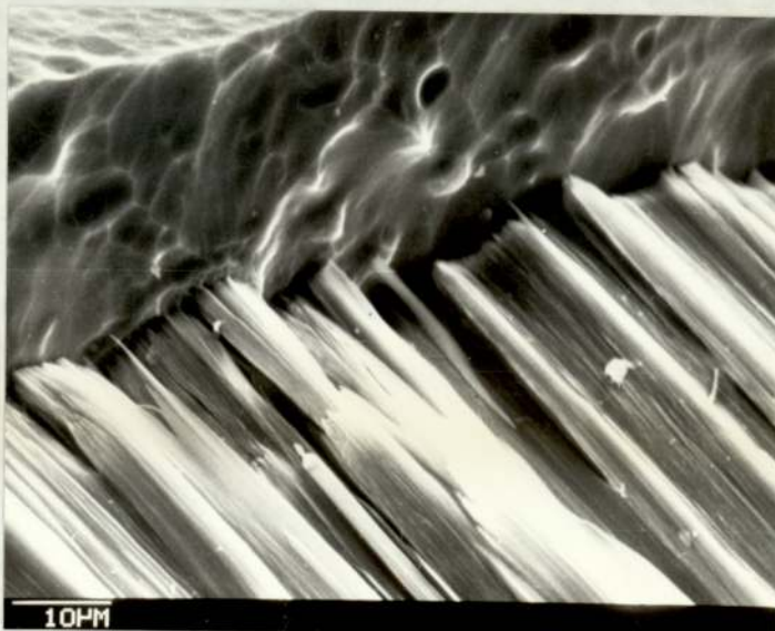
Fig. 3.84 Same pretreatment as 3.81(i) but anodized for 36 minutes at 10.5 \text{ A/dm}^2 , after chemical dissolution of oxide. T.a. 60^{\circ}
