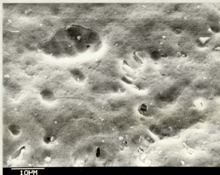
Fig. 3.32 Alloy 5182 (etched), after 17½ minutes anodizing at 9 A/dm 2 . T.a. 45°
