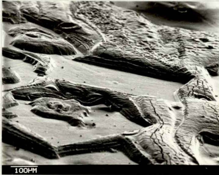
Fig. 3.43(ii) As Fig. 3.43(i), showing greater detail of the depressions at the sites of prior icing defects. T.a. 70^\circ
