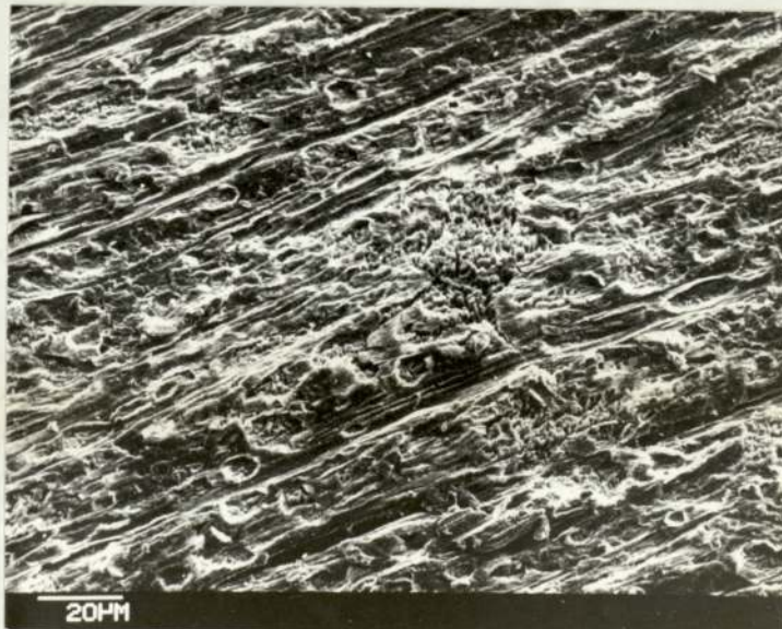
Fig. 3.18 Alloy II, P180 abraded, after 23 minutes anodizing in 5% H_2SO_4 at 22.1 A/dm^2 . No agitation, shows "burning". T.a. 45^\circ
