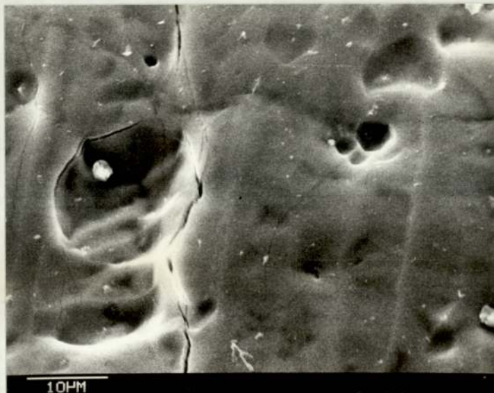
Fig. 3.34 Alloy 2117HP (etched), after 18½ minutes anodizing at 9 A/dm 2 . T.a. 45°
