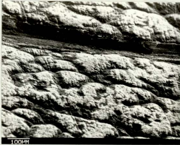
Fig. 3.23 Alloy II, 1 \mu m polish, scored, after 7½ minutes anodizing at 11 A/dm 2 . T.a. 70°
