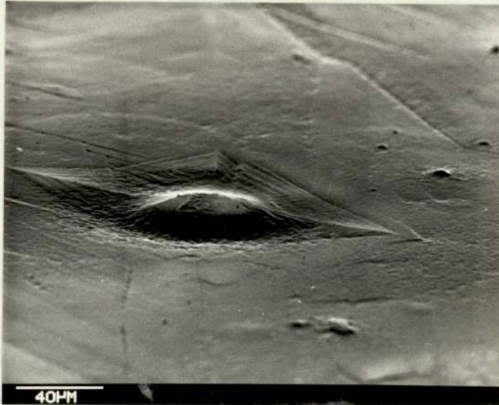
Fig. 3.42 Icing defect around a gassing defect after 120 seconds electropolishing. T.a.80°
