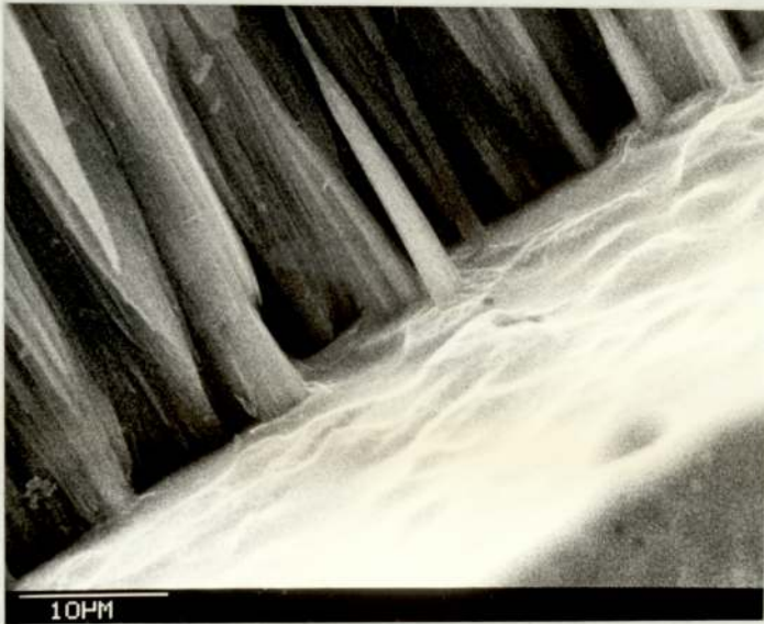
Fig. 3.81(i) Cross-sectional view of C.P. Al, chemically polished and anodized for 4\frac{1}{2} minutes at 41.6 \text{ A/dm}^2 , after chemical dissolution of oxide. T.a. 10^\circ
