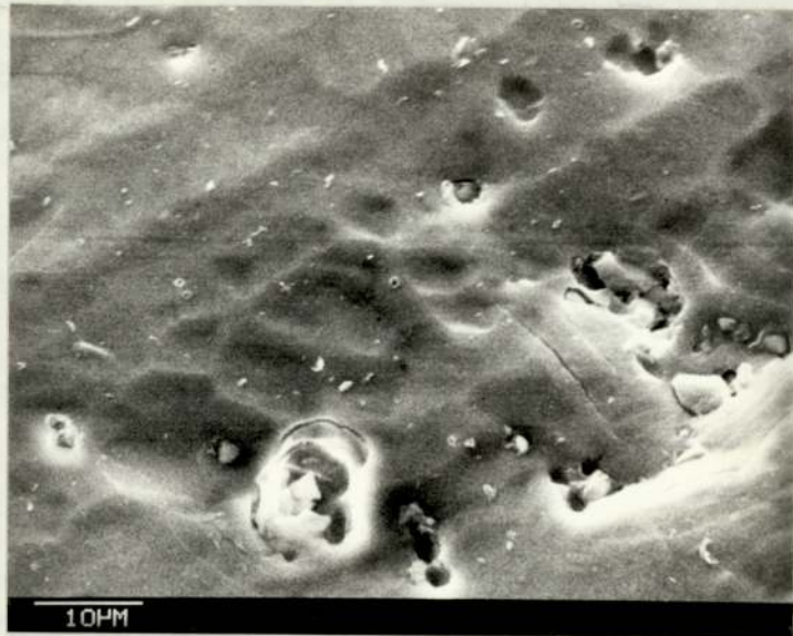
Fig. 3.33 Alloy 2117CP (etched), after 15 minutes anodizing at 10.4 A/dm 2 . T.a. 45°
