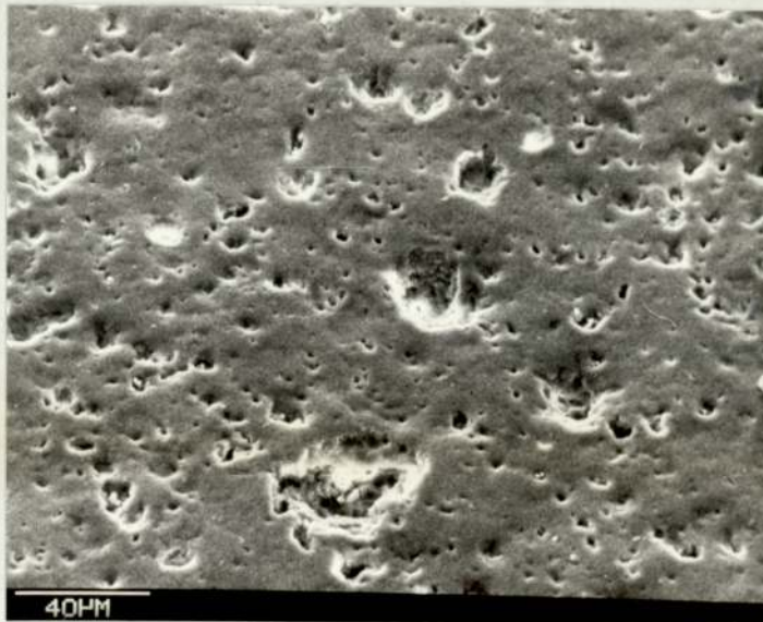
Fig. 3.78(i) Underside of oxide electrolytically detached from alloy 2117CP. T.a. 45^{\circ}
