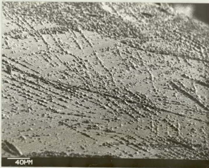
Fig. 3.6(i) S.P.Al "As rolled", after 1 sec anodizing at 39.7 A/dm 2 . T.a.70 o
