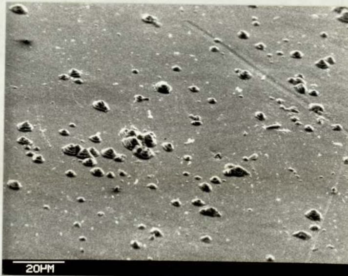
Fig. 3.9(i) C.P. Al. "As rolled", after 5 secs anodizing at 6.6 \text{ A/dm}^2 . T.a. 70^\circ
