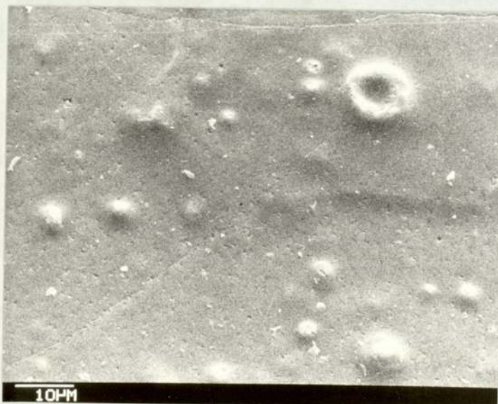
Fig. 3.92(ii) As Fig. 3.92(i), with anodic oxide chemically stripped off. T.a. 45°
