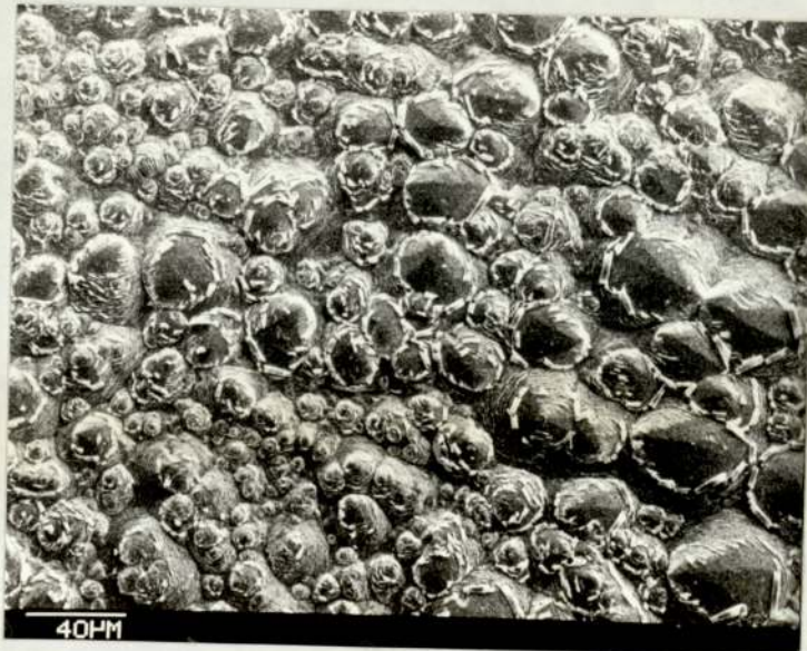
Fig. 3.28(i) As Fig. 3.25, after 120 secs anodizing at 35.7 \text{ A/dm}^2 . Shows spalling and curling of outer layer of oxide. T.a. 10^\circ .
