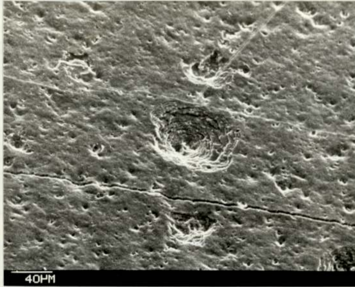
Fig. 3.77(i) Underside of oxide electrolytically detached from alloy BB3. T.a. 45^{\circ}
