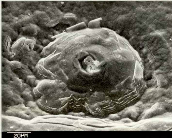
Fig. 3.38 As Fig. 3.37, after 4\frac{1}{2} minutes anodizing at 41.6 \text{ A/dm}^2 . T.a. 45^\circ
