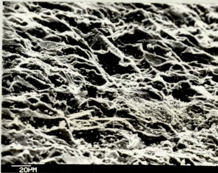
Fig. 3.12 S.P.Al surface after being sand blasted. T.a. 70^{\circ}
