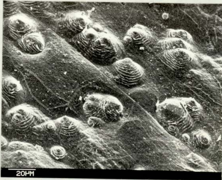
Fig. 3.19(i) Alloy II, 1 μm polish, after 14 minutes anodizing in 5% H 2 SO 4 at 22.1 A/dm 2 . T.a. 45°
