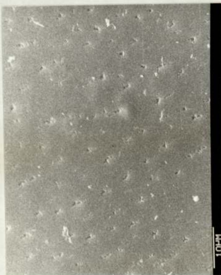
Fig. 3.89(i) 15 Minutes anodizing at 5.8 A/dm 2
