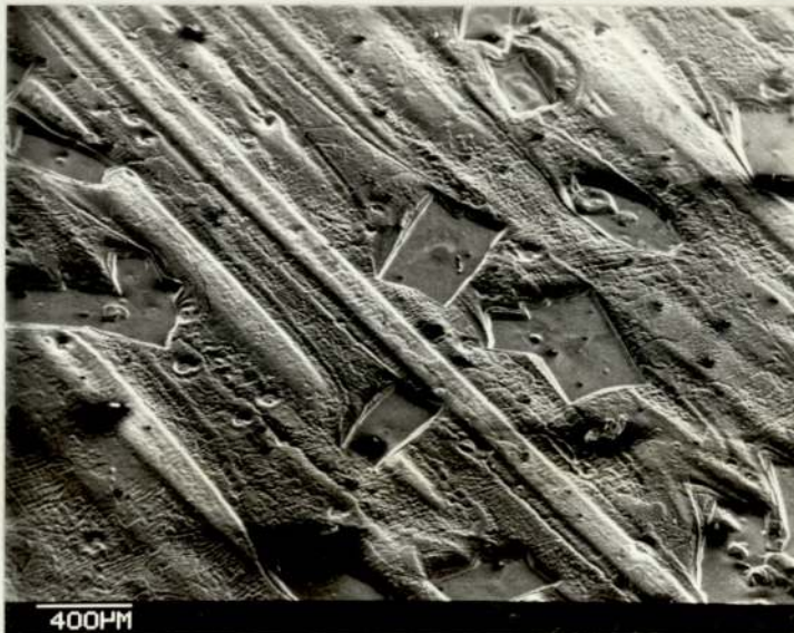
Fig. 3.43(i) Surface topography after electropolishing and then hard anodized. Shows depressions at sites of prior icing defects. T.a.45°
