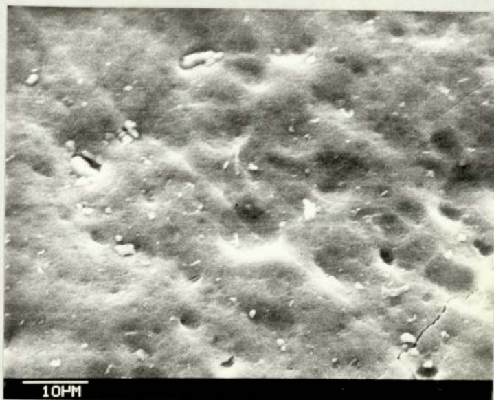
Fig. 3.31 Alloy BB3 etched in 10% NaOH at 60°C for 2 minutes, after 17 minutes anodizing at 10.4 A/dm 2 . T.a. 45°
