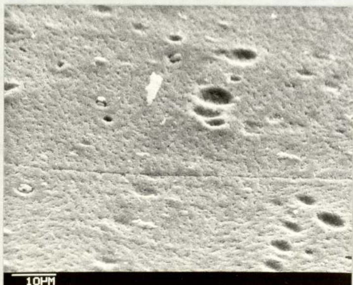
Fig. 3.93(ii) As Fig. 3.93(i), with anodic oxide chemically stripped off. T.a. 45°
