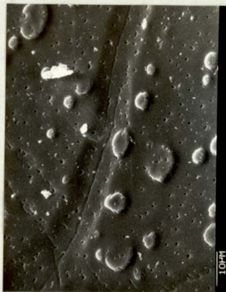
Fig. 3.87(xi) 15 minutes anodizing at 19.2 A/dm 2
