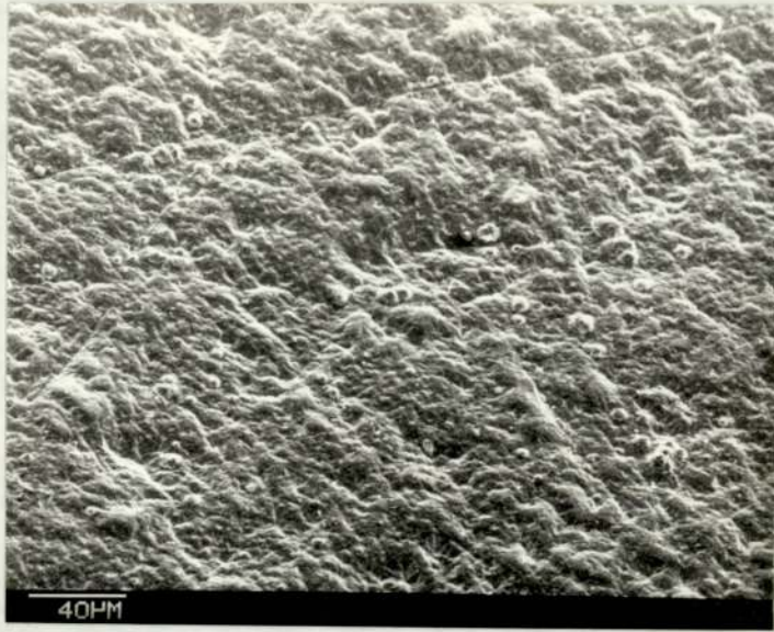
Fig. 3.49 C.P. Al, heat treated and water quenched, after 17 minutes anodizing at 6.9 \text{ A/dm}^2 . T.a. 45^\circ
