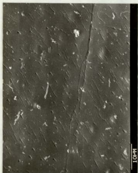
Fig. 3.87(ii) 30 minutes anodizing at 5.8 A/dm 2
