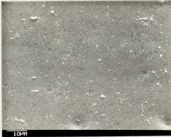
Fig. 3.37 S.P. Al chemically polished in 78% \text{H}_3\text{PO}_4 - 16% \text{H}_2\text{SO}_4 - 6% \text{HNO}_3 - 0.5% \text{CuSO}_4 at 98^\circ\text{C} for 90 secs. T.a. 45^\circ
