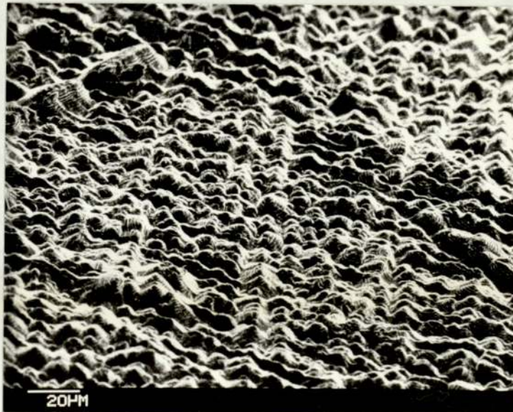
Fig. 3.5(i) S.P. Al. "As rolled", after 300 secs anodizing at 23.8 \text{ A/dm}^2 . T.a. 70^\circ
