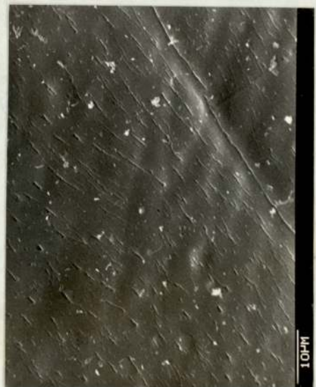
Fig. 3.87(i) 15 minutes anodizing at 5.8 A/dm 2
