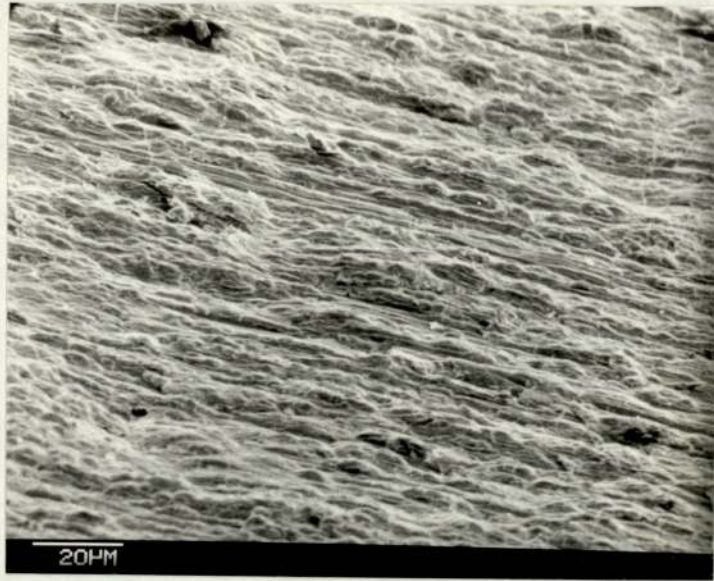
Fig. 3.17 Alloy II, P180 abraded, after 18 minutes anodizing in 5% H_2SO_4 at 22.1 A/dm^2 . T.a. 70^\circ
