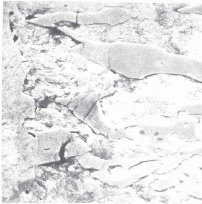
(a) Sub-surface cracking of eutectic carbides.
