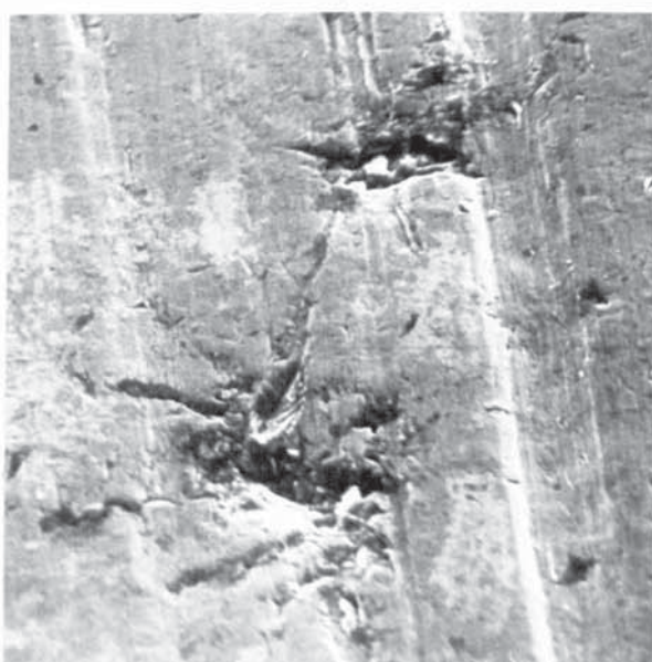
(c) Iron 5 (3%C-20%Cr) Hv=858, wear index=1.27
