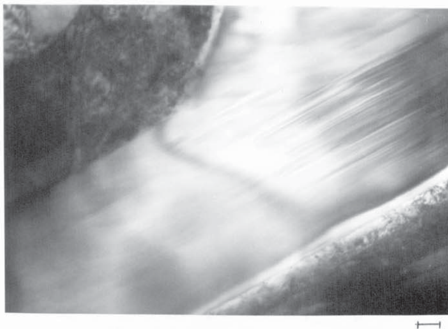
(a) Contrast due to faulting in eutectic M_7C_3 Marker is 0.1 \mu m .
