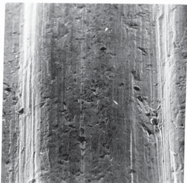
(a) As cast, pearlite matrix Hv=564, wear index=0.95
