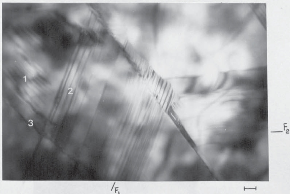
(a) Wavy faults (1) producing steps in straight fault (2). Two lines of intense contrast (3) crossing into faulted region.
