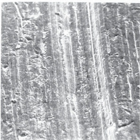
(a) 3%C-20%Cr iron Pearlite+austenite matrix Hv=590, wear index=1.10
