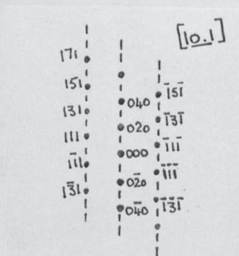
(b) Diffraction pattern from central M_7C_3 carbide.
